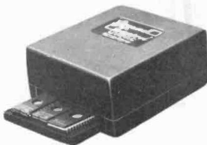
measures 90mm x 80mm x 40mm. A fibre optic indicator is used to show that the unit is in operation. EPROMs are simply loaded onto the conductive foam supplied and inserted into the unit. The 'Uvipac' costs £21.45 as a standard unit or £24.95 with a built-in (15 min) timer. From Ground Control, Alfreda Avenue, Hullbridge, Essex SS5 6LT (0702 230324).
