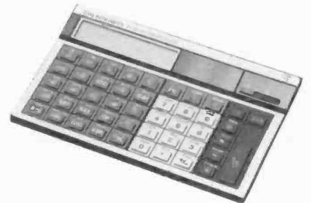
58C/59 family of calculators. The constant memory feature retains data and program information even when the calculator is turned off.
