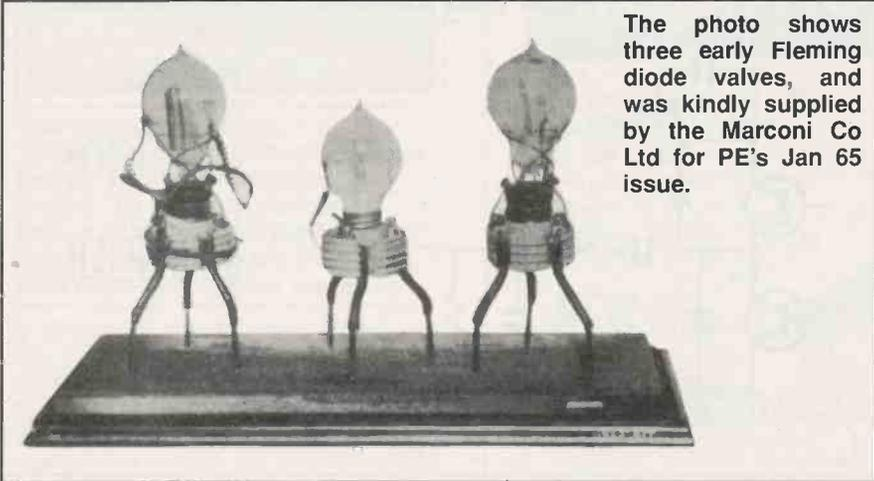
**The photo shows three early Fleming diode valves, and was kindly supplied by the Marconi Co Ltd for PE's Jan 65 issue.**
