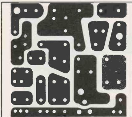
Even in issue one, PE showed pcb track layouts, though they bore striking resemblance to Meccano plates! This board was for a drive amplifier
