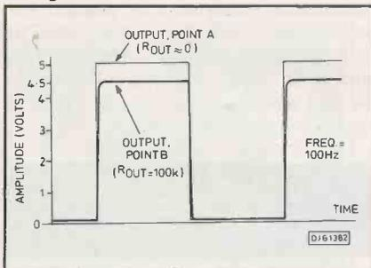
Fig 2. Multivibrator outputs.
