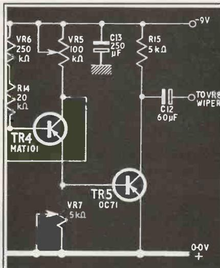
Circuit for part of the Didjeridoo project in PE Nov 64. The transistors are pnp germanium types, npn and silicon devices were not yet readily available to readers. The 'inverted' power lines would have caused mental acrobatics for some! Using white lines on a black background was probably meant to imply equivalence to 'blue prints', so inspiring a feeling of 'belonging' to the engineering fraternity.
