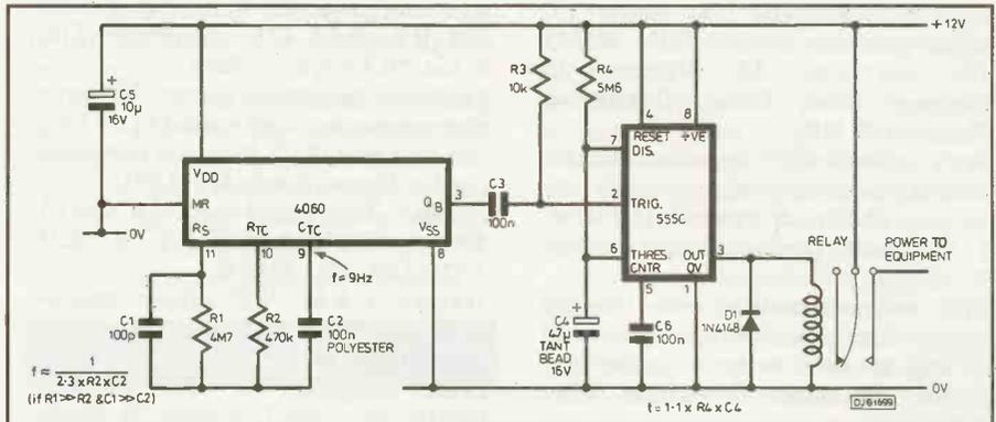
Fig 1. Suggested extended timing ratio circuit and typical waveforms.
