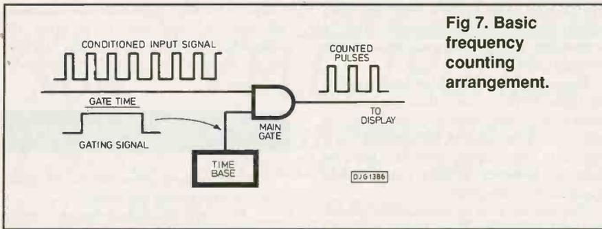
**Fig 7. Basic frequency counting arrangement.**
