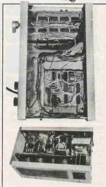
PE's first digital clock, in Dec 70, used digitron tubes for the numerical displays. These were a type of valve with glowing digits. The circuit was designed around the standard 7400 series of ttl chips. With the current all those chips and tubes consumed, the unit was probably a good source of central heating as well!
