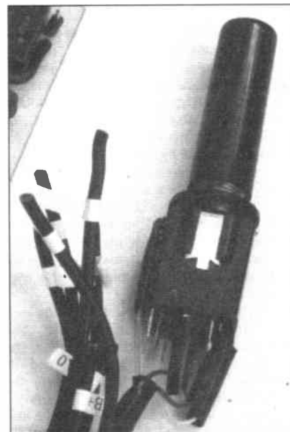
View of the jack socket connections, with jack plug inserted, and of the tabbed coding of the other wires before connection.
