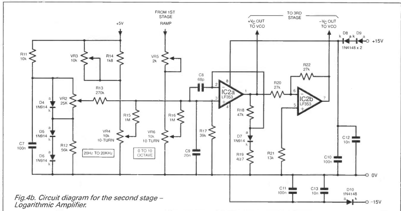
Fig.4b. Circuit diagram for the second stage - Logarithmic Amplifier.
