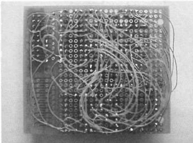
Underside wiring for the 8-bit interrupt latch.
