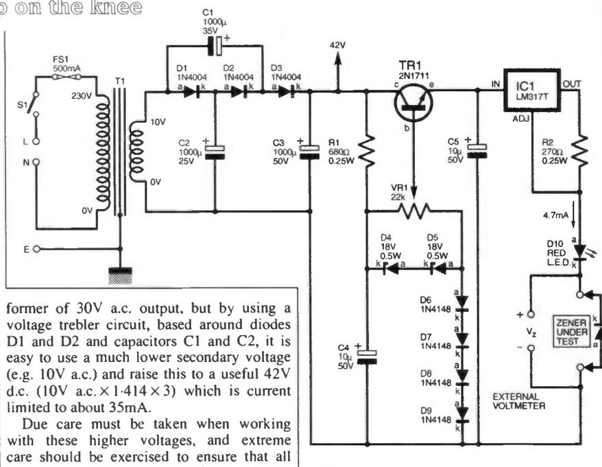
former of 30V a.c. output, but by using a voltage trebler circuit, based around diodes D1 and D2 and capacitors C1 and C2, it is easy to use a much lower secondary voltage (e.g. 10V a.c.) and raise this to a useful 42V d.c. (10V a.c.  $\times$  1.414  $\times$  3) which is current limited to about 35mA.
