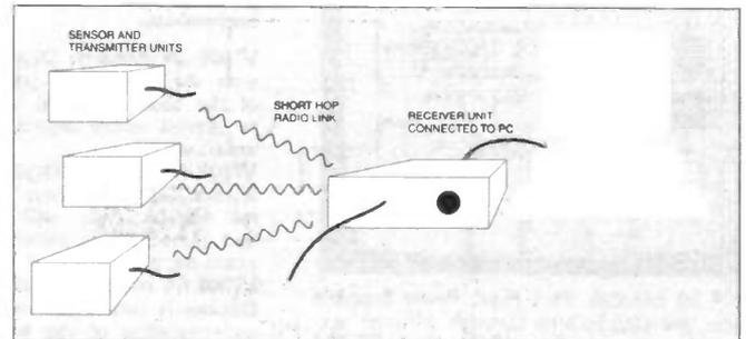
Fig.1. Block diagram of the Wireless Monitoring System.
