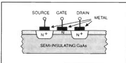
Fig. 1. Construction of a MESFET device.
