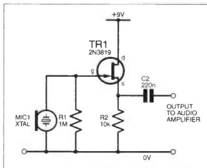
Fig. 1. Crystal amplifier circuit of the Acoustic Probe.
