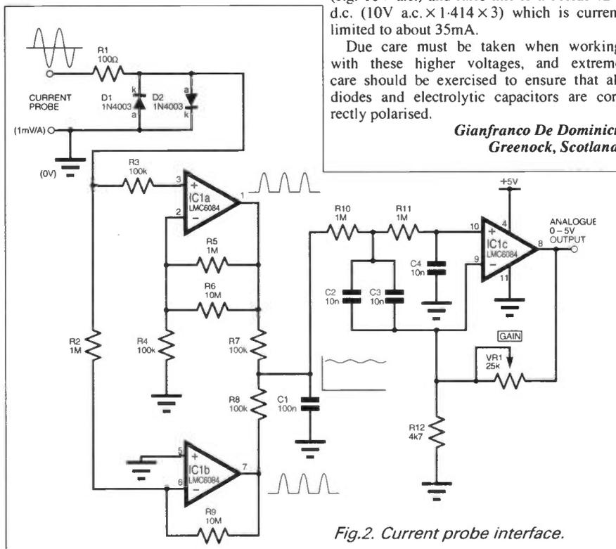
Fig.2. Current probe interface.
