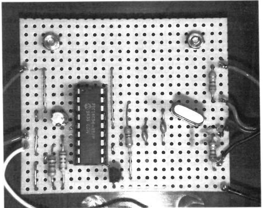
Layout of components on the completed stripboard. Make sure you include the four very small link wires.
