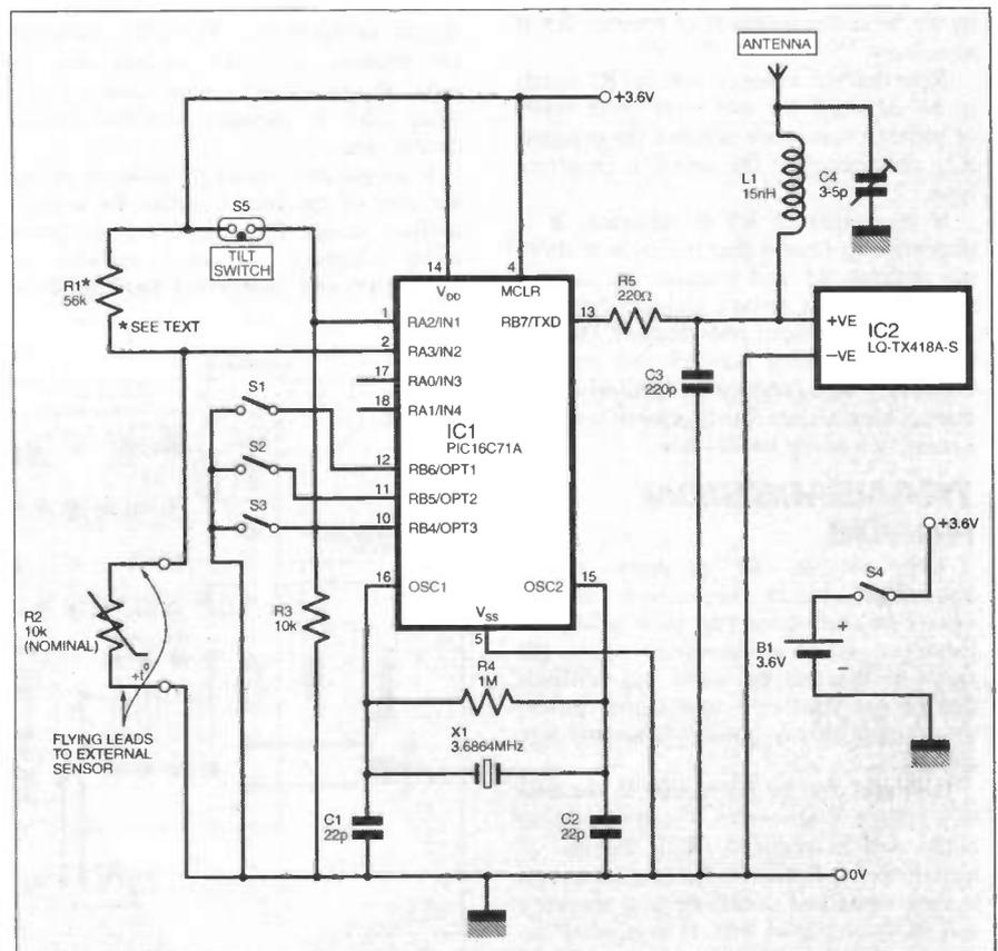
Fig. 4. Complete circuit diagram for the Transmitter. Note that switches S1 to S4 are d.i.l. slide types.
