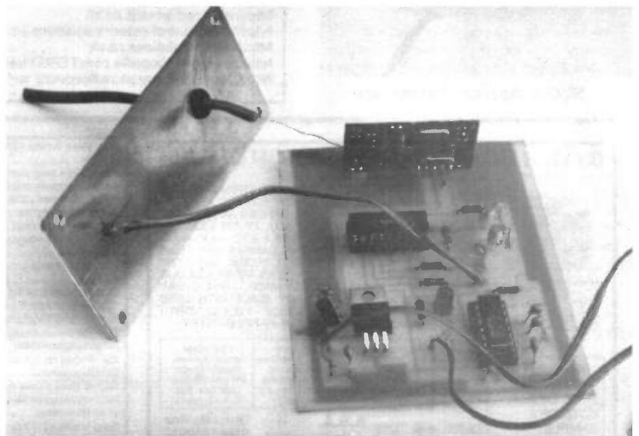
The r.f. status l.e.d. mounted and wired on the front panel. This can also be accompanied by the RS232 com status l.e.d. if preferred.
