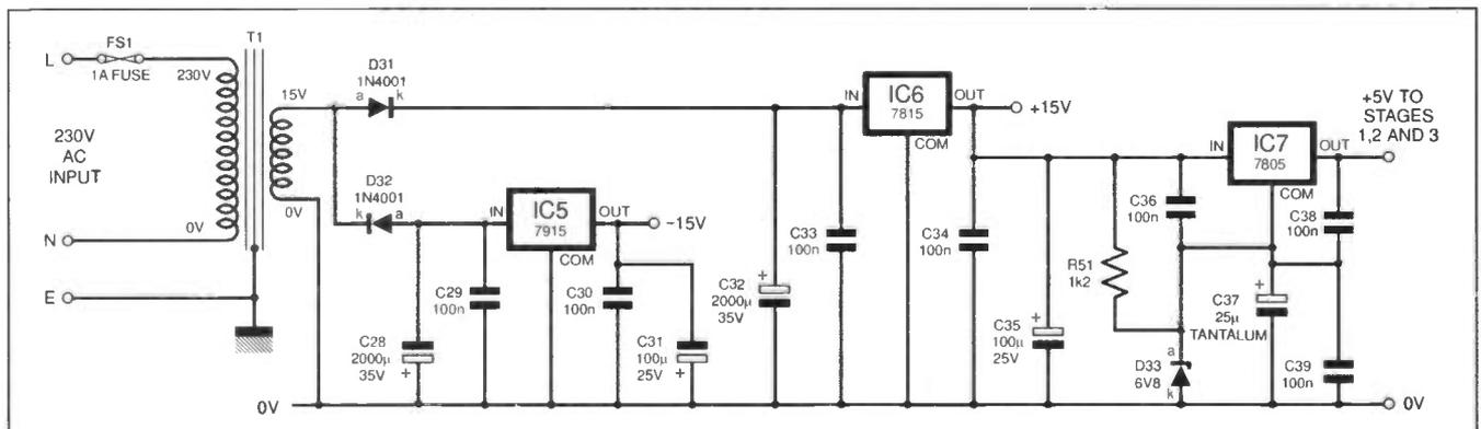
Fig.4e. Mains power supply circuit for the A.F. Sweep Signal Generator.
