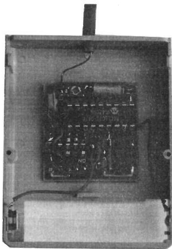
Positioning of the p.c.b. inside the Transmitter case.
