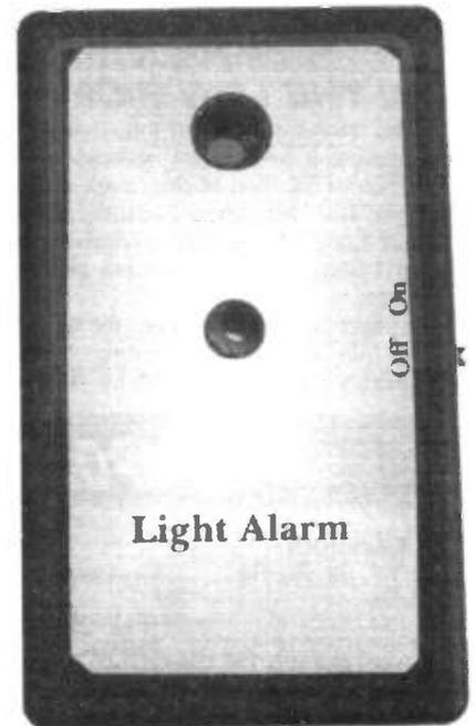
*The light "window" and sound exit holes should align with the l.d.r. and warning buzzer when the case is closed up.*
