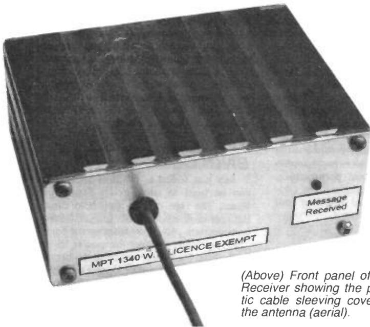
(Above) Front panel of the Receiver showing the plastic cable sleeving covering the antenna (aerial).
