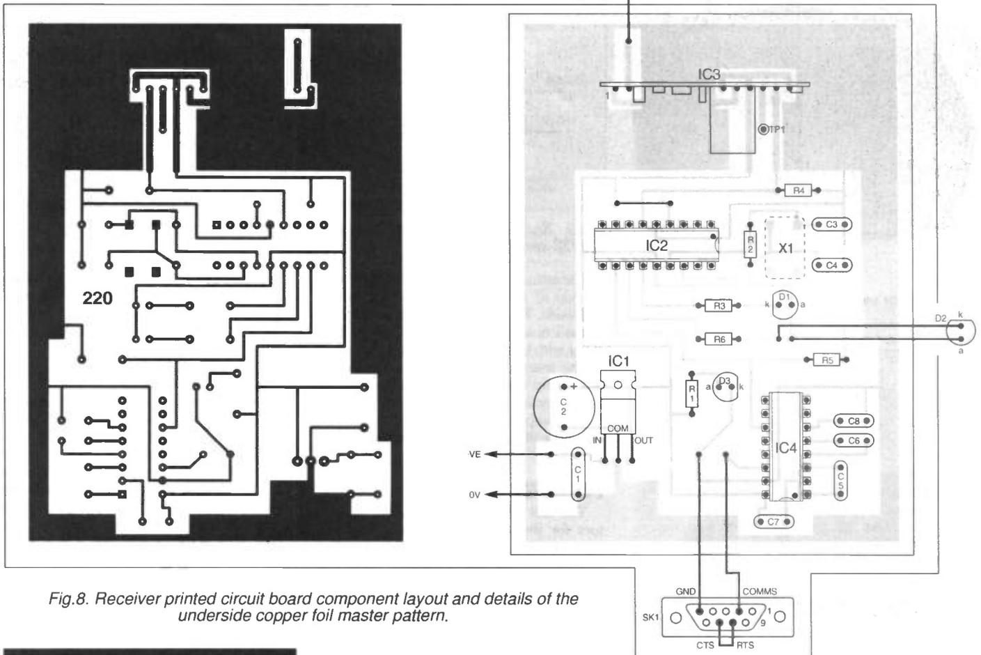
Fig.8. Receiver printed circuit board component layout and details of the underside copper foil master pattern.
