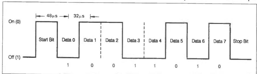
Fig. 1. Example waveform diagram for a MIDI byte.
