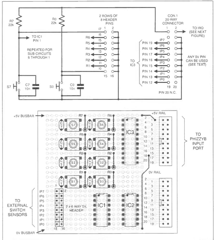
Fig.4. Switch circuit diagram and board layout for the 8-bit interrupt latch.
