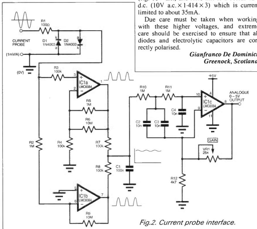
Fig.2. Current probe interface.
