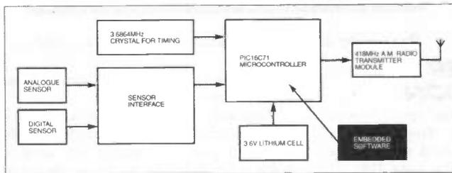
Fig. 2. Transmitter block diagram.
