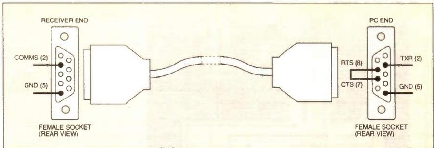
Fig.9. Serial cable interconnection details between the Receiver and the PC RS232 serial port.
