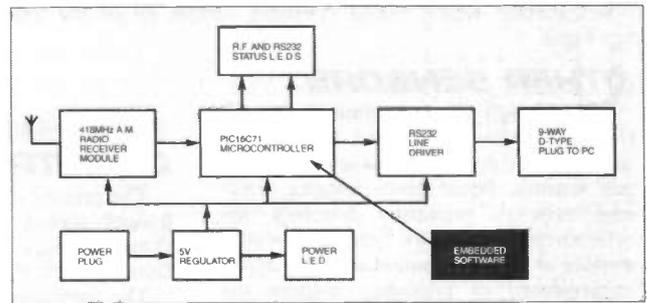
Fig. 3. Block schematic diagram for the Receiver.
