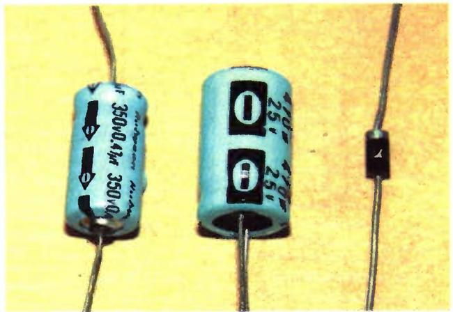
*The polarity of polarised components is clearly marked on the components themselves, and should be marked unambiguously on component layout diagrams. Note the band on the diode designating the cathode (k) end.*
