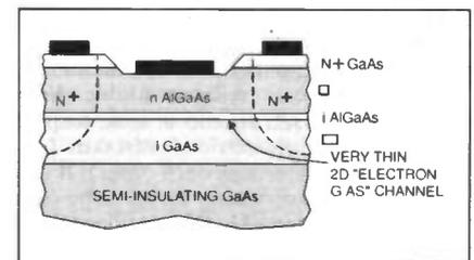
Fig. 2. Internal structure of a PHEMT.
