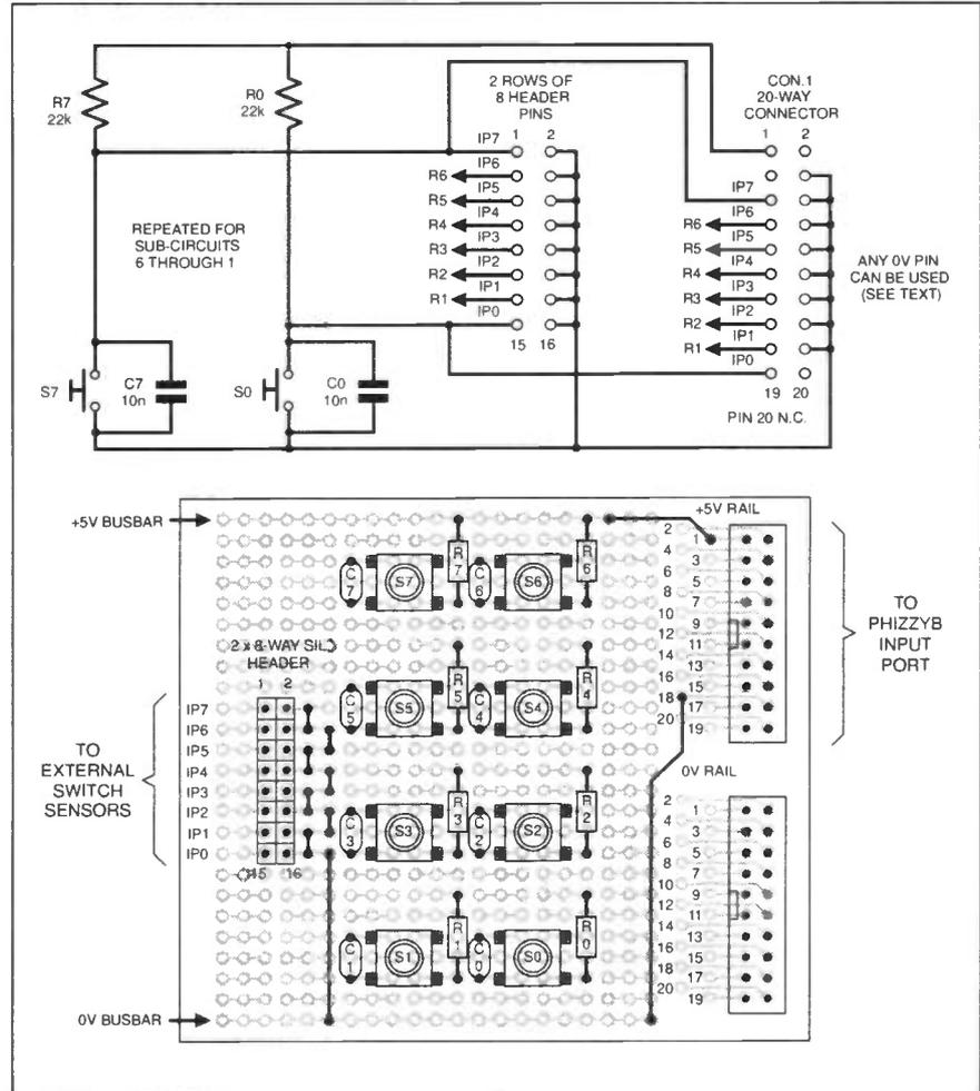
Fig.1. Circuit diagram and board layout for a simple 8-switch input “polling” module.
