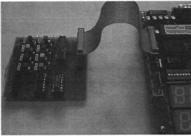
The 8-bit interrupt latch connected to PhizzyB.
