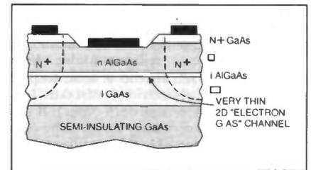
Fig. 2. Internal structure of a PHEMT.
