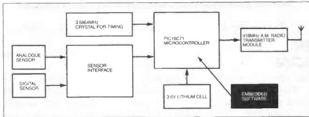
Fig. 2. Transmitter block diagram.
