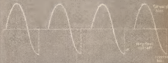
Fig. 1c. Current through a step recovery diode
