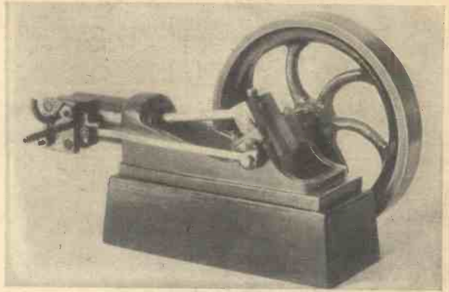
Fig. 2.—Another view of the slide-valve mechanism
