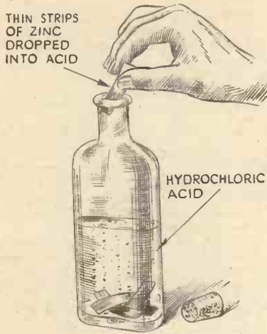
Fig. 1.—Chloride of zinc can be made by dissolving strips of zinc in hydrochloric acid. A porcelain vessel should, for preference, be used
