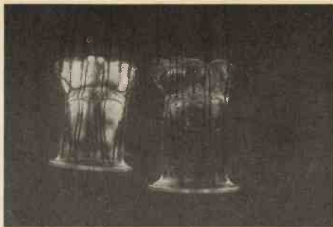
* Fig. 7.—The base of a wireless valve photographed with Pola Screens. The one on the left has not been annealed and the light patches show the existence of strains in the glass. The right-hand one has been properly annealed.
