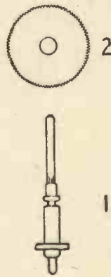
The various parts to be fitted to the minute hand spindle showing the order of assembly.
