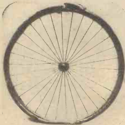
A wheel of the first pneumatic-tyred bicycle, now in a museum. The tyre was correctly constructed with the threads in tension.
