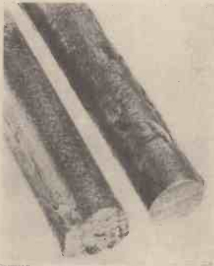
(Left) A rod of antimony. (Right) A rod of pure tin. The antimony is coarsely crystalline. It will not withstand the slightest shock without breaking. The tin, being finely crystalline, will resist considerable strain without fracture
