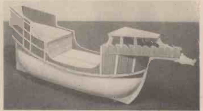
Figs. 5 and 7.—(Above) How the upper decks are mounted on the keel. (Right), The hull ready for painting
