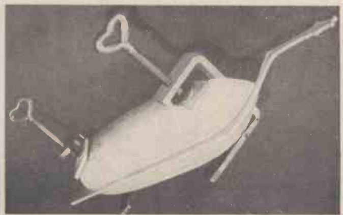
Figs. 3 and 4.—(Left), The two hull pieces B, and the keel A. (Right) The hull pieces glued to the keel
