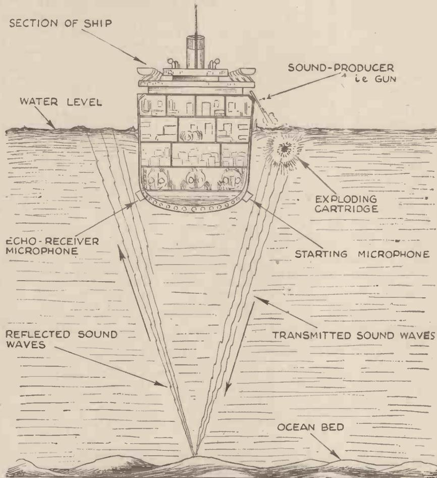
The fundamental principle of the modern "echo" system of ocean depth sounding
