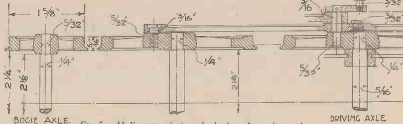
Fig. 5.—Half sectional plan of wheels and coupling rod
