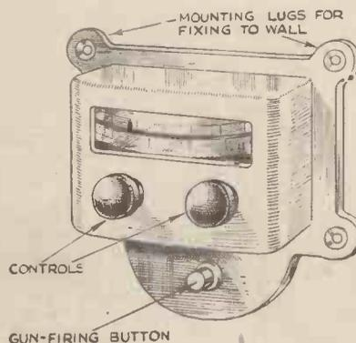
Showing the depth indicator instrument dial by means of which the sound impulse is indicated and the sea depth read off at a glance in fathoms from the calibrated dial
