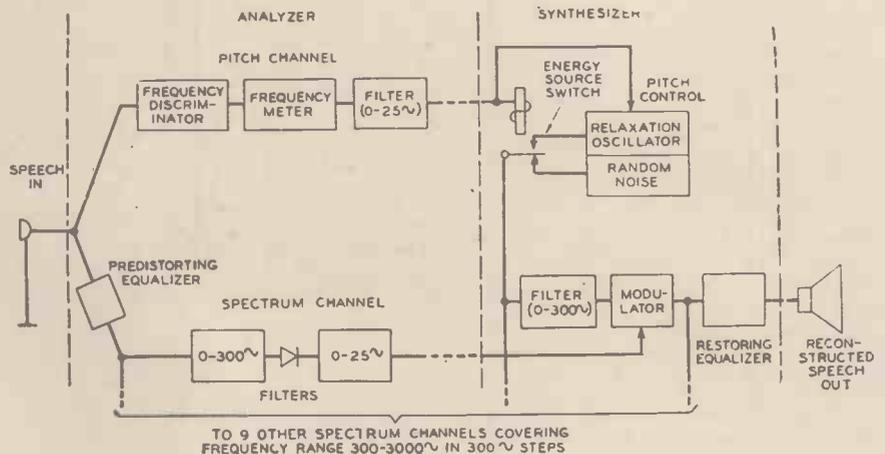
Fig. 1.—Simplified circuit diagram of the Vocoder
