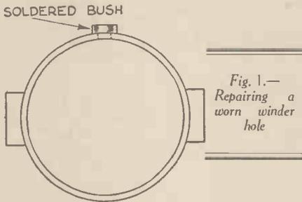
Fig. 1.—Repairing a worn winder hole
