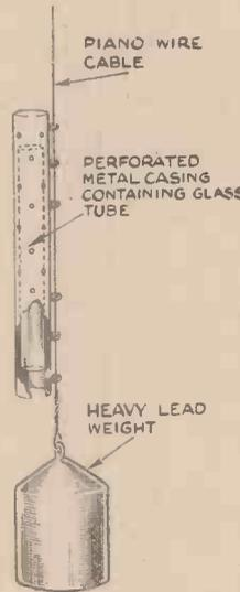
The Kelvin "sinker" for estimating ocean depth. The glass tube hangs open end downwards and is coated interiorly with silver chloride, which discolours in contact with sea water
