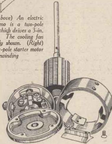
should use a stout wire here, as a machine having 1 ampere flowing through the field coils has about 10 amperes circulating through the armature, hence the necessity for a good commutator and brush gear. With most machines there is some arrange-
