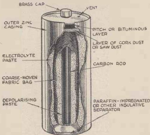
From this diagram the essentials of dry battery construction may be seen at a glance
