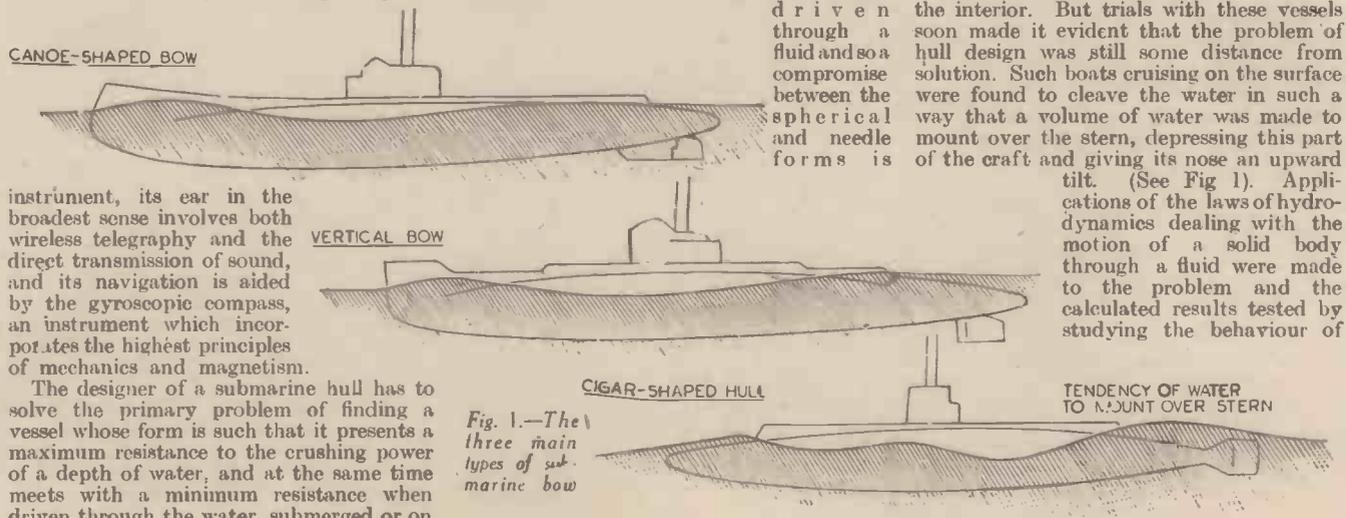
Fig. 1.—The three main types of submarine bow
