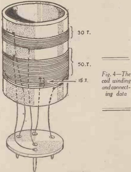
Fig. 4—The coil winding and connecting data
