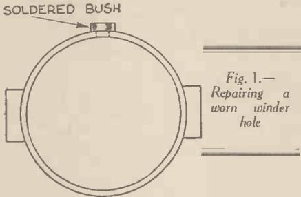
Fig. 1.—Repairing a worn winder hole
