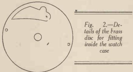
Fig. 2.—Details of the brass disc for fitting inside the watch case
