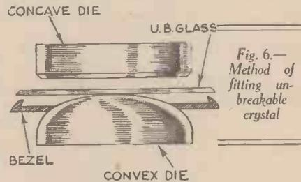
Fig. 6.—Method of fitting unbreakable crystal
