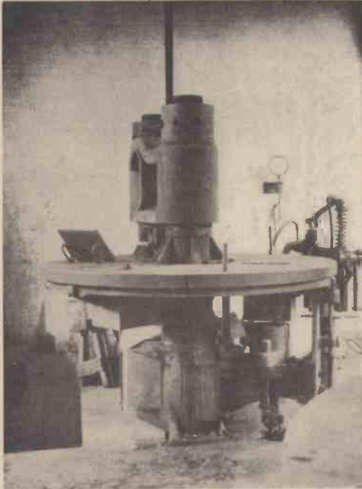
A modern hydraulic press used for the manufacture of cement tiles functions upon the principle first applied by Joseph Bramah
