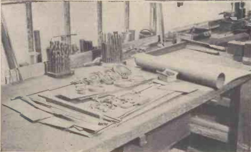
Fig. 2.—Sheet metal, tubing, and castings used in the construction of the model
