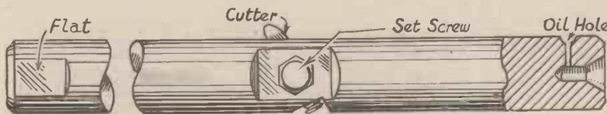
Fig. 1.—A suitable boring bar
