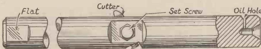
Fig. 1.—A suitable boring bar
