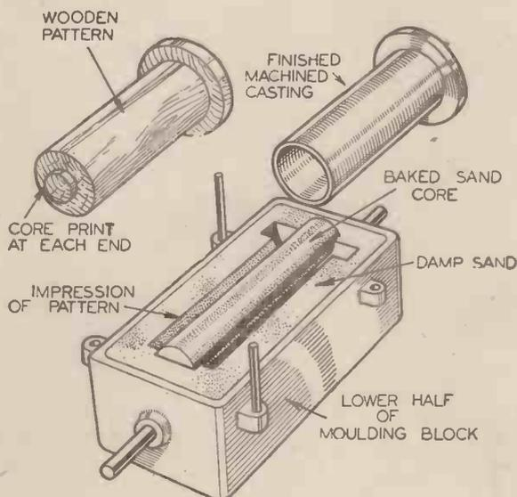
(Left) The principle on which a simple casting is made. The pattern is pressed first into one half of a sand mould, and then into the other. The core, made from sand, bound with oil and baked, is placed between the two halves of the mould when they are assembled. Only the bottom half of the moulding box is shown in the illustration. (Right) Diagrammatic illustration of the method of making a centrifugal casting
