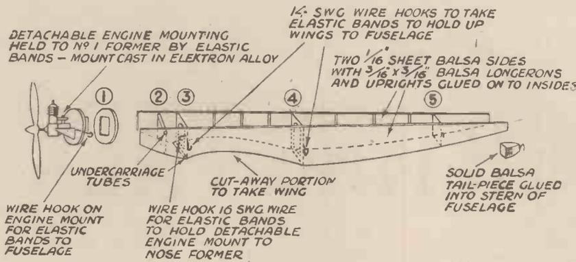
Fig. 3.—Method of assembling the fuselage
