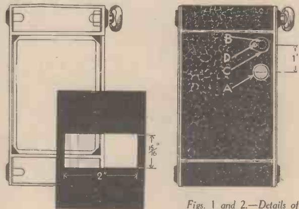
Figs. 1 and 2.—Details of the black mask and how the back cover of the camera is drilled
