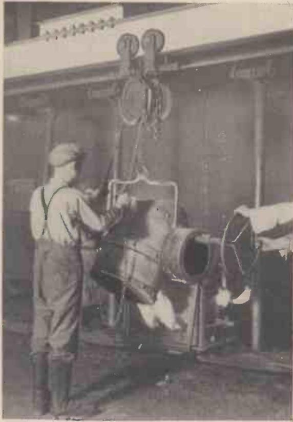
The ladle filled with molten metal being tipped to pour a cylinder-clock casting
