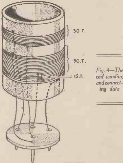
Fig. 4—The coil winding and connecting data
