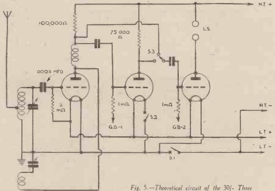
Fig. 5.—Theoretical circuit of the 30/- Three
