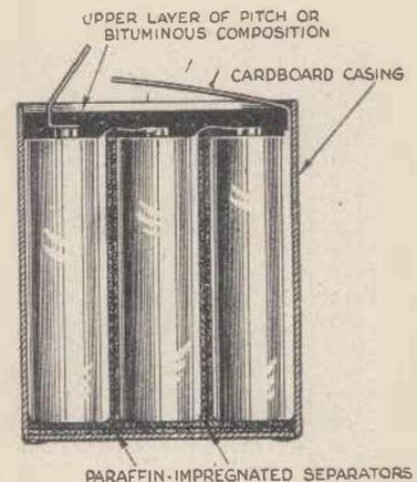
Showing the arrangement of the individual cells in a "flat" pocket lamp battery
