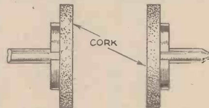
Fig. 7.—How the cork chucks are made
