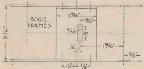
Fig. 7.—Bogie frames and stretcher plate
