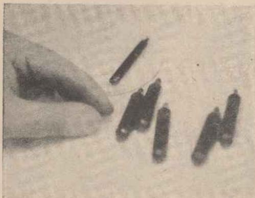
Owing to its corrosive nature, pure bromine is best sealed in a number of small glass tubes, in which condition it is best stored for future use
