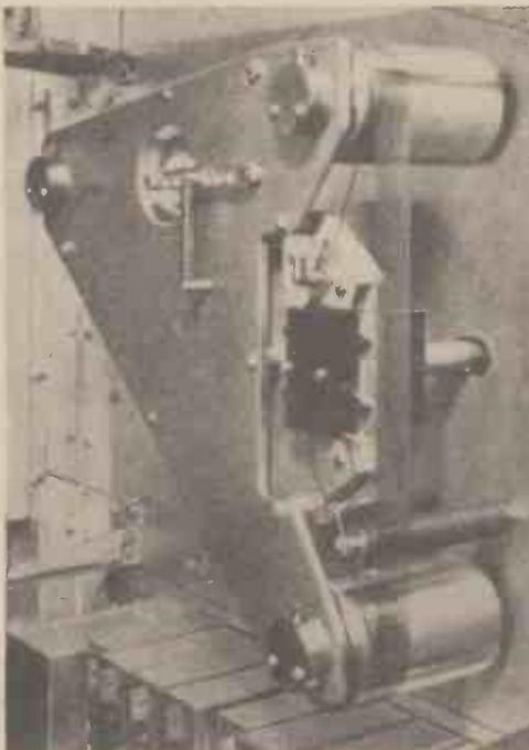
Fig. 3.—Front view of tape machine with cover removed
