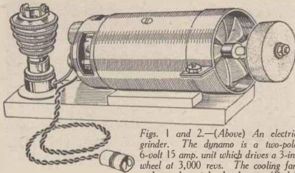
Figs. 1 and 2.—(Above) An electric grinder. The dynamo is a two-pole 6-volt 15 amp. unit which drives a 3-in. wheel at 3,000 revs. The cooling fan and guard are clearly shown. (Right) Parts of a 6-volt four-pole starter motor ready for rewinding
