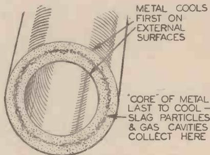
When a cylindrical casting is made with a sand mould and core, the outside surfaces of the metal tend to solidify first, an unreliable "core" results
