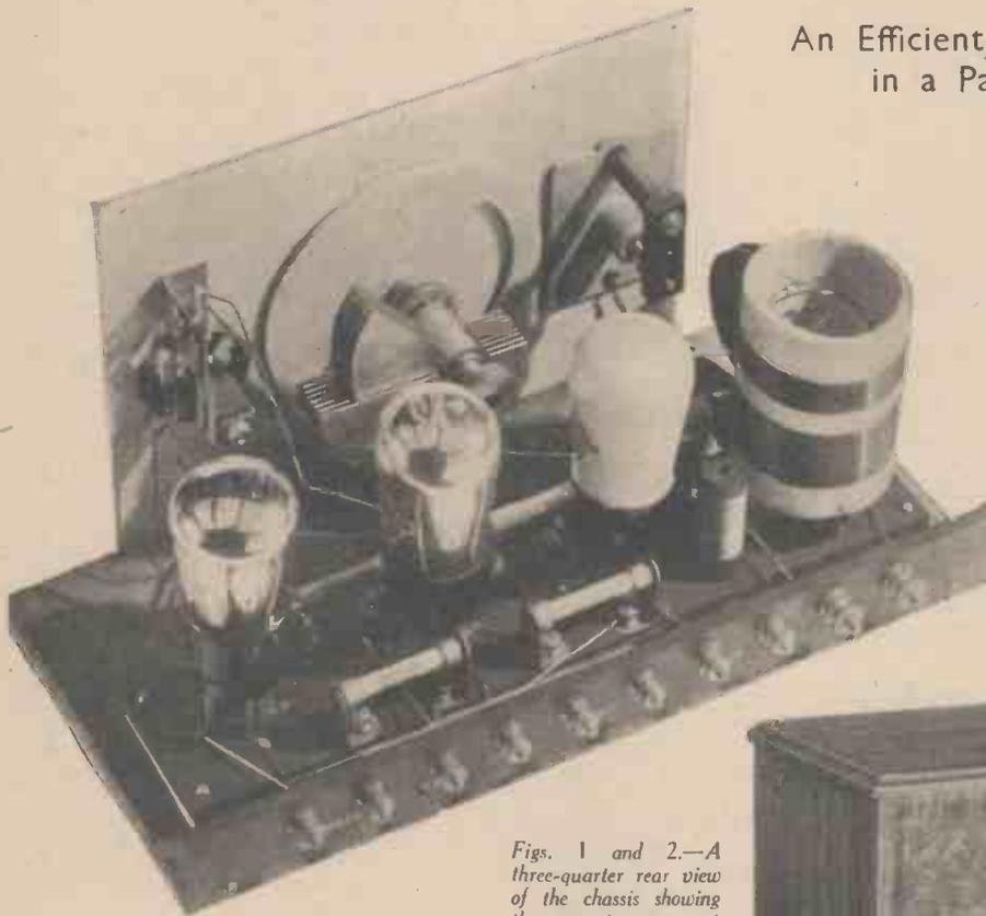
required. The reaction control is effected by means of a special moving plate type of condenser using the metal panel as one plate and a sheet of mica is supported to provide the dielectric. A threaded rod gives control over the moving plate and this operates most effectively in providing the reaction effects. The home-made coil has a suitable winding, of course, to ensure that reaction is smooth over the entire band.
