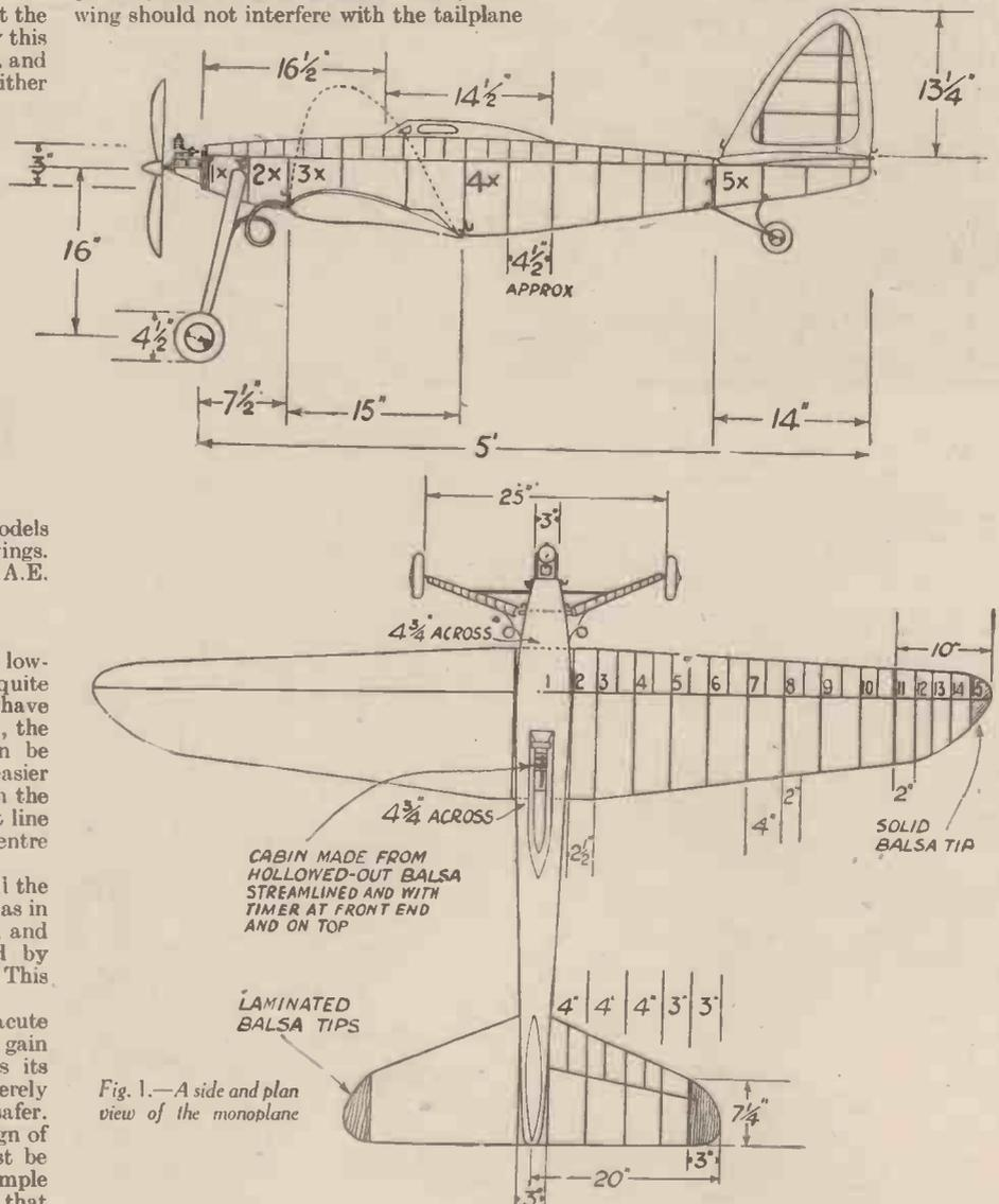
Fig. 1.—A side and plan view of the monoplane
