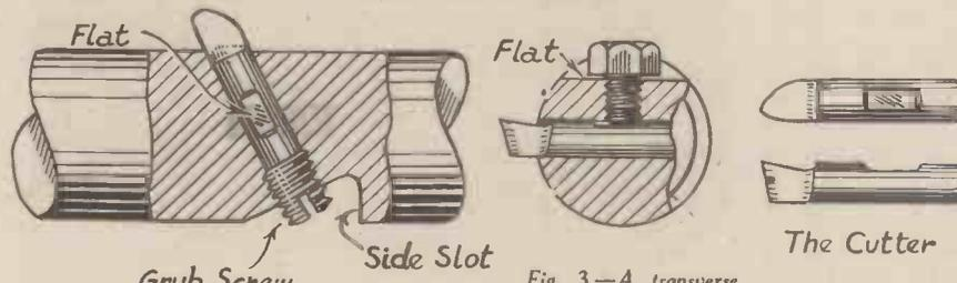
Fig. 2.—A sectional view of the bar showing the position of the cutter
