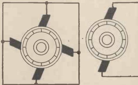
Fig. 3.—(Left) Brush connections for a two-pole motor. (Right) Connections for a four-pole motor
