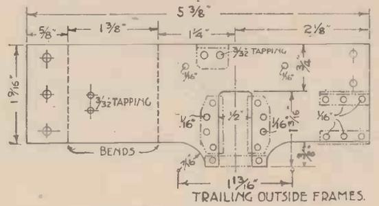
Fig. 8.—Detail of outside trailing frames
