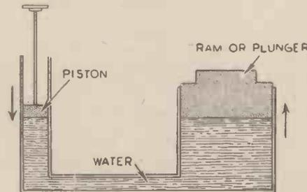
Illustrating the principle of the hydraulic press which Bramah raised to the status of an engineering creation
