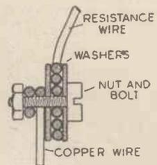
Figs. 4 and 5.—(left) Details of the former. (Right) The connections on the heater or resistance unit
