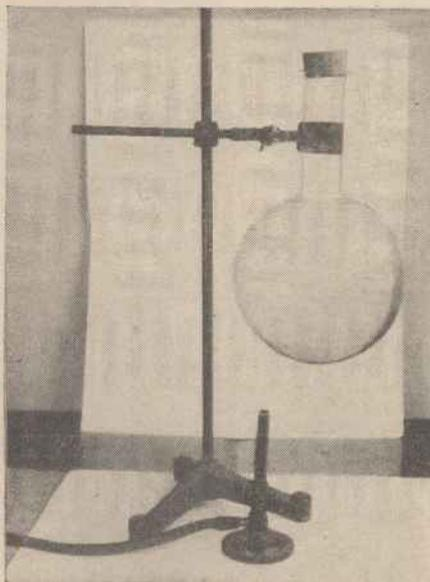
By heating a few crystals of iodine in a large flask, the beautiful and characteristic violet vapour of the element may readily be discerned
