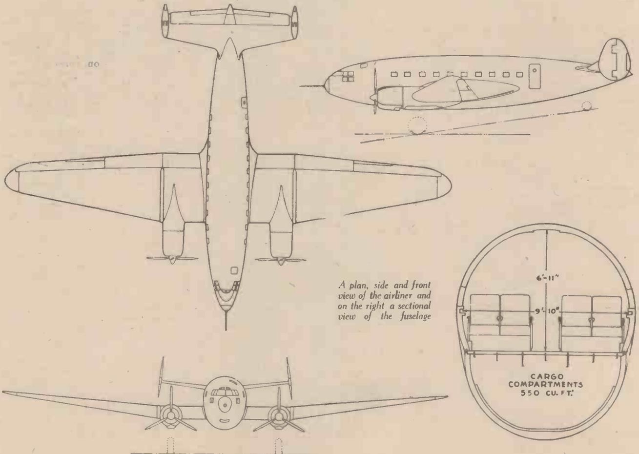
A plan, side and front view of the airliner and on the right a sectional view of the fuselage
