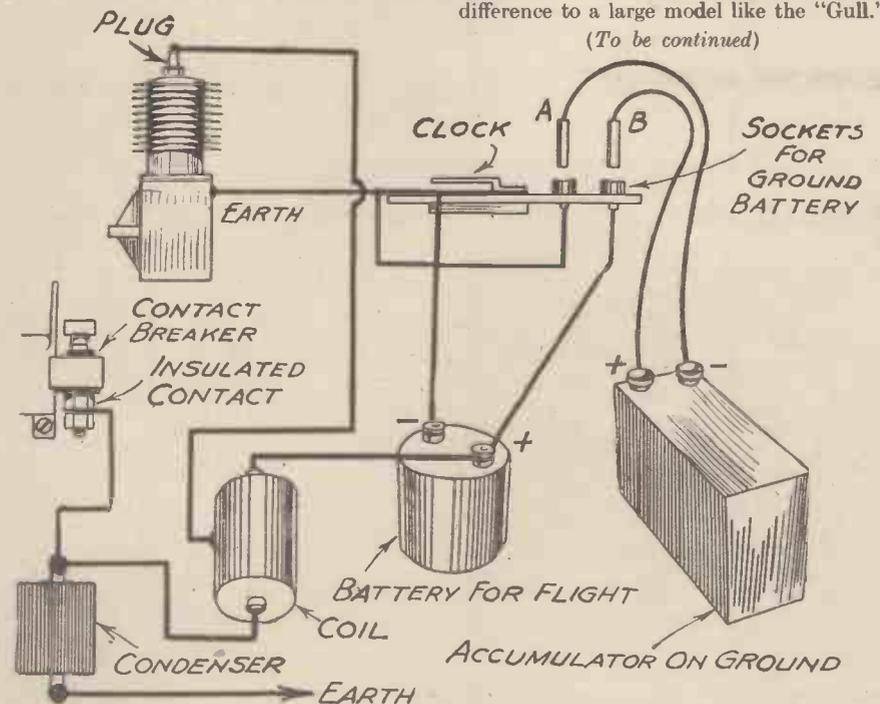
Fig. 4.—Wiring diagram of the ignition system
