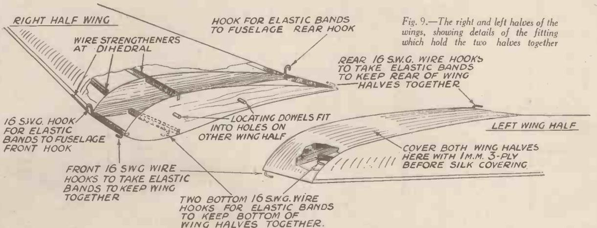
Fig. 9.—The right and left halves of the wings, showing details of the fitting which hold the two halves together
