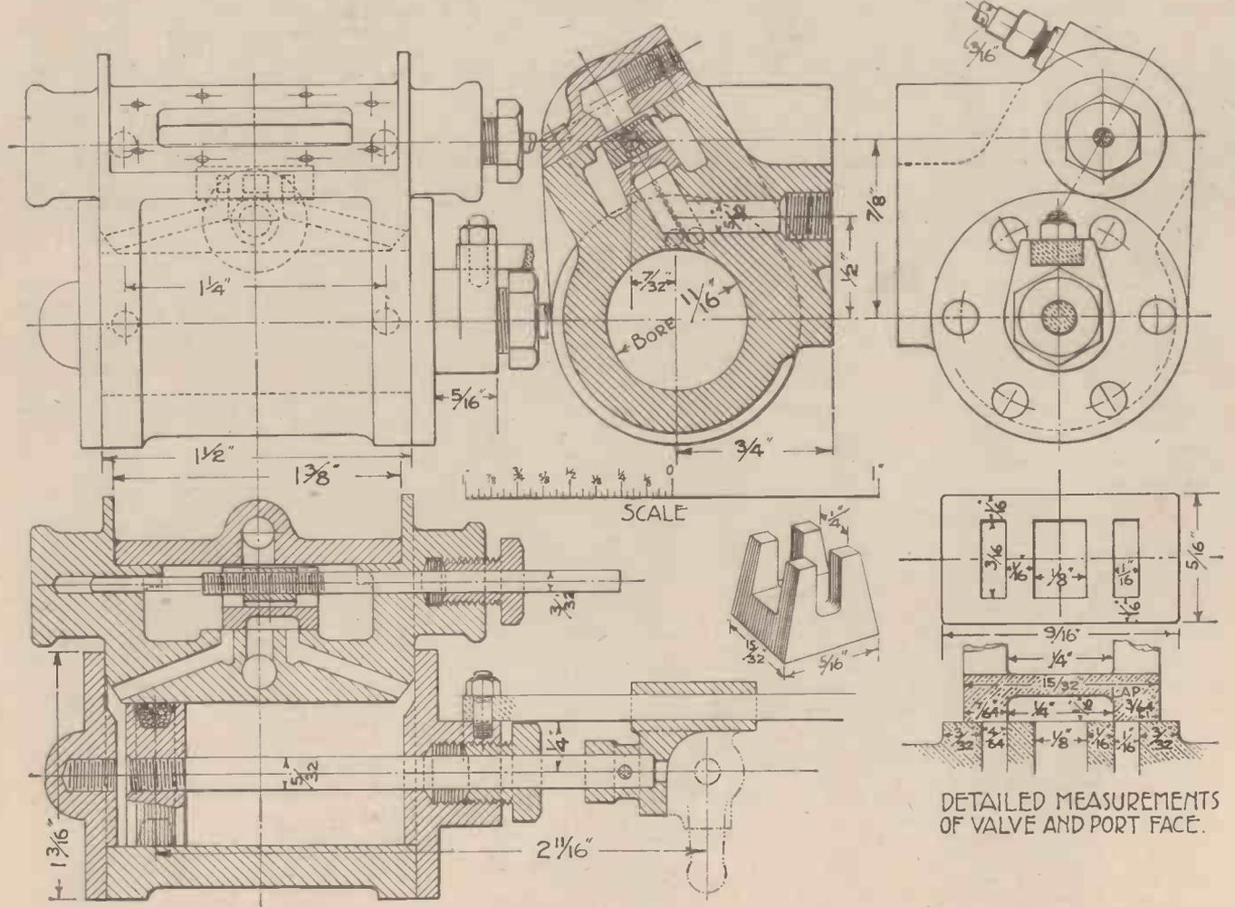
Fig. 21.—Details of cylinder, crosshead and slide-valve
