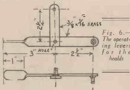
Fig. 6.—The operating levers for the healds
