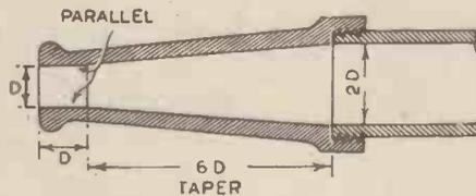
Fig. 4.—A nozzle for a Pelton wheel
