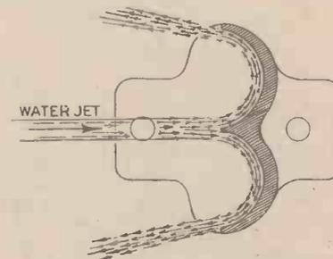
Fig. 3.—Bucket casting for a Pelton wheel
