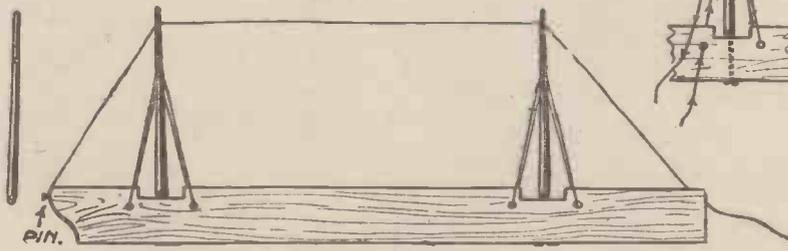
Figs. 2 and 4.—(Left) The masts, two of which are required, with holes bored for the rigging and for securing it to the hull. (Right) The hull with masts and rigging attached
