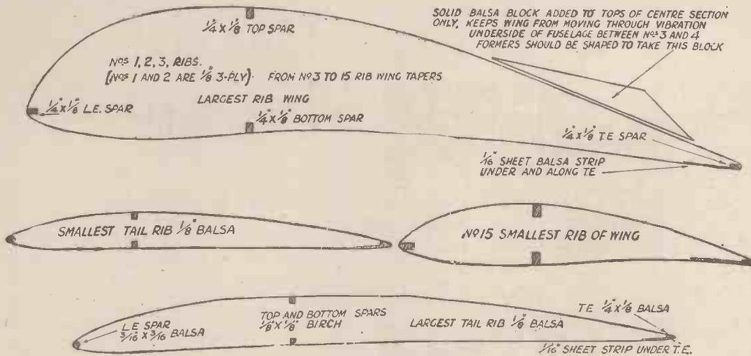
Fig. 7.—The wing and tail sections
