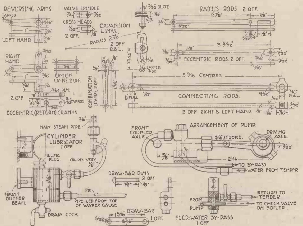
Fig. 24.—Details of valve gearing, connecting rods, boiler feed pump, and displacement lubricator
