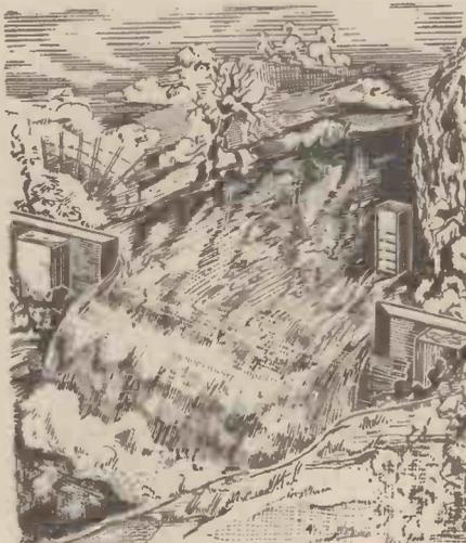
Fig. 2.—A notched weir for measuring water flow
