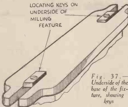
Fig. 37.—Underside of the base of the fixture, showing keys
