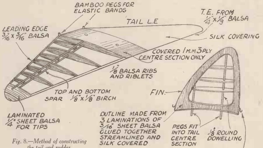
Fig. 8.—Method of constructing the tail and rudder
