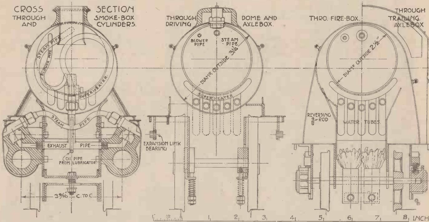
Figs. 15 to 18.—Cross sections through cylinders, boiler and firebox, and rear elevation of cab fittings
