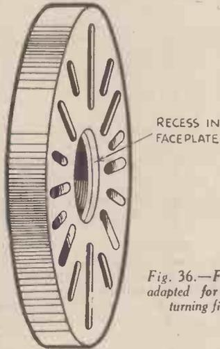
Fig. 36.—Face-plate adapted for mounting turning fixtures
