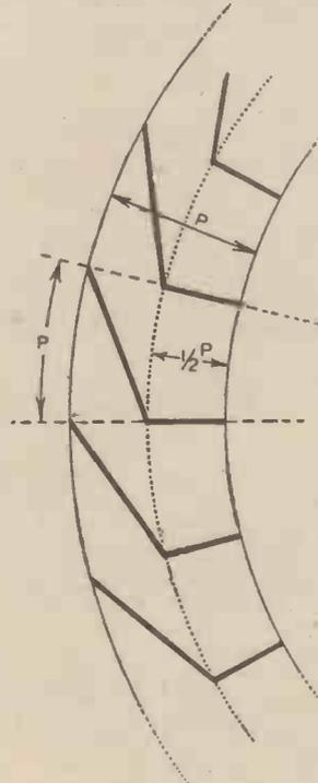
Fig. 8.—Proportions of buckets for overshot and breast wheels. There should be about two buckets for each foot in diameter of the water wheel, and the wheel should be arranged to deal with the required quantity of water without waste over the tops of the buckets
