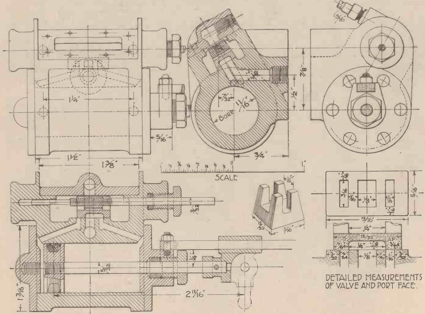
Fig. 21.—Details of cylinder, crosshead and slide-valve
