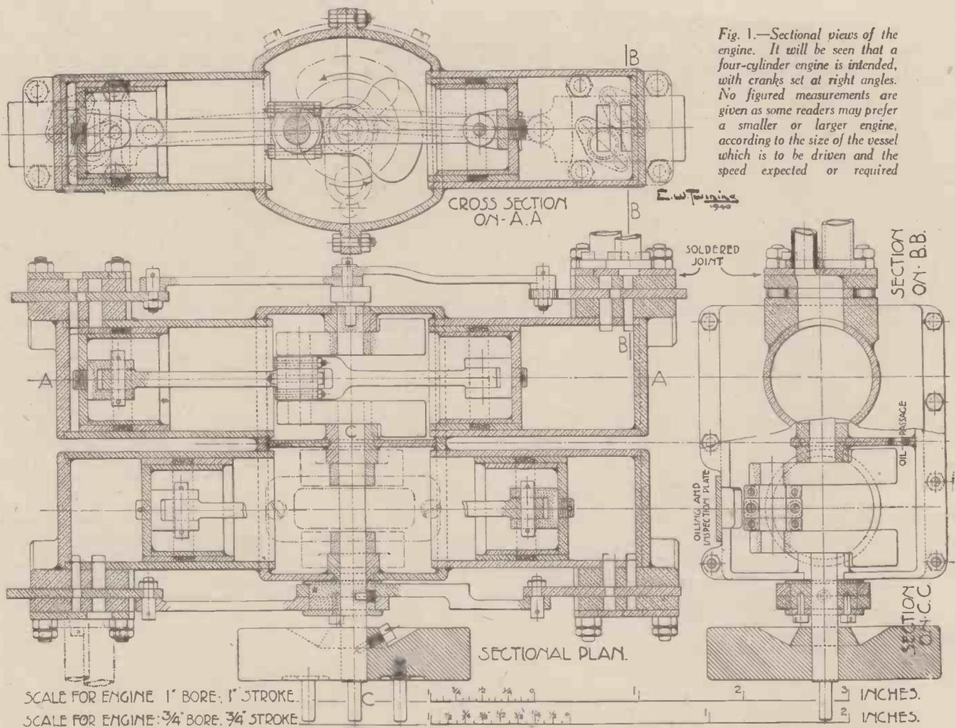
Fig. 1.—Sectional views of the engine. It will be seen that a four-cylinder engine is intended, with cranks set at right angles. No figured measurements are given as some readers may prefer a smaller or larger engine, according to the size of the vessel which is to be driven and the speed expected or required.
