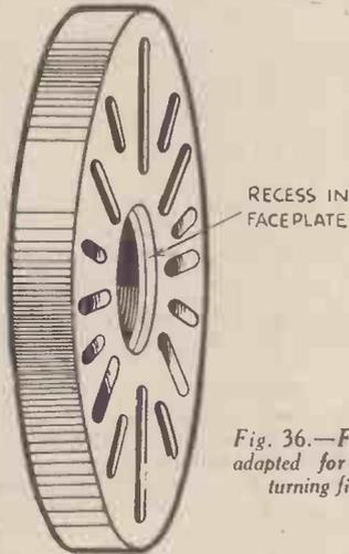
Fig. 36.—Face-plate adapted for mounting turning fixtures
