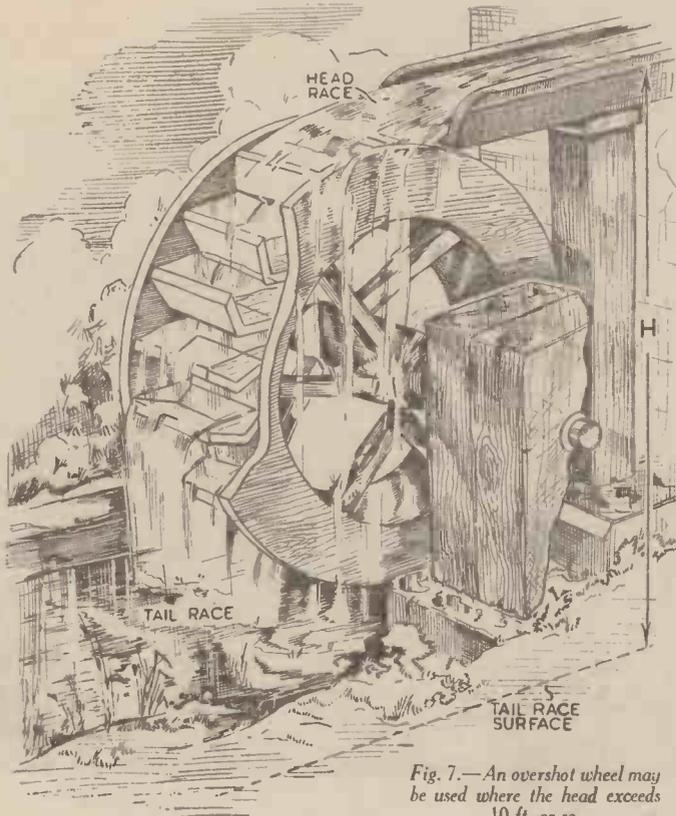
Fig. 7.—An overshot wheel may be used where the head exceeds 10 ft. or so
