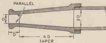
Fig. 4.—A nozzle for a Pelton wheel
