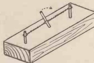
Figs. 2 to 5.—(Left) The construction of the healds and (below) the method of making the wires. (Centre) Adjusting the wires. (Right) The central eyelet should be in a plane at right angles to the eyelets at each end
