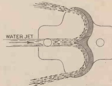
Fig. 3.—Bucket casting for a Pelton wheel
