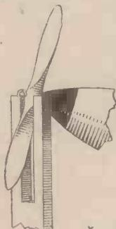
Fig. 1 and 2. — (Left) Showing how the propeller is held by the forked arm (Below) A detail sketch showing the mechanism for launching the aeroplane
