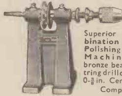
Superior quality Combination Grinding, Polishing and Drilling Machine. "Ollite" bronze bearings, self-centring drillchuck. Capacity 0-3/8 in. Centre height 6 in. Complete 15/6
