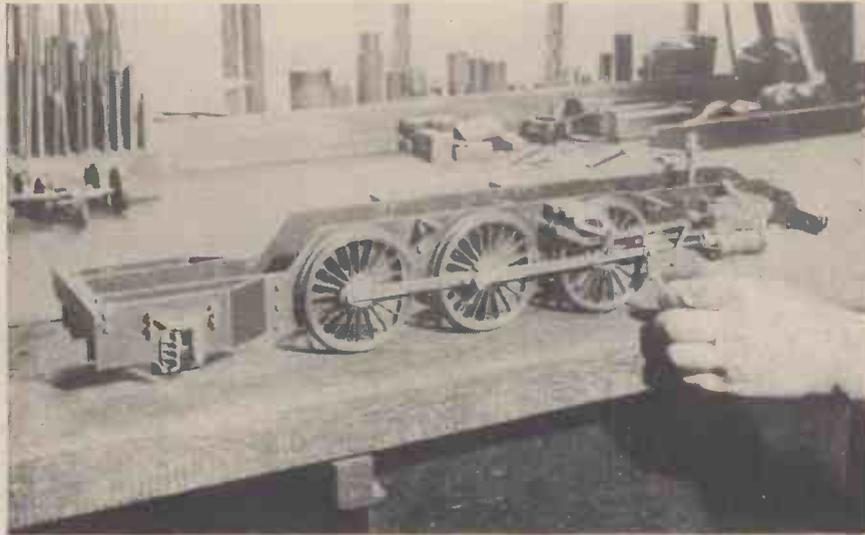
Fig. 19.—Engine main frames, with driving wheels, cylinder and valve gear assembled on one side
