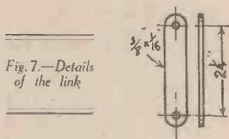
Fig. 7.—Details of the link
