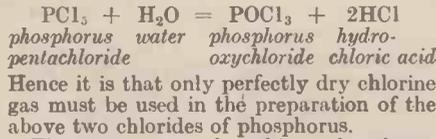
The best way of making phosphorus oxychloride,  $POCl_3$ , is to add water to phosphorus pentachloride very carefully, and drop by drop until the white solid turns to a liquid.
