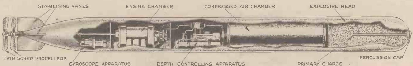
Showing the internal construction of a torpedo
