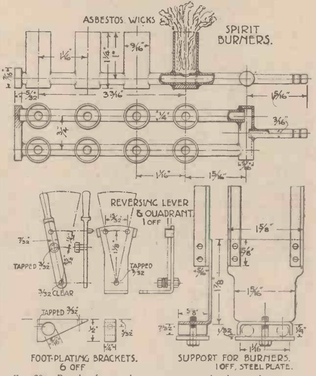
Fig. 20.—Details of spirit burner, supporting bracket, and reversing lever and quadrant
