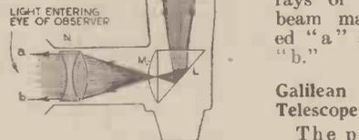
Fig. 6.—Vertical section of a periscope showing the optical system and path of the central beam
