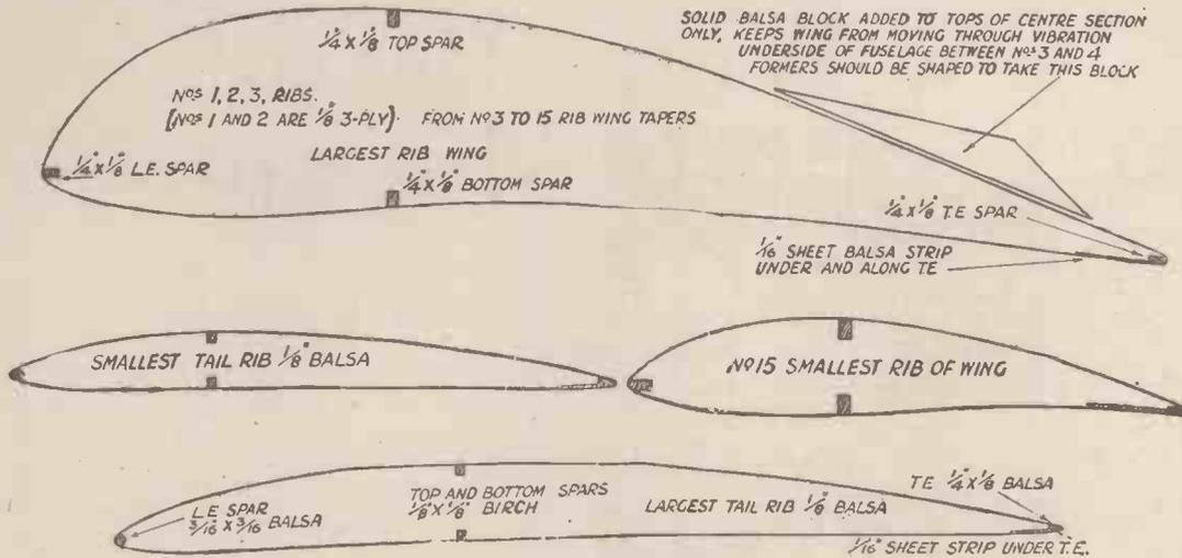
Fig. 7.—The wing and tail sections
