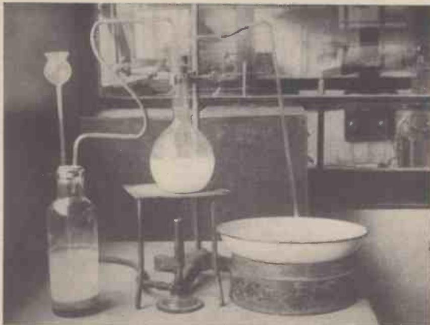
Preparing hydrogen phosphide or "phosphine" by boiling yellow phosphorus with caustic soda solution in a flask. The bottle on the left contains marble chippings and dilute hydrochloric acid in order to generate carbon dioxide gas which is led into the flask to displace the air therein before beginning the preparation of the hydrogen phosphide
