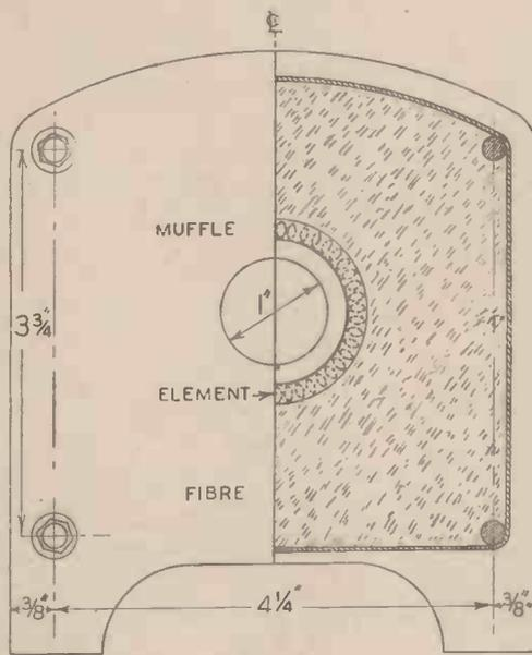
Fig. 1.—An end elevation in part section of a 200 watt electric furnace
