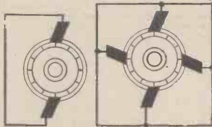
(Left) The brush connections for a two-pole motor. (Right) Connections for a four-pole motor. In practice carbon brushes are placed radially to the centre and not at an angle
