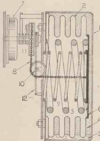
A sectional view of the motor of the Atmos clock
