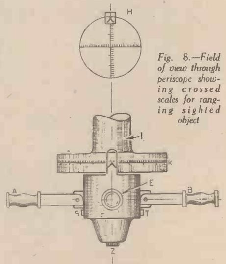
Fig. 8.—Field of view through periscope showing crossed scales for ranging sighted object
