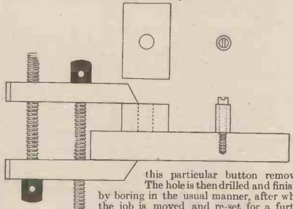
this particular button removed. The hole is then drilled and finished by boring in the usual manner, after which the job is moved and re-set for a further boring, and so on until completed.
