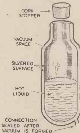
Cross section through a vacuum flask
