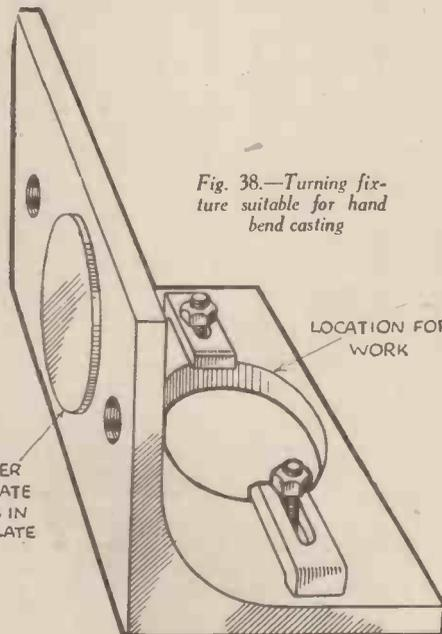
Fig. 38.—Turning fixture suitable for hand bend casting
