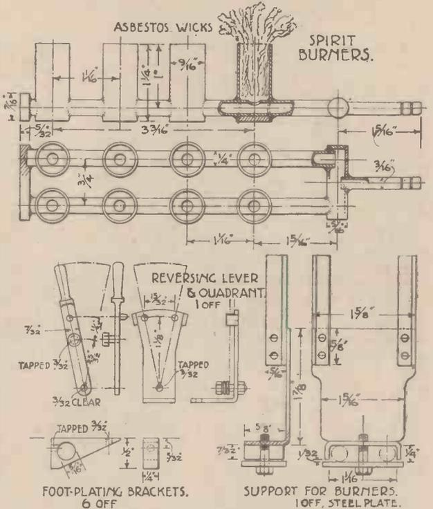
Fig. 20.—Details of spirit burner, supporting bracket, and reversing lever and quadrant
