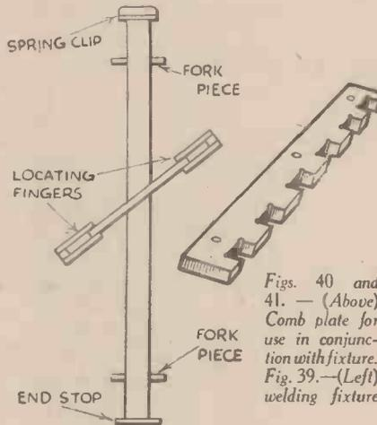
Figs. 40 and 41. — (Above) Comb plate for use in conjunction with fixture. Fig. 39. — (Left) welding fixture
