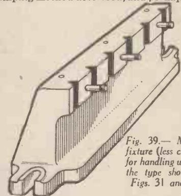
Fig. 39.—Milling fixture (less clamps) for handling work of the type shown in Figs. 31 and 32
