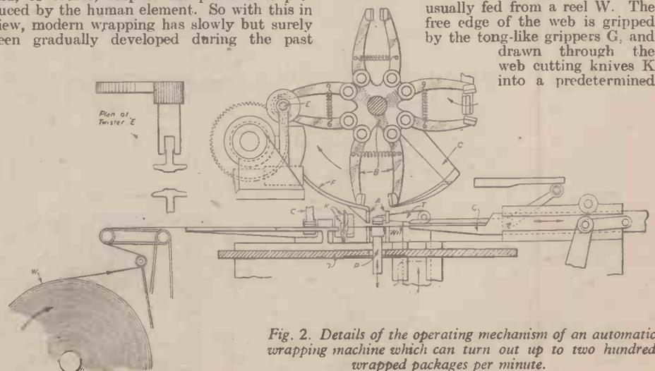
Fig. 2. Details of the operating mechanism of an automatic wrapping machine which can turn out up to two hundred wrapped packages per minute.
