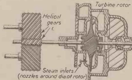
Fig. 7. Reduction gears used with the De Laval turbine.
