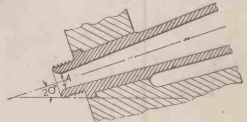
Fig. 3. Section of steam nozzle, showing the jet taper.
