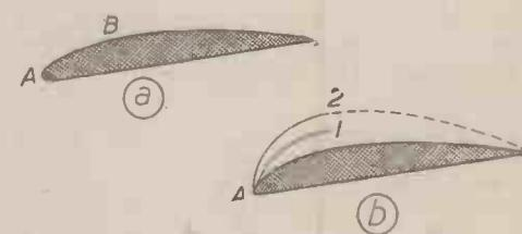
Fig. 4. The principle of the variable wing flap.
