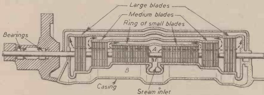
Fig. 6. Longitudinal section of a modern steam turbine.
