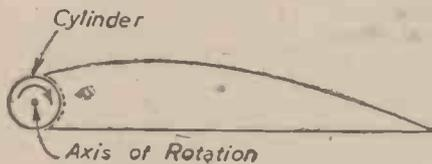
Fig. 6. Rotating cylinder device.
