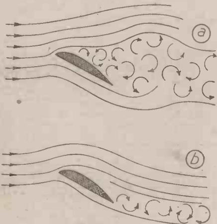
Fig. 2. Illustrating the air flow over a stalled wing.
