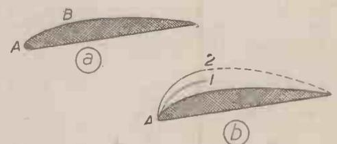
Fig. 4. The principle of the variable wing flap.
