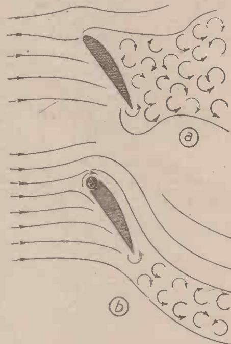
Fig. 7. Diagrams illustrating the effect of increased angle of attack.
