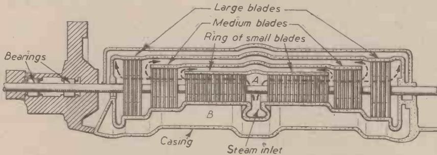
Fig. 6. Longitudinal section of a modern steam turbine.
