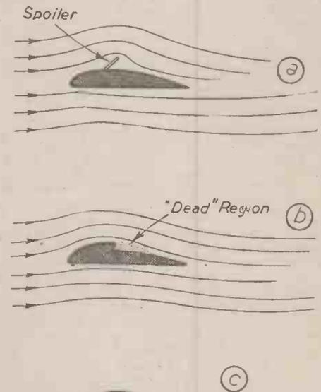
Fig. 3. Illustrating the effect of using a "spoiler."
