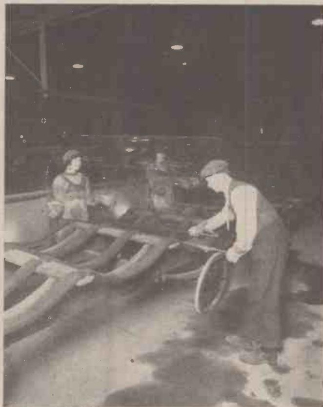
Fig. 4. A section of a glass cylinder being split into "shaws" before flattening.
