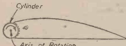
Fig. 6. Rotating cylinder device.
