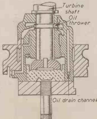
Fig. 4 (left). Section through the step bearing of a Curtis turbine.
