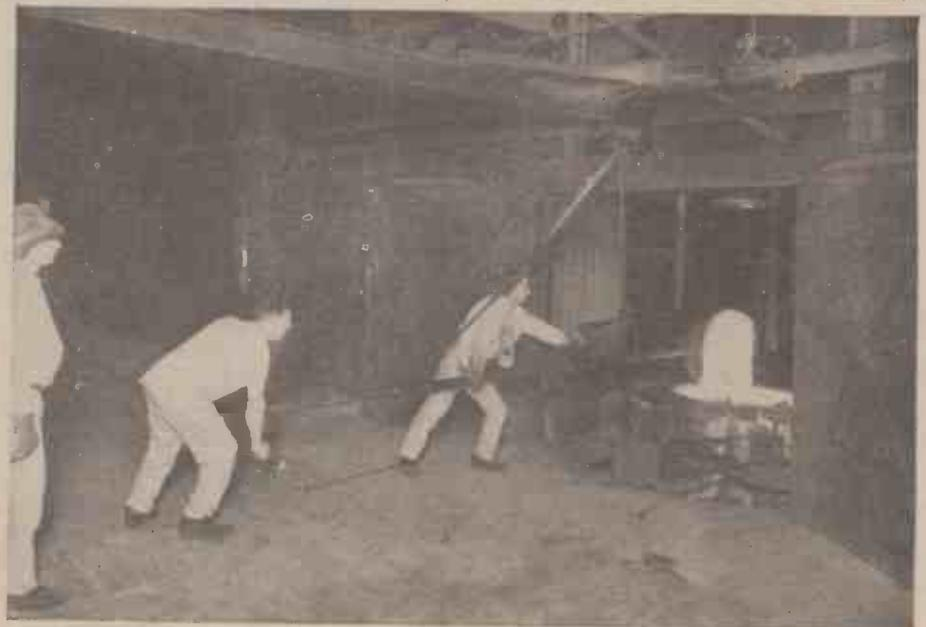
Fig. 1. Teeming the molten glass into the double-sided crucible, or drawing pot.
