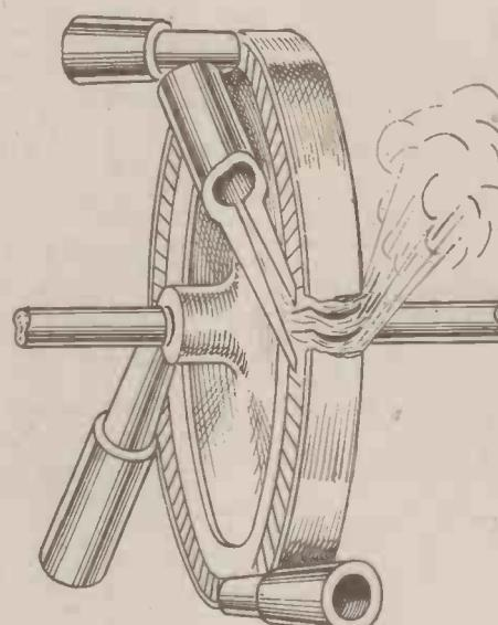
Fig. 2. The principle of the De Laval steam turbine.
