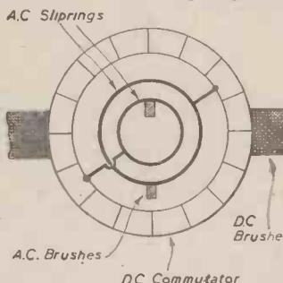
Converting a 6-volt generator to supply D.C. by adding slip-rings
