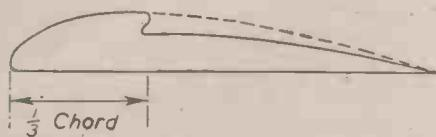
Fig. 1. The principle of the stepped wing.
