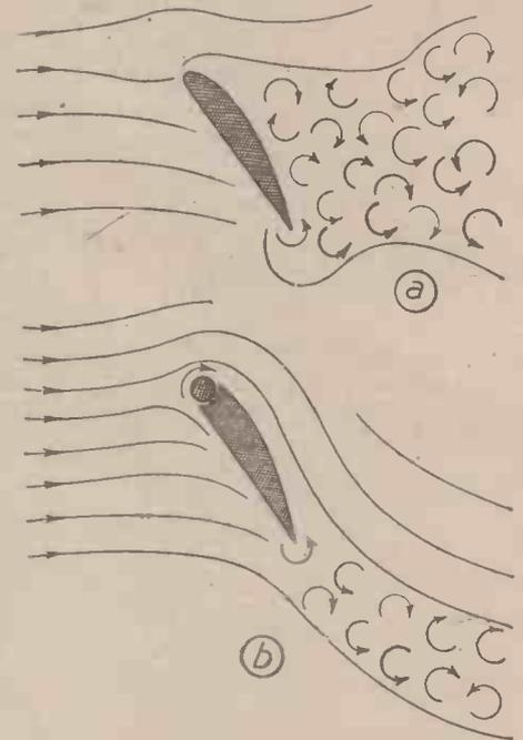
Fig. 7. Diagrams illustrating the effect of increased angle of attack.
