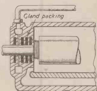
Fig. 5 (right). Section of a typical turbine bearing, showing the glands.
