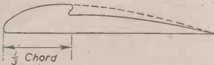
Fig. 1. The principle of the stepped wing.
