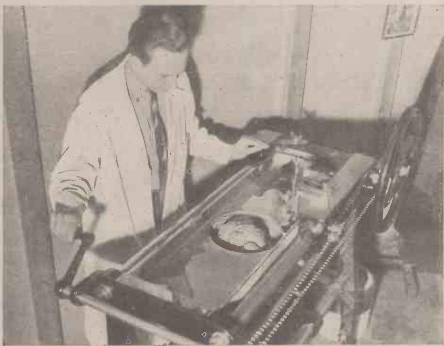
A brain microtome for cutting sections of the brain as thin as 5/2,500 thousands of an inch.
