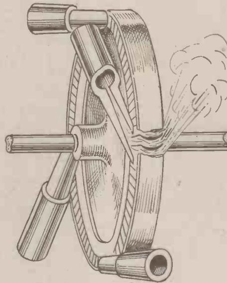
Fig. 2. The principle of the De Laval steam turbine.
