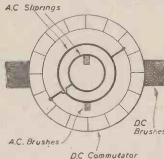
Converting a 6-volt generator to supply D.C. by adding slip-rings
