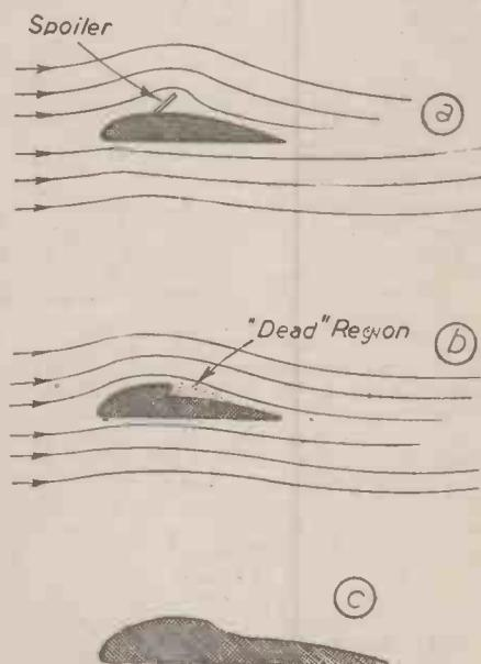
Fig. 3. Illustrating the effect of using a "spoiler."
