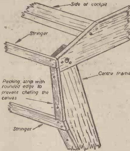
Fig. 8.—Detail of centre frame showing packing strips.
