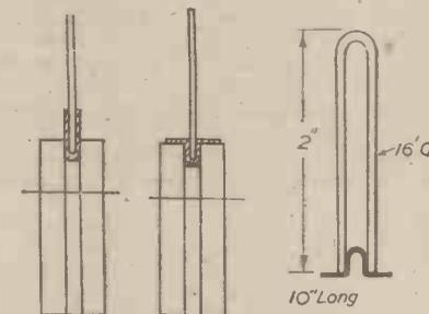
Figs. 6 and 7.—Method of forming the rail.
