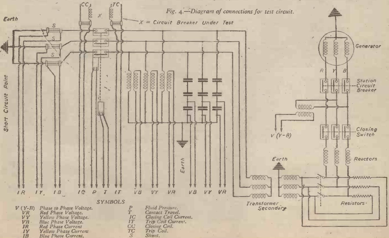
Fig. 4.—Diagram of connections for test circuit.
