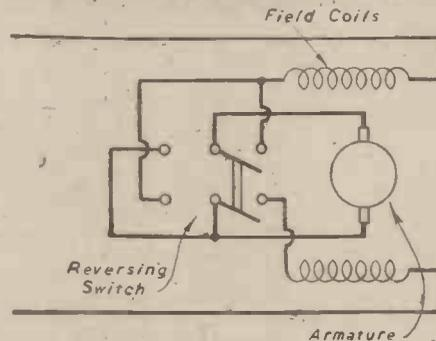
Connections for a double-pole two-way switch for reversing an A.C. motor.
