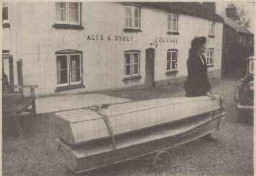
The two halves of the canoe strapped together and ready for transport.
