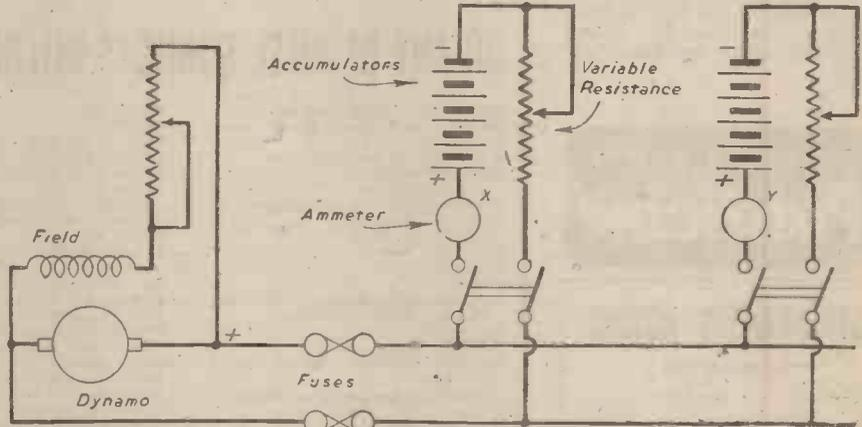
Diagram of two charging circuits with independent control.
