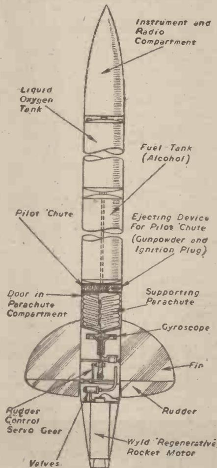
Fig. 24.—Diagram of the Wyld sounding rocket (1938).
