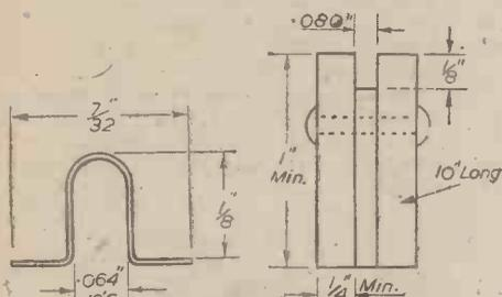
Fig. 1.—Simple rail section.
