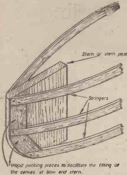
Fig. 7.—Method of securing stringers at the stem and stern posts.
