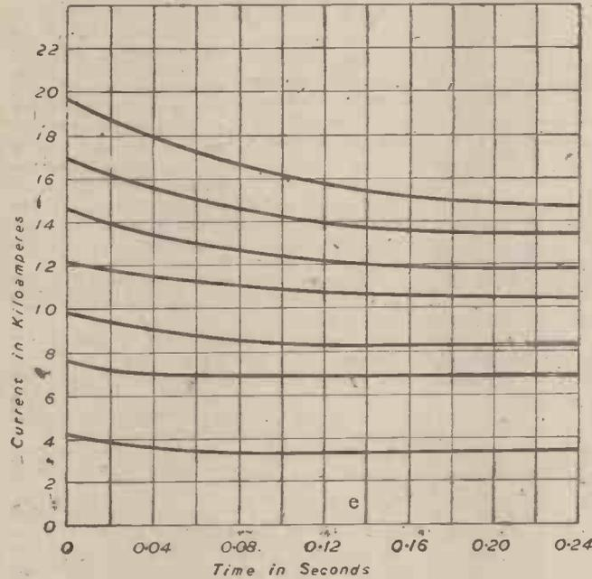
Fig. 5.—Curves showing decrement of current for various values of test circuit reactance.
