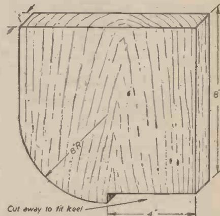
Fig. 5.—Dimensions for stem and stern post.
