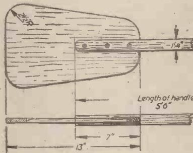
Fig. 11.—Details of construction of double-ended paddles.
