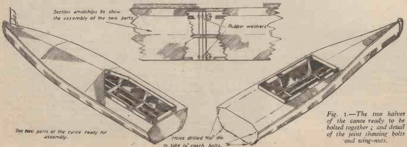
Fig. 1.—The two halves of the canoe ready to be bolted together; and detail of the joint showing bolts and wing-nuts.
