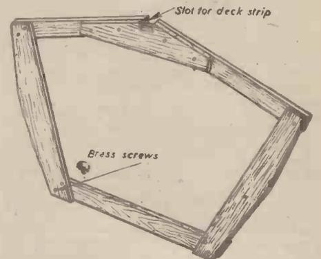
Fig. 2.—General construction of the cross-frames.
