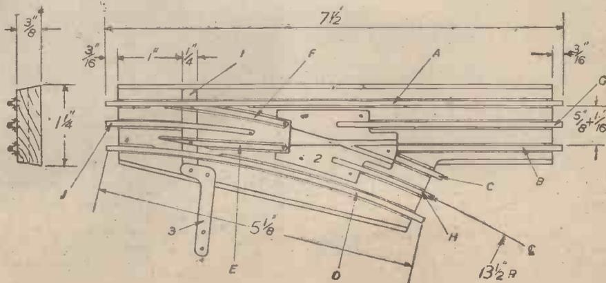
Fig. 9.—Layout for right-hand points.
