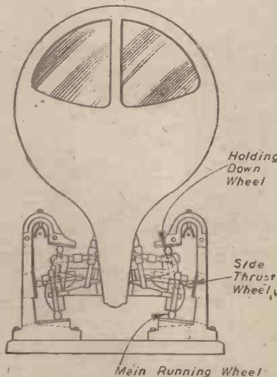
End view of a "Hyperailion" vehicle, showing the arrangement of running wheels and track.
