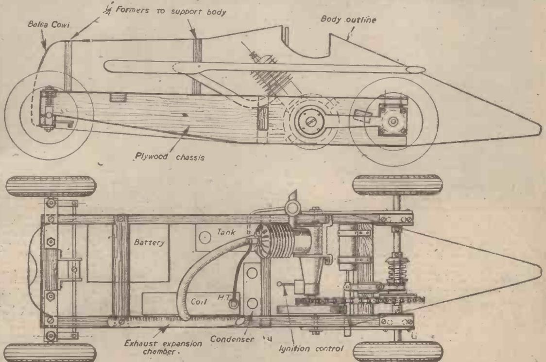
Figs. 1 and 2.—Side elevation and chassis plan of the Leyland Thomas 10 c.c. petrol-driven racing car. (One quarter full size.)
