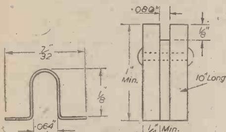
Fig. 1.—Simple rail section.
