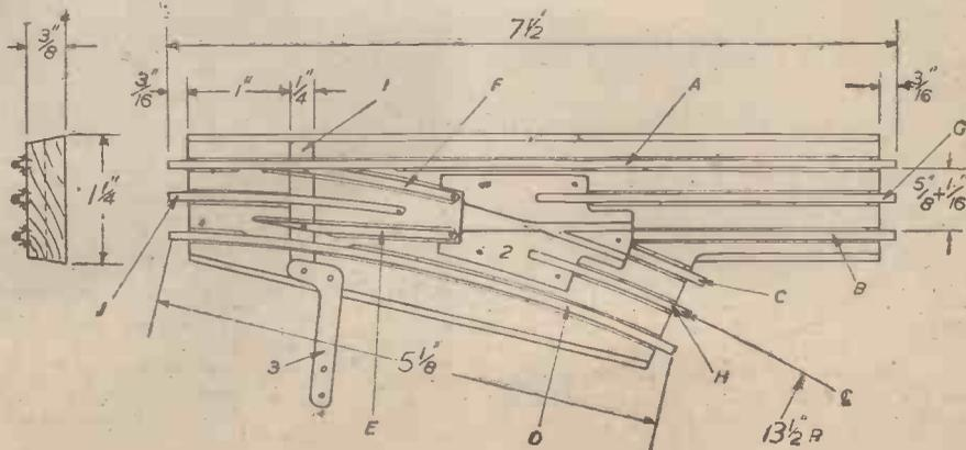
Fig. 9.—Layout for right-hand points.
