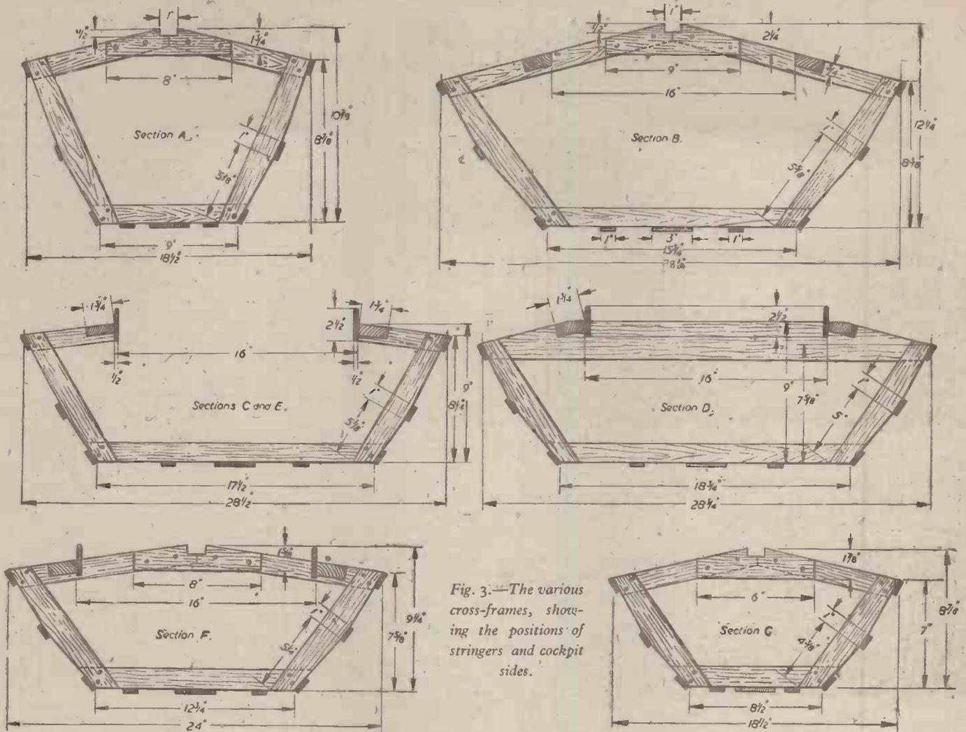
Fig. 3.—The various cross-frames, showing the positions of stringers and cockpit sides.
