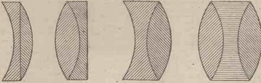
Typical sections of compound lenses constructed on Dollond's achromatic principle.
