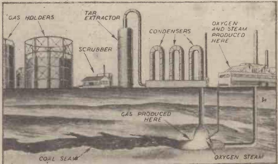
Pictorial diagram of the Gorlovka experimental mine for the underground gasification of coal.
