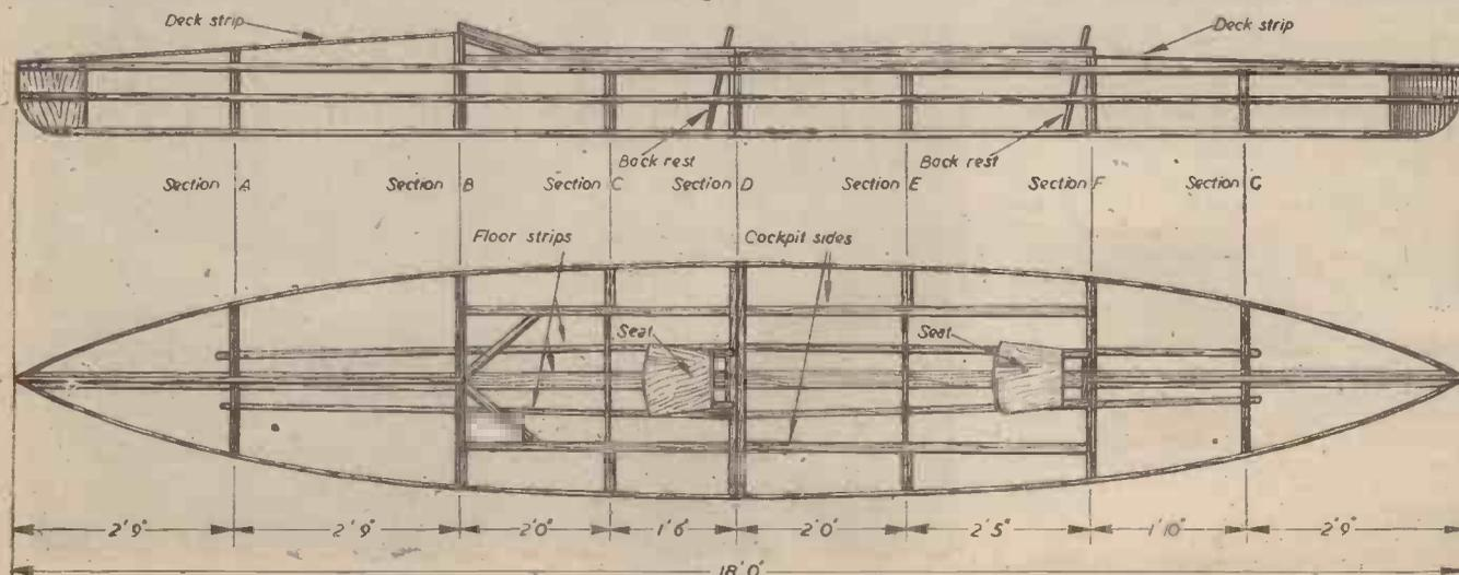
Fig. 6.—Side elevation of complete framework, and plan showing main keel strips and deck framework.
