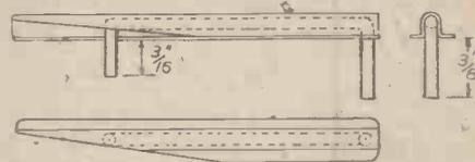
Fig. 13.—Method of joining the tongue of the moving rails.
