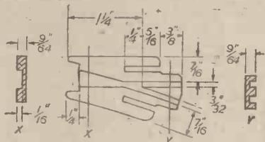
Fig. 11.—Insulating junction plate.
