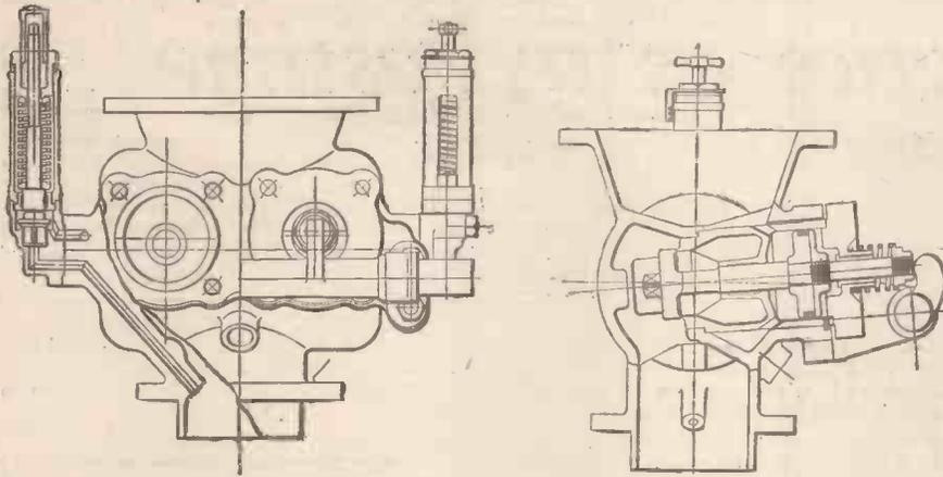
Fig. 13. — Double full-bore marine type safety valve with relay cylinders included (Cockburns, Ltd.).
