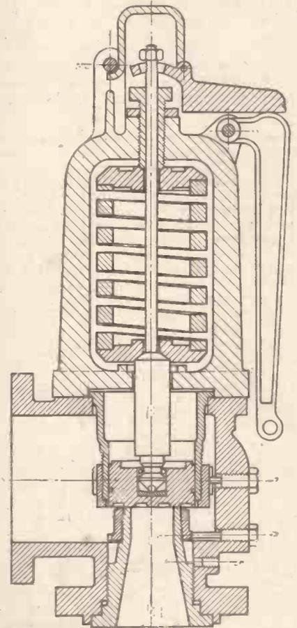
Fig. 6.—"Pop" safety valve (Crosby Valve & Engineering Co.).
