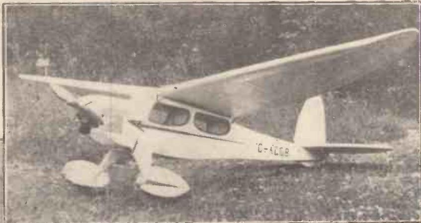
Fig. 4.—The Bowden White-Wings diesel model has a large wing area 6ft. 6in. span with central chord 16in. on an elliptical wing. The fuselage is 'almost crash proof' and is covered with balsa sheet. The model can be flown by a 3.5 c.c. to a 5 c.c. diesel.
