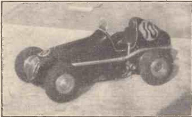
Fig. 3.—Mr. Baigent's 0.9 c.c. baby diesel car that travels at great speed around a special track. The model is a scale Austin 7 racer and is only 8in. long.
