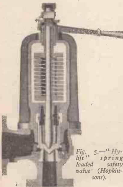
Fig. 5.—"Hy-lift" spring loaded safety valve (Hopkinsons).
