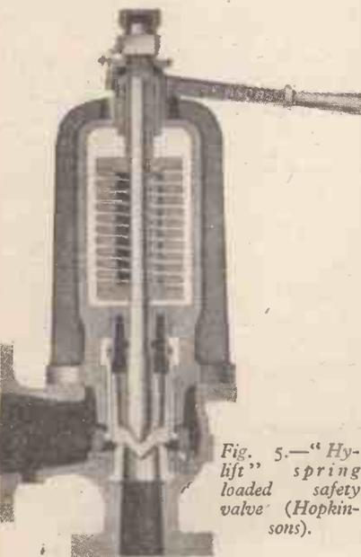
Fig. 5.—"Hy-lift" spring loaded safety valve (Hopkinsons).
