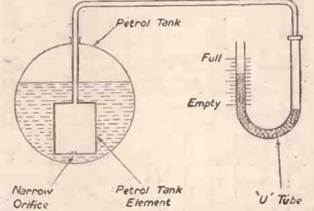
Diagram of a hydrostatic petrol-level indicator.—(R. W. Cooper.)
