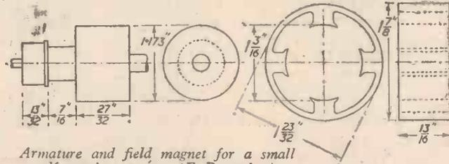
Armature and field magnet for a small self-starting motor.—(E. Rawnsley.)
