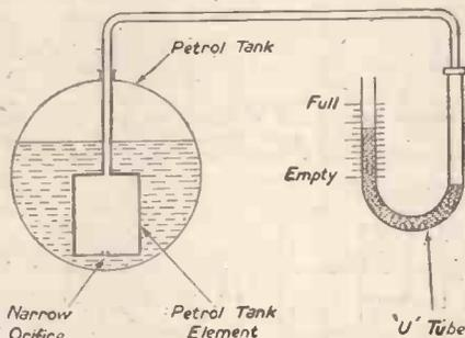
Diagram of a hydrostatic petrol-level indicator.—(R. W. Cooper.)
