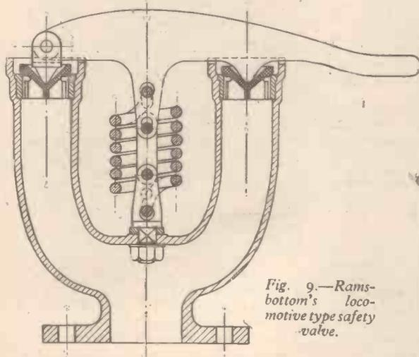
Fig. 9.—Ramsbottom's locomotive type safety valve.
