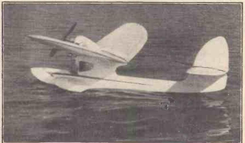
Fig. 1.—C. E. Bowden's baby model flying-boat of 38in. span called the "WEE SEA BEE" is seen powered by a 1 c.c. British diesel engine. The model is sitting on top of the water ready to take off because of its light waterloading.
