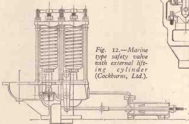
Fig. 12.—Marine type safety valve with external lifting cylinder (Cockburns, Ltd.).
