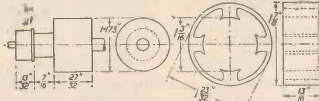
Armature and field magnet for a small self-starting motor.—(E. Rawnsley.)
