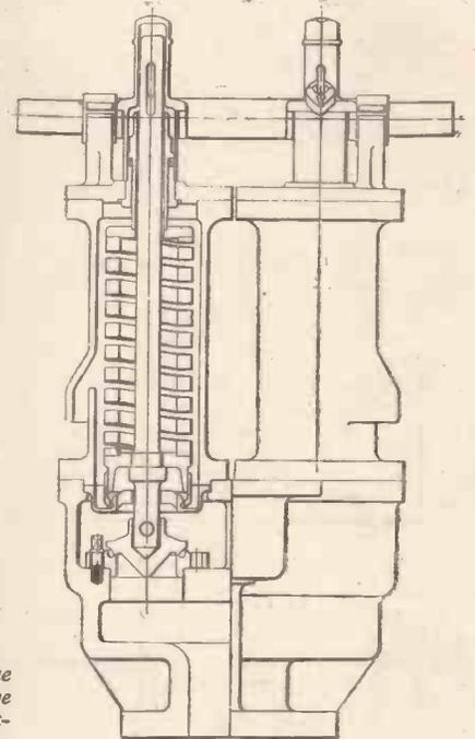
Fig. 14. — High lift marine type safety valve for saturated steam (Cockburns, Ltd.).
