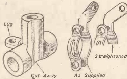
Fig. 3.—Detail of T-tube.
