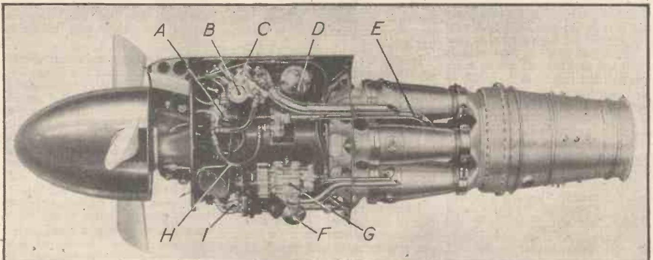
Key diagram showing the disposition of the chief component parts. A. Oil distributor and high pressure relief valve; B. Main oil pressure filter; C. Main pressure and high pressure pump; D. Tachometer; E. Air cooling pipe to rear bearing; F. Fuel flow control filter; G. Gas starter; H. Air feed pipe to front bearing; I. Tecalemit micro pump for rear bearing.
