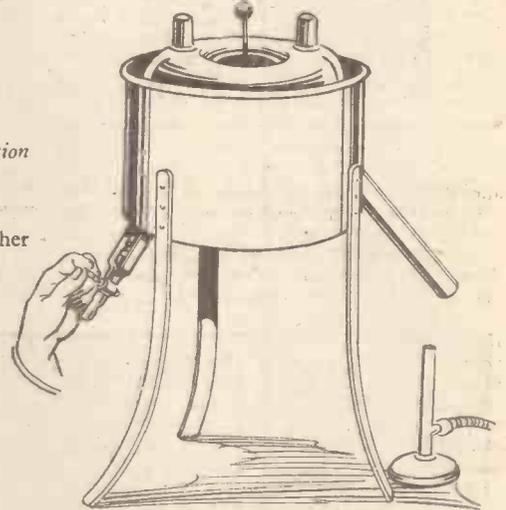
Fig. 9.—An industrial viscosimeter used for the purpose of determining oil viscosities.
