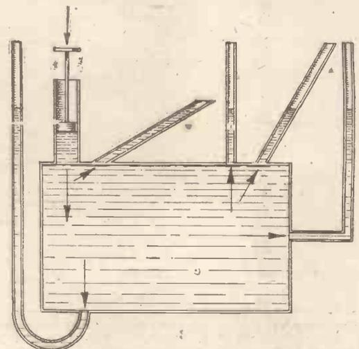
Fig. 6.—Apparatus demonstrating the fact that a liquid transmits an applied pressure in all directions.
