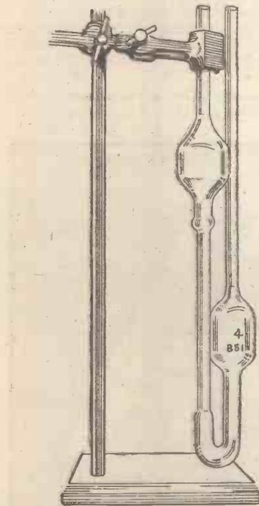
Fig. 10.—A capillary-tube viscosimeter used for "fine" determinations of viscosity in absolute units.
