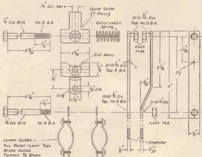
Fig. 1.—Details of the operating mechanism.
