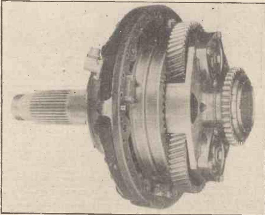
The reduction gear of the "Mamba" which reduces the 15,000 r.p.m. of the compressor and turbine to a propeller speed of 1,450. The reduction gear ratio is .097 : 1. The annulus gear and two out of the three helical planet gears are visible. The gear at the rear of the planet carrier provides the drive for the engine auxiliaries.
