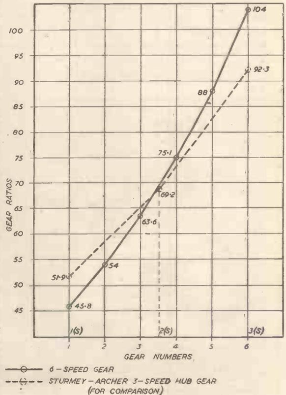
Fig. 5.—Graph indicating range of Sturmey-Archer hub gears.
