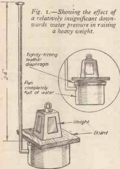
Fig. 1.—Showing the effect of a relatively insignificant downwards water pressure in raising a heavy weight.
