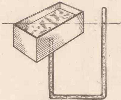
Fig. 5.—Illustrating the balancing of a large mass of water by a much smaller mass.
