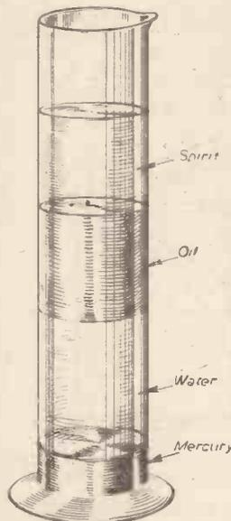
Fig. 2.—Showing the manner in which a four-layer column of non-miscible liquids can be formed, the liquids ranging themselves in order of gravity.
