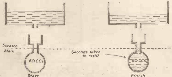
Fig. 8.—Diagram illustrating the principle of the modern industrial viscosimeter. The time taken to discharge a given volume of liquid is noted.
