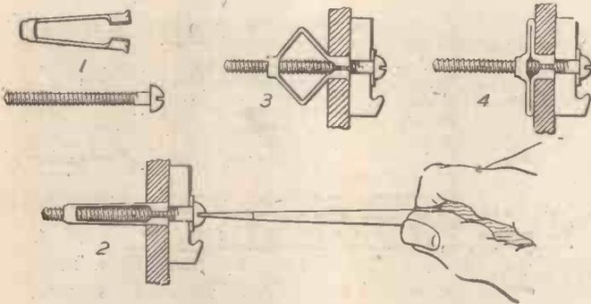
Method of fitting a Masonite Rawl Anchor
