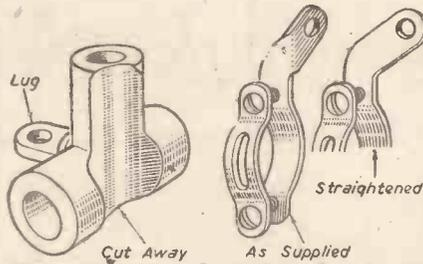
Fig. 3.—Detail of T-tube.
