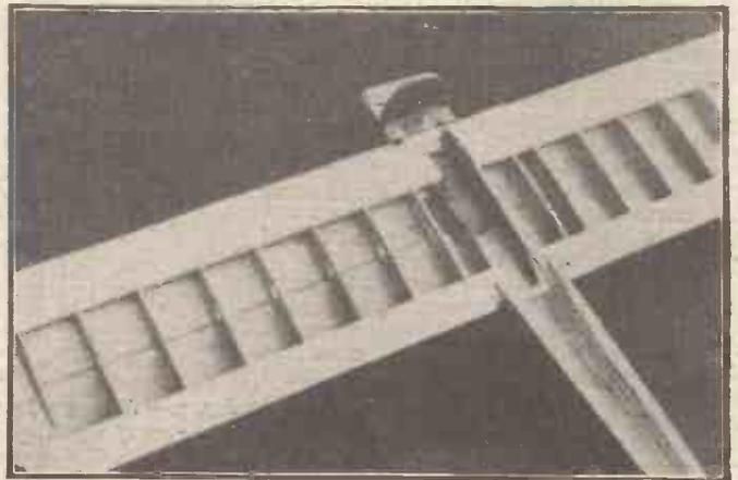
Fig. 28.—The control plate and connecting wires to wing tip and elevator horn, are now fitted internally on this model in order to reduce drag. The pivot bolt is very well reinforced with plastic wood to resist the pull of centrifugal force which may be considerable on a fast model.
