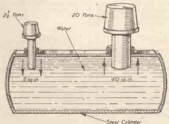
Fig. 3.—Illustrating the principle of the hydraulic press, as explained last month.
