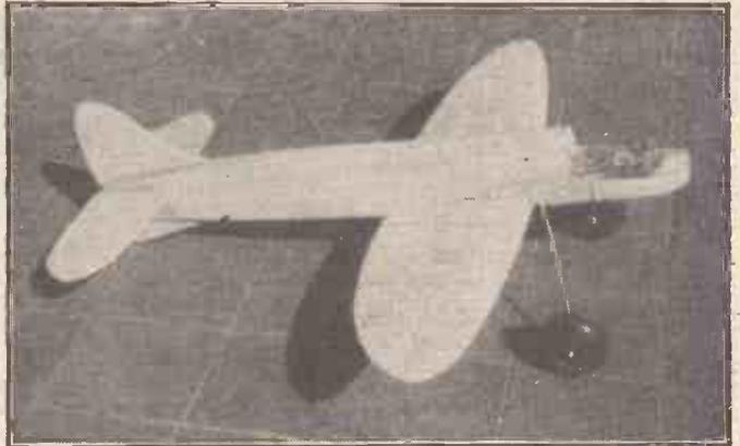
Fig. 31.—The model now has wing, tail and fin cemented in. Fillets of plastic wood strengthen and improve appearance. The fin should be laminated or of three-ply to withstand possible blows from landing turnovers!
