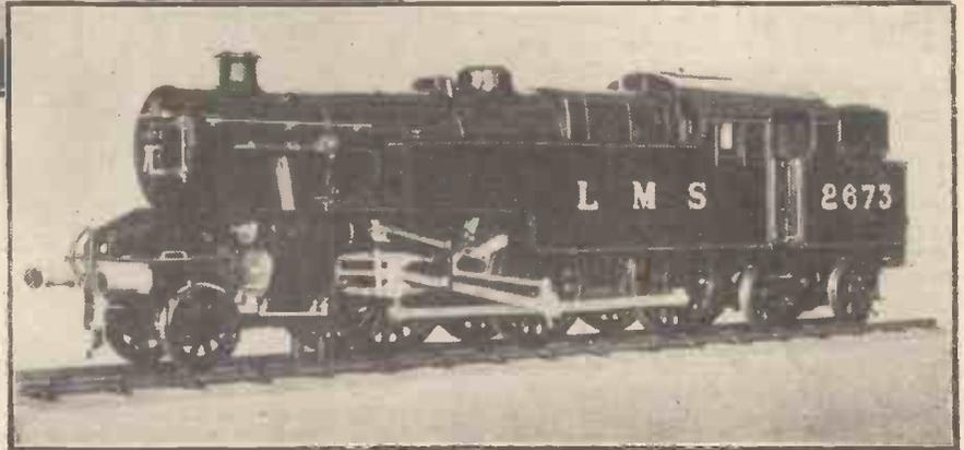
Fig. 5.—An excellent glass-case display model of a 2-6-4 class 4P tank locomotive, operating on the London and Midland Region of British Railways. Scale: ¼in. to 1ft.
