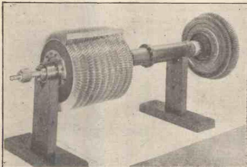
The "Mamba" 10-stage axial flow compressor and two-stage turbine assembly. The small size of the compressor is noticeable in comparison with the 12in. rule. It handles over 20 tons of air per hour.
