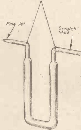
Fig. 7.—A Sprengel tube for the determination of liquid specific gravities.
