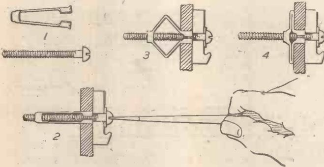
Method of fitting a Masonite Rawl Anchor
