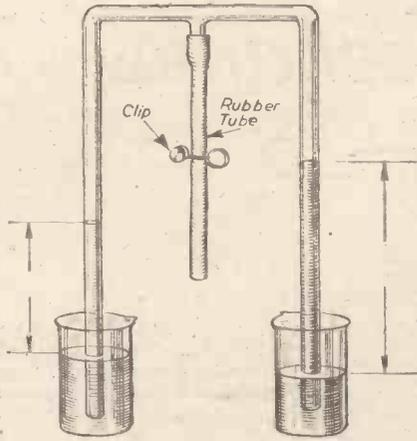
Fig. 4.—Hare's apparatus for comparing the gravities of liquids.
