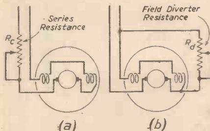
Fig. 16.—Speed control of a series motor by means of resistance.
