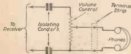
Fig. 1.—Circuit diagram.
