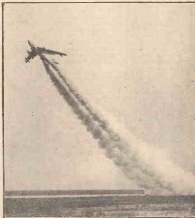
Six turbo-jets and eighteen dry-fuel rockets combine 42,000 lb. thrust in this spectacular take-off of the Boeing "Stratojet."
