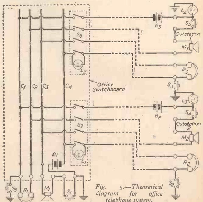
Fig. 5.—Theoretical diagram for office telephone system.
