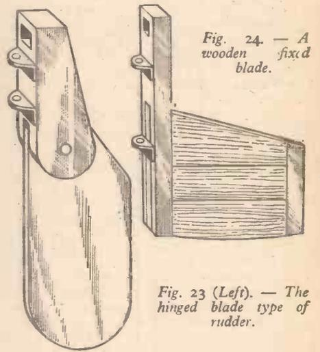
Fig. 23 (Left).—The hinged blade type of rudder.
