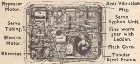
This unit represents a wealth of mechanical and electrical components. Consists of: Over 100 various precision gear wheels, helicals, rollers, spirals, levels, ratchets, worm drives, skew gears and variable pitch worm gear. Precision pitch stabilizing gyro unit. Servo syphon unit with four concertina type reservoirs, small bore servo tubes, servo switch.
