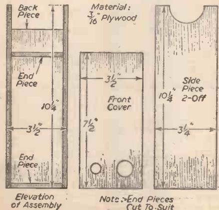
structed of 3/16in. plywood, glued and bradded together, the front being fastened by means of four small screws for ease of removal when changing batteries. The positions of the batteries, call lights and their associated switches are clearly shown in the photograph Fig. 4, while the diagram
