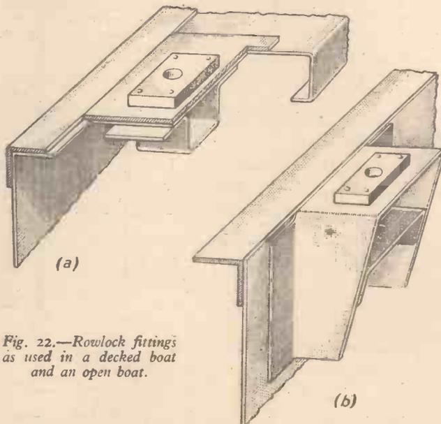
Fig. 22.—Rowlock fittings as used in a decked boat and an open boat.
