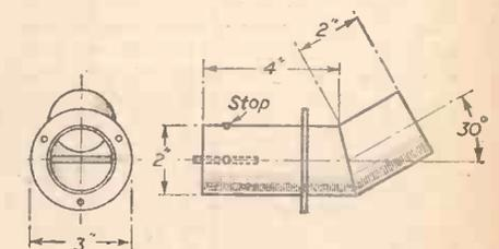
Fig. 5.—End and side views of the delivery piece.
