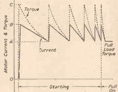
Fig. 14.—Starting of series motor.
