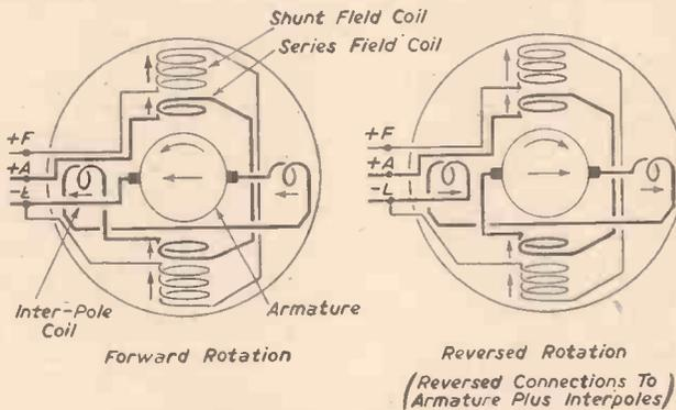
Fig. 19.—Method of reversing a compound motor.
