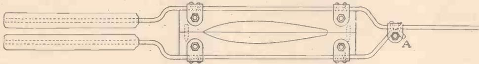
Fig. 5.—Suggested form of holder for dies for hand operation.
