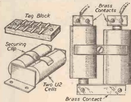
Fig. 3.—Batteries and connections.
