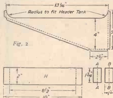
Figs. 2, 3 and 4.—Details of the top of heater, fan cover and supports.
