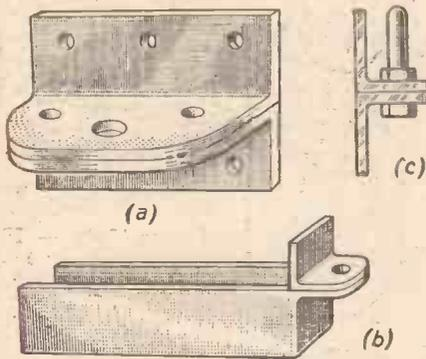
Fig. 25.—Details of rudder hinge fittings.
