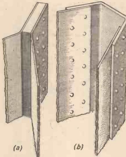
Fig. 21.—Methods of forming the stem.
