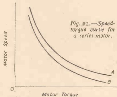
Fig. 12.—Speed-torque curve for a series motor.
