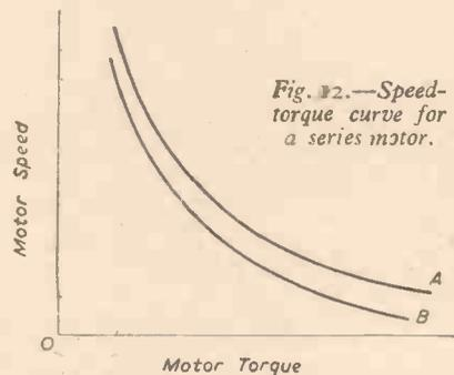
Fig. 12.—Speed-torque curve for a series motor.
