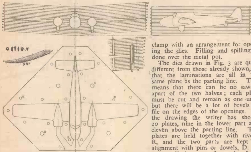
Fig. 3.—Laminated dies for casting aircraft models.
