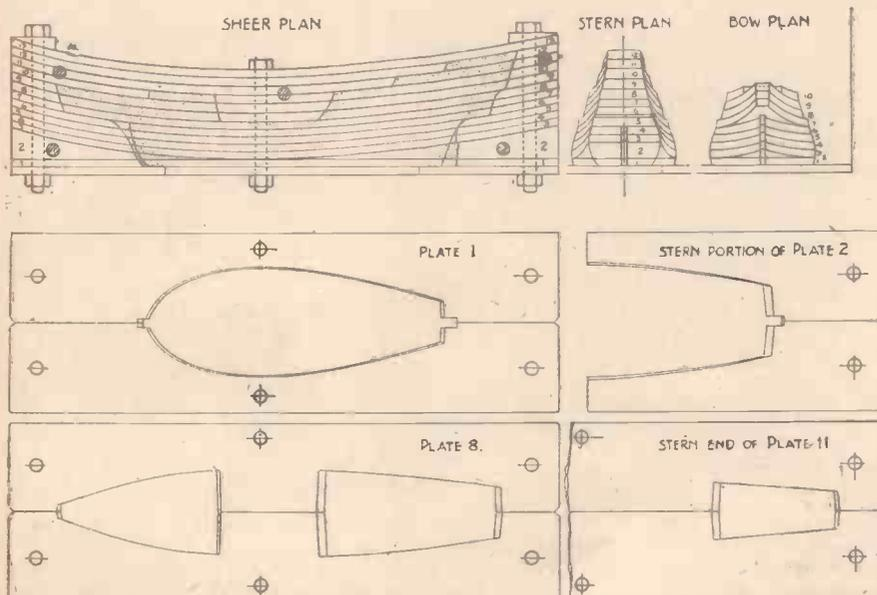
Fig. 2.—Dies for casting models of an Elizabethan ship.
