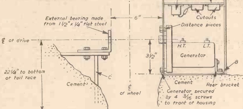
Fig. 3.—Arrangement of housing and external bearing.
