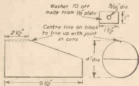
Fig. 2.—Details of forming block for shaping buckets
