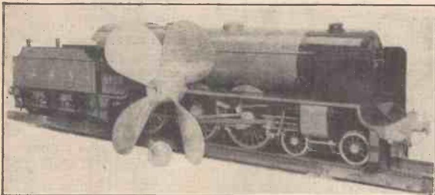
Fig. 5.—The 7½ in. gauge (1½ in. to 1 ft. scale) Royal Scot locomotive built to the order of Mr. Pardoe of Peru. This locomotive is adapted for oil firing. As a comparison in size, the four-blade propeller in front of the Royal Scot is a model, built to the same scale as the locomotive, of a propeller of one of the latest Orient Line ships; the new Orcades.
