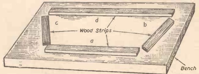
Fig. 29.—Jig for assembling frames.
