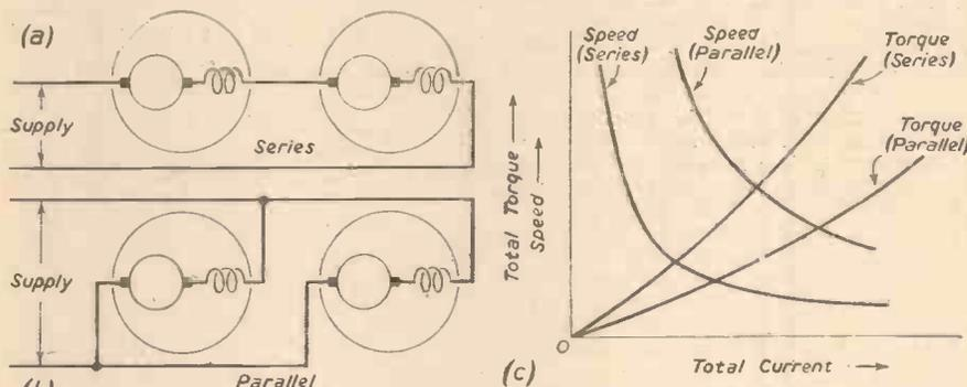
Fig. 17.—Series-parallel control of two series motors.
