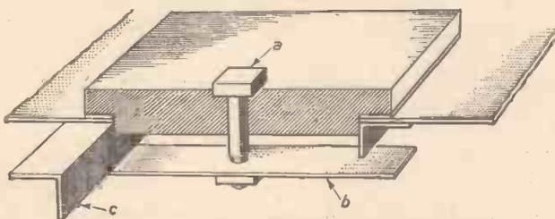
Fig. 27.—Sectional view of a watertight hatch.
