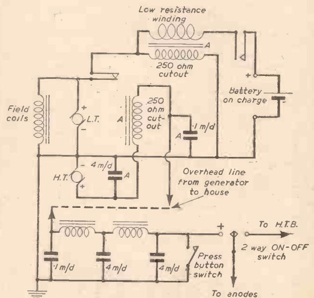
Fig. 5.—Circuit diagram of electrical connections.
