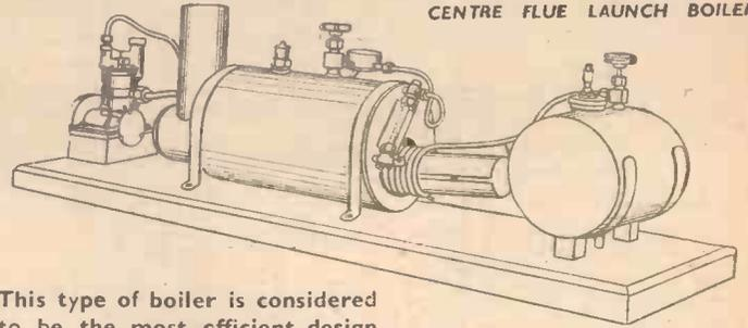
This type of boiler is considered to be the most efficient design for power boats. It is made of solid drawn copper tube, is brazed throughout and every unit is tested to 150 lbs. pressure.
