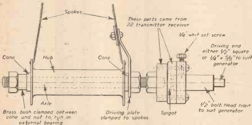
Fig. 1.—Details of the coupling between the wheel hub and the generator shaft.
