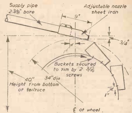
Fig. 4.—Showing the position of discharge nozzle in relation to buckets.
