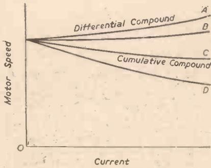
Fig. 18.—Characteristics of compound motors.
