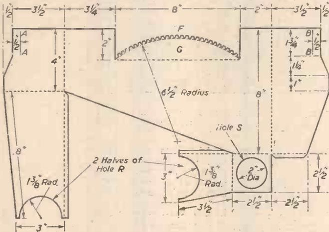
Fig. 1.—Shape and dimensions of tinfoil blank for forming the heater casing.
