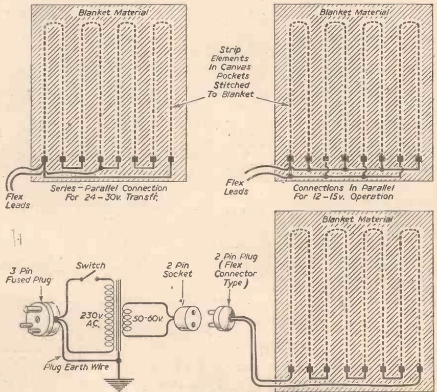
Diagram showing arrangement of elements, and connections to transformer.
