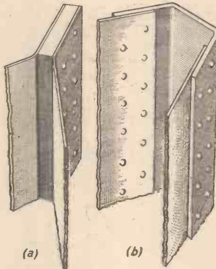
Fig. 21.—Methods of forming the stem.
