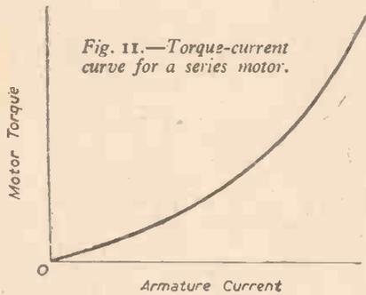
Fig. 11.—Torque-current curve for a series motor.
