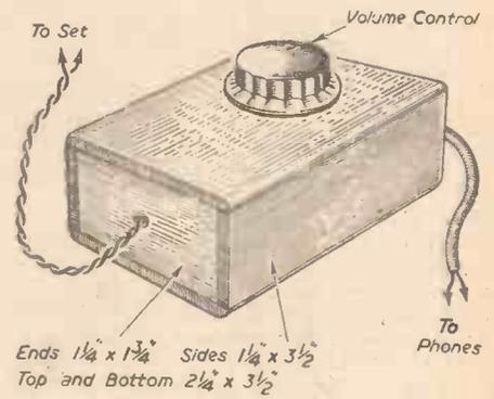
Fig. 3.—View of the completed unit giving dimensions for the casing.
