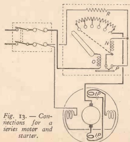
Fig. 13.—Connections for a series motor and starter.
