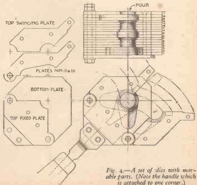
Fig. 4.—A set of dies with movable parts. (Note the handle which is attached to one corner.)
