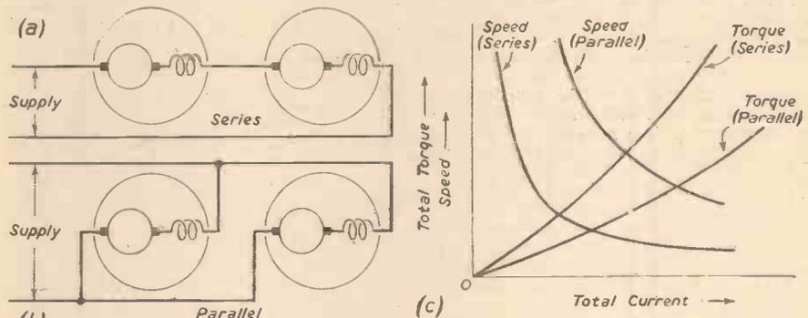
Fig. 17.—Series-parallel control of two series motors.
