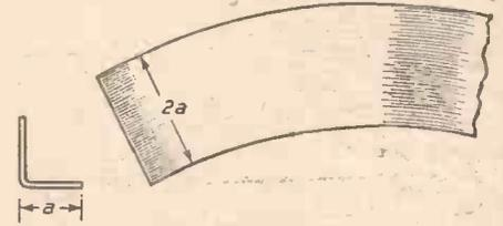
Fig. 28.—Showing how the chine plate is cut into curved strips.
