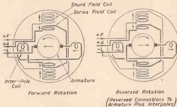
Fig. 19.—Method of reversing a compound motor.
