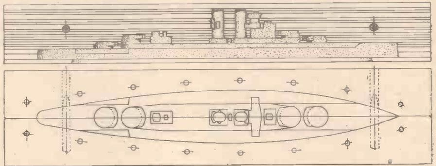
Fig. 1.—Dies for casting models of a battle-cruiser.
