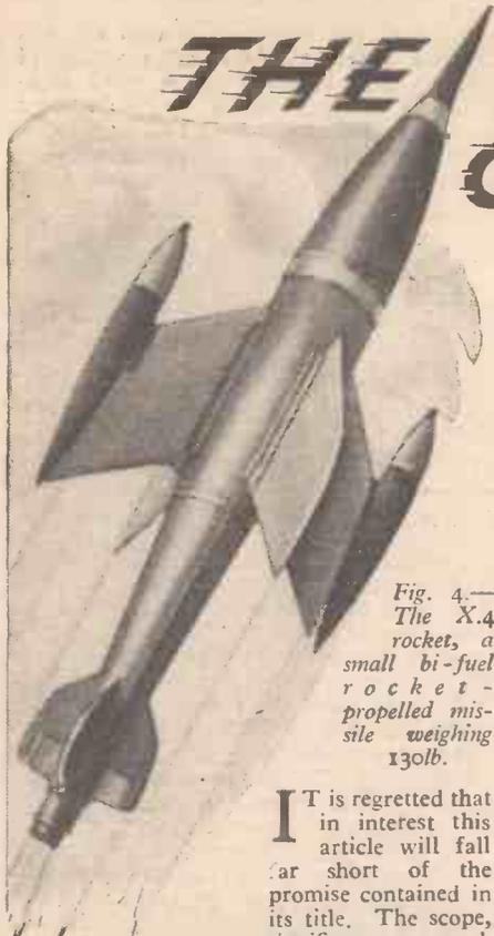
Fig. 4.—The X.4 rocket, a small bi-fuel rocket-propelled missile weighing 130lb.
