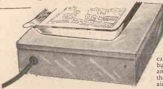
four holes in the base to take the rubber feet fixing screws and one for the cable entry in the side. The cable entry hole should have a rubber bush of the type used in radio sets and the cable should be a tight fit in the bush in order to keep the case airtight.
