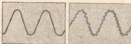
Fig. 2.—A single fundamental tone and the effect of harmonics.
