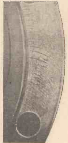
Fig. 3.—Crazy cracks on a ground ring.
