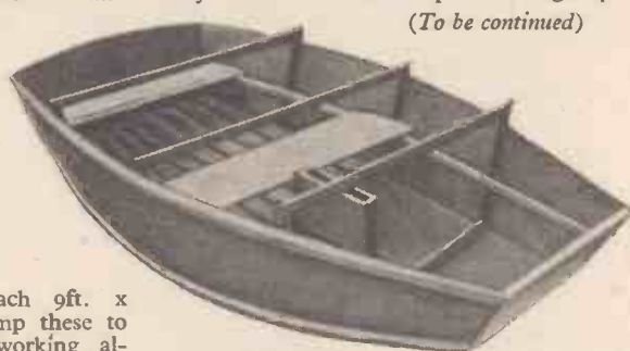
Fig. 14.—The hull after being removed from the form and three bracing strips replaced.
