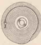
Fig. 35 (left).—On the left, a flat hairspring. Centre and right, a Breguet hairspring in end and plan view showing the overcoil.
