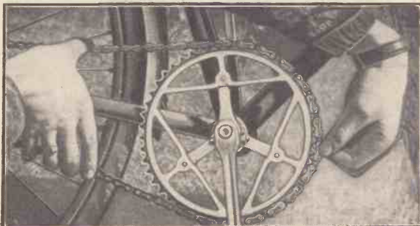
Fig. 2.—Testing for chain wear by holding top and bottom together and lifting away from chainring
