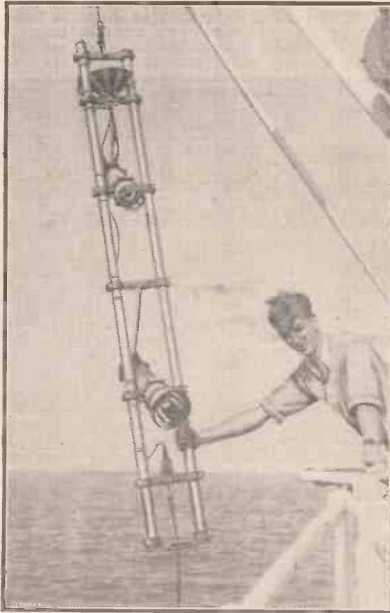
Fig. 3.—A deep-sea underwater camera.
