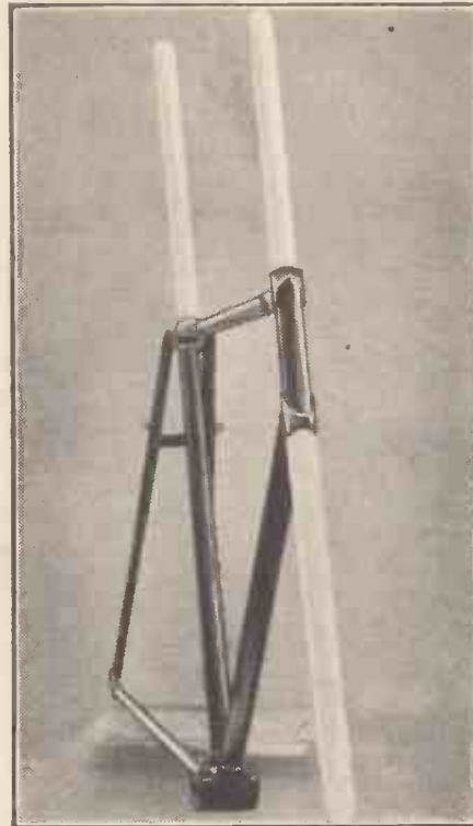
Fig. 3.—Checking head and seat tube alignment.
