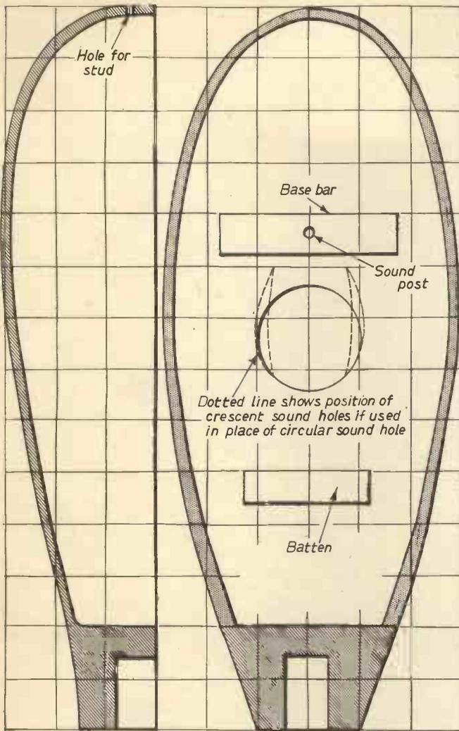
Fig. 3.—Plan of the body. The squares each represent 1 in. full size
