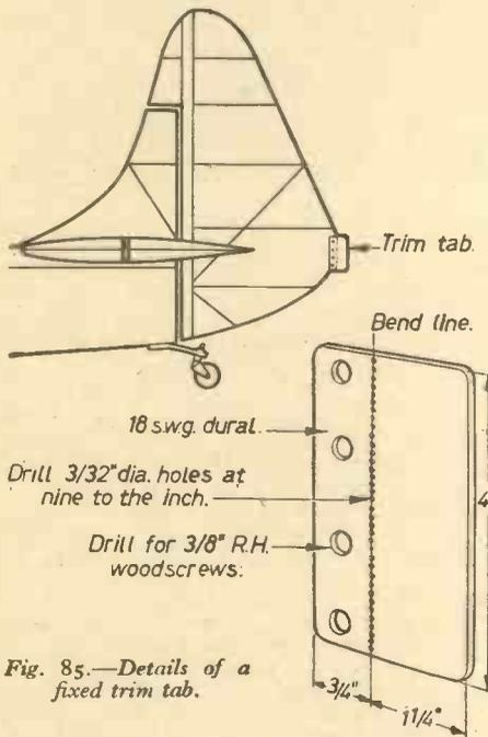
Fig. 85.—Details of a fixed trim tab.
