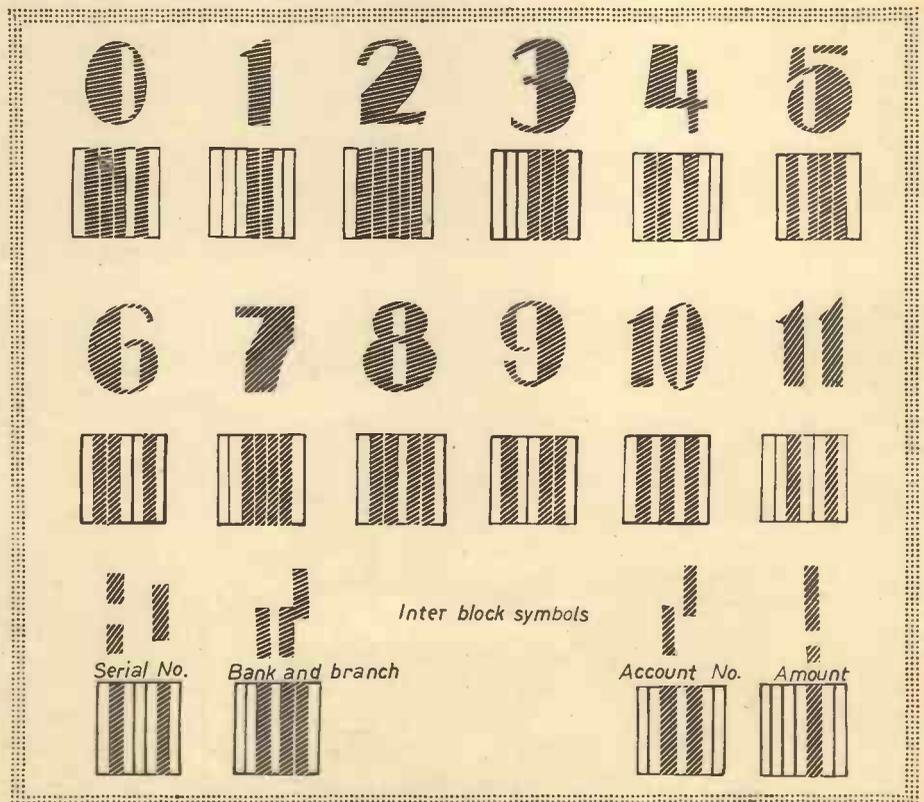
A five-element bar code has been built into the design of the numerals.
