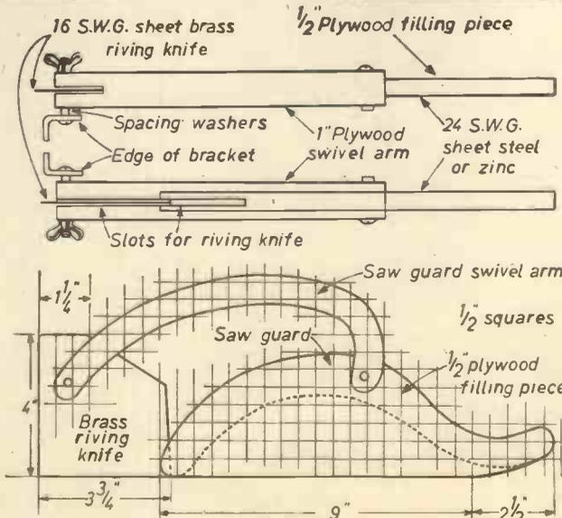
Fig. 5.—Saw guard and riving knife. (Top) View looking down. (Centre) Underside view. (Bottom) Side view. The curved dotted line shows how plywood filling between the two pieces of sheet zinc is cut away to clear the saw.
