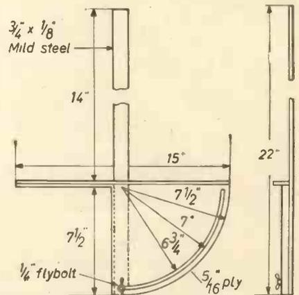
Fig. 7.—Plan and side elevation of mitre gauge.
