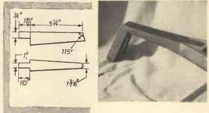
Fig. 5.—Dimensions of the neck and photograph of the neck and head temporarily fixed to the body.
