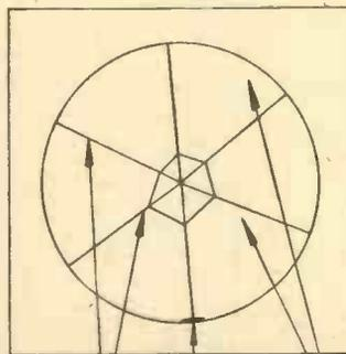
Fig. 6.—Cutting a large hole, shown diagrammatically.
