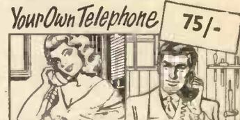
**Telephone Set Type "A".** Ringing and speaking both ways on a 4-core cable. Carries the voice loudly and clearly over any distance. Two hand-sets are supplied as illustrated and the set is complete with Pushes, Buzzers, Battery, Plugs and Sockets. 4-core PVC cable 10d. yd. 75/- set, post 3/6. Set Type "B". Speaking only 38/9, post 3/6. Use twin wire 3d. yd.
