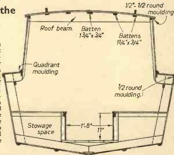
members at frames 2, 3 and 4 and cut out a notch upon which the beams can rest (Fig. 28). Screw the beams into position.
