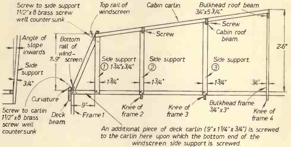
Fig. 29.—Details of cabin side structures.
