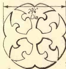
Fig. 12 (left).—The sound-hole inlay.
