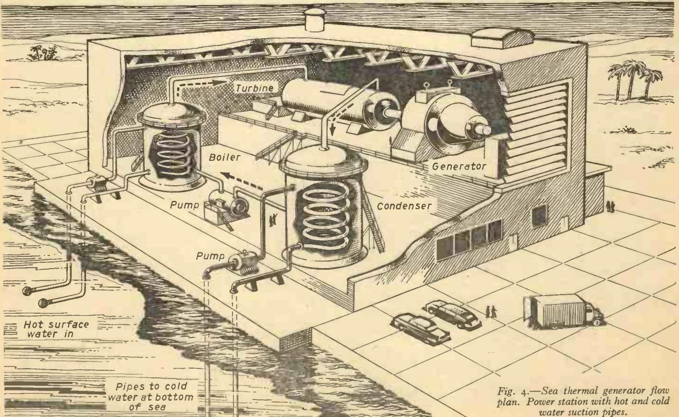
Fig. 4.—Sea thermal generator flow plan. Power station with hot and cold water suction pipes.
