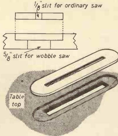
Fig. 2.—Details of inset for accommodating wobble saw.
