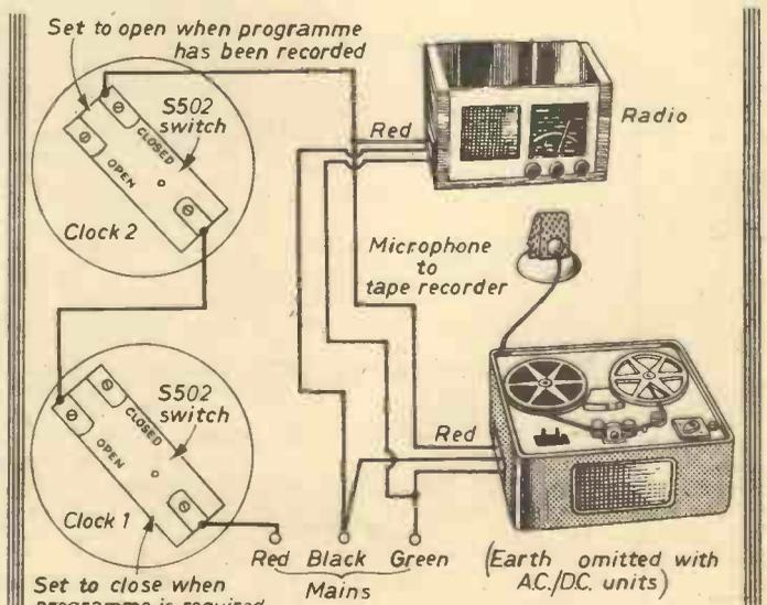
Fig. 45.—Using two home-made micro time switches to record a radio programme.
