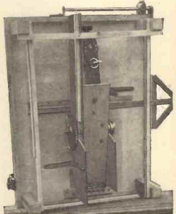
Fig. 4 (Right).—A further underside view showing the whole of the rise and fall mechanism.
