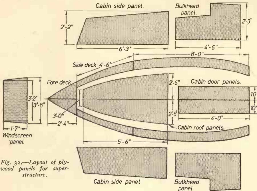
Fig. 32.—Layout of plywood panels for superstructure.
