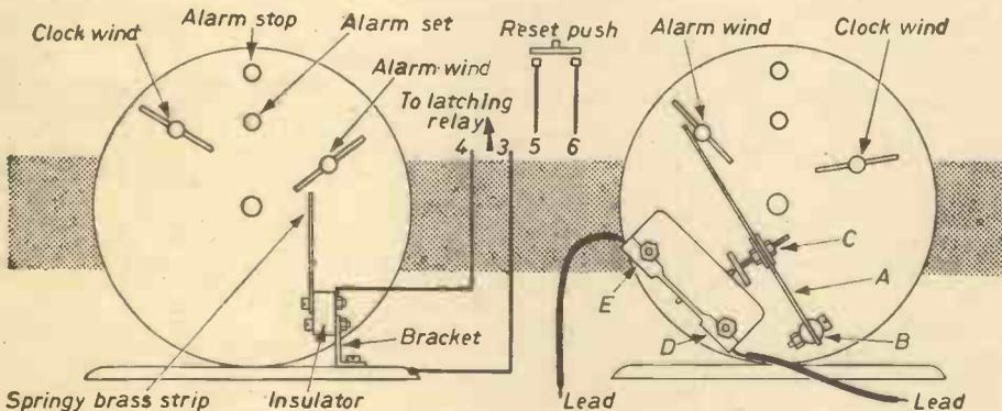
Fig. 43.—Simple alarm clock time switch.
