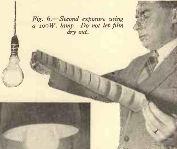
Fig. 6.—Second exposure using a 100W. lamp. Do not let film dry out.
