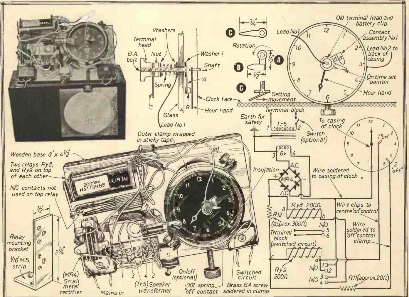
Fig. 51.—Main dimensions of the relay mounting bracket.
