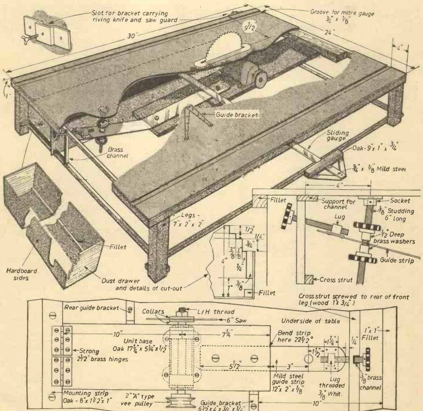
Fig. 1.—General arrangement and plan views of the saw table and insets showing sawdust drawer and adjustment controls.
