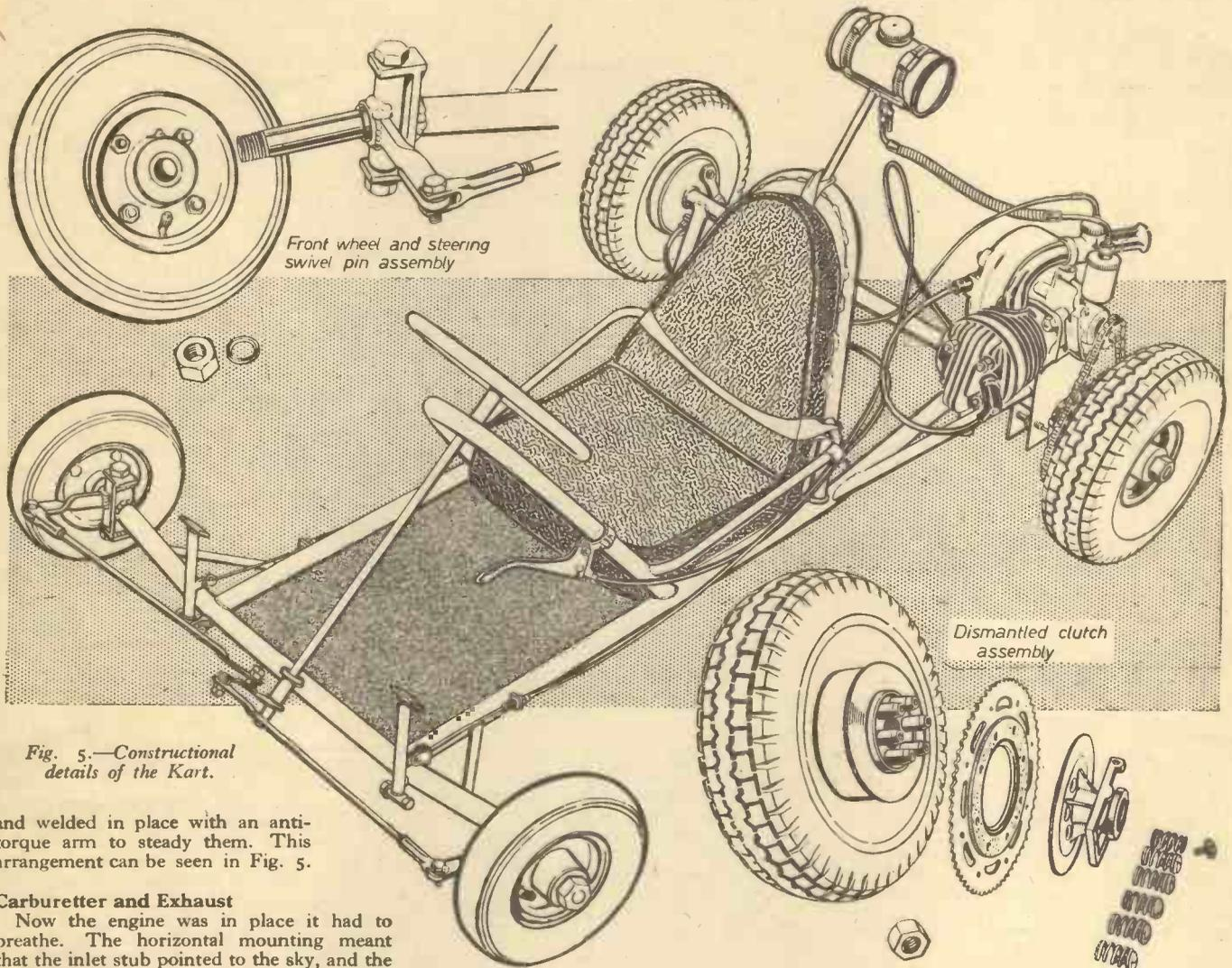
Fig. 5.—Constructional details of the Kart.
