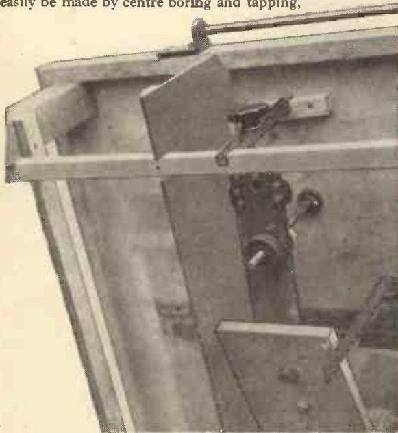
Fig. 3 (Left).—An underside view of the saw table showing particularly the adjustment mechanism.
