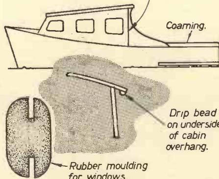
Fig. 35.—Cockpit side screen and rubber moulding for windows.
