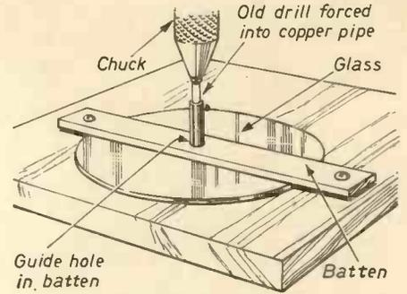
Fig. 48.—Drilling the glass.
