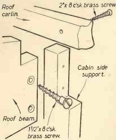
Fig. 28.—Details of junction of roof beam, roof carlins, and cabin side supports.
