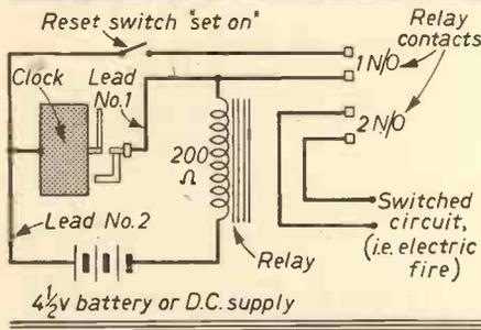
Fig. 47 (Above).—Wiring for "on" only.
