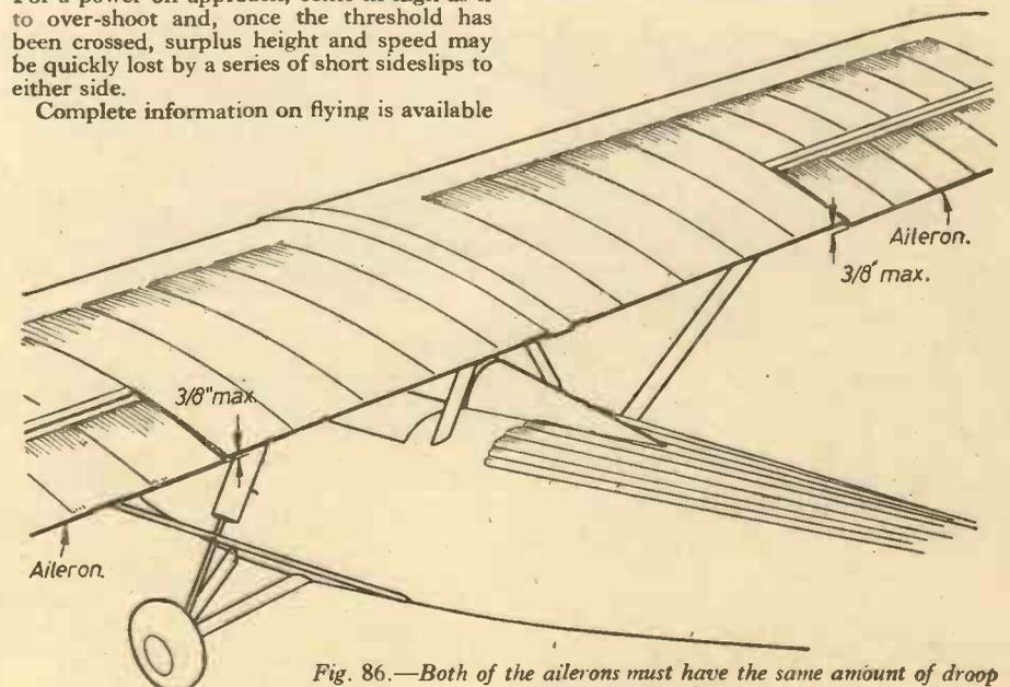
Fig. 86.—Both of the ailerons must have the same amount of droop with the control column central.
