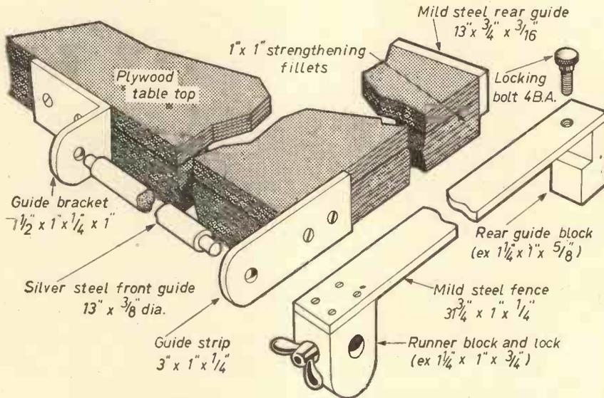
Fig. 6.—Details of the fence. Wooden parts are shown shaded.
