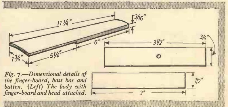
Fig. 7.—Dimensional details of the finger-board, bass bar and batten. (Left) The body with finger-board and head attached.
