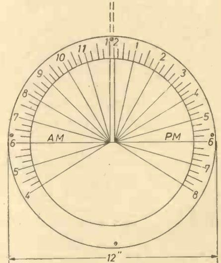
Fig. 5.—The completed sundial. The words "Add 7 min. for apparent time at Greenwich" should be engraved on the dial.
