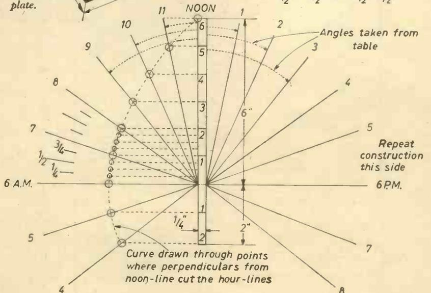
Fig. 4.—The method used for subdividing the hours into quarters, etc.
