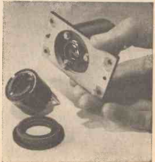
Lens mount, lens, heater and front cover glass.
