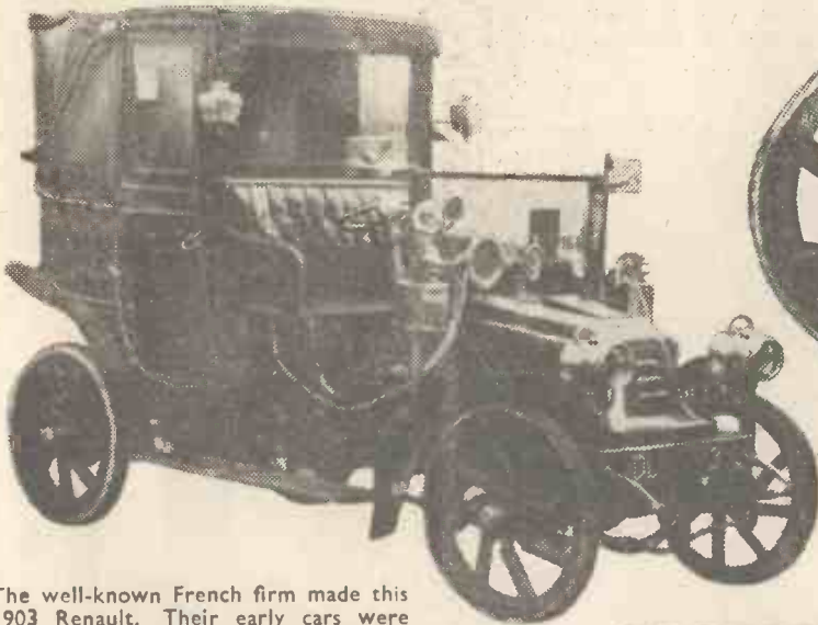
The wheels of this Renault had hydraulic spokes. This must have been the earliest type of independent suspension on all four wheels.
