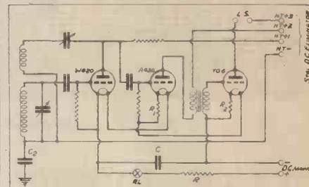
lead must be removed from earth terminal and a fixed condenser (say, 0.05 MF.) connected between earth and receiver.
