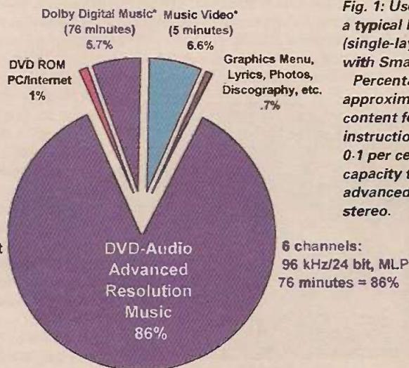
Fig. 1: Use proportions of a typical DVD-Audio disc (single-layer, one-sided with Smart content). Percentages are approximate. Smart content fold-down instructions use less than 0.1 per cent of disc capacity to deliver advanced resolution stereo.
