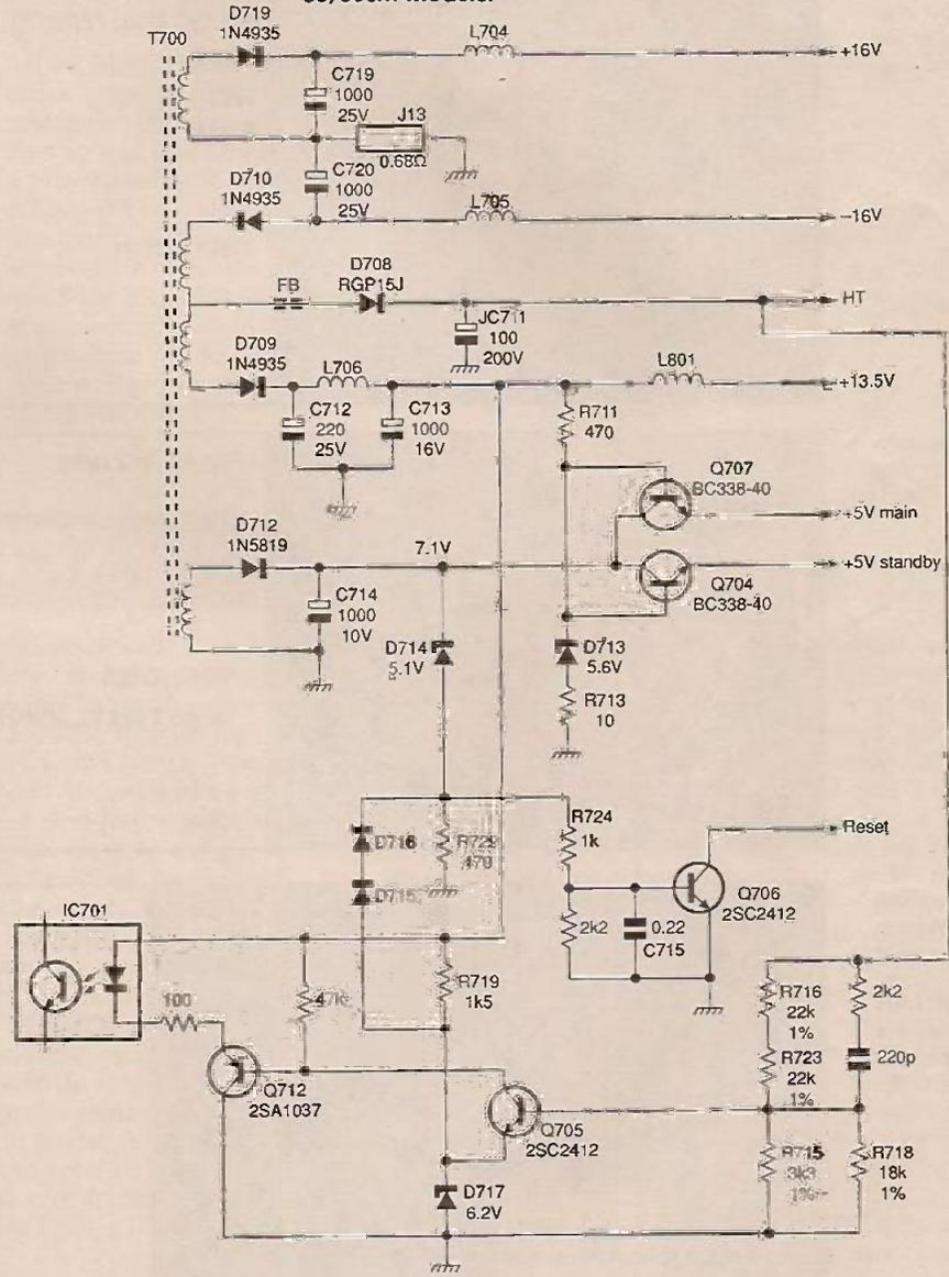
standby. If Q707 is faulty it's a good idea to replace C714 as well, even if it has been replaced before. Q706 provides the reset pulse at pin 10 of the microcontroller chip IC1001. It's controlled by the
