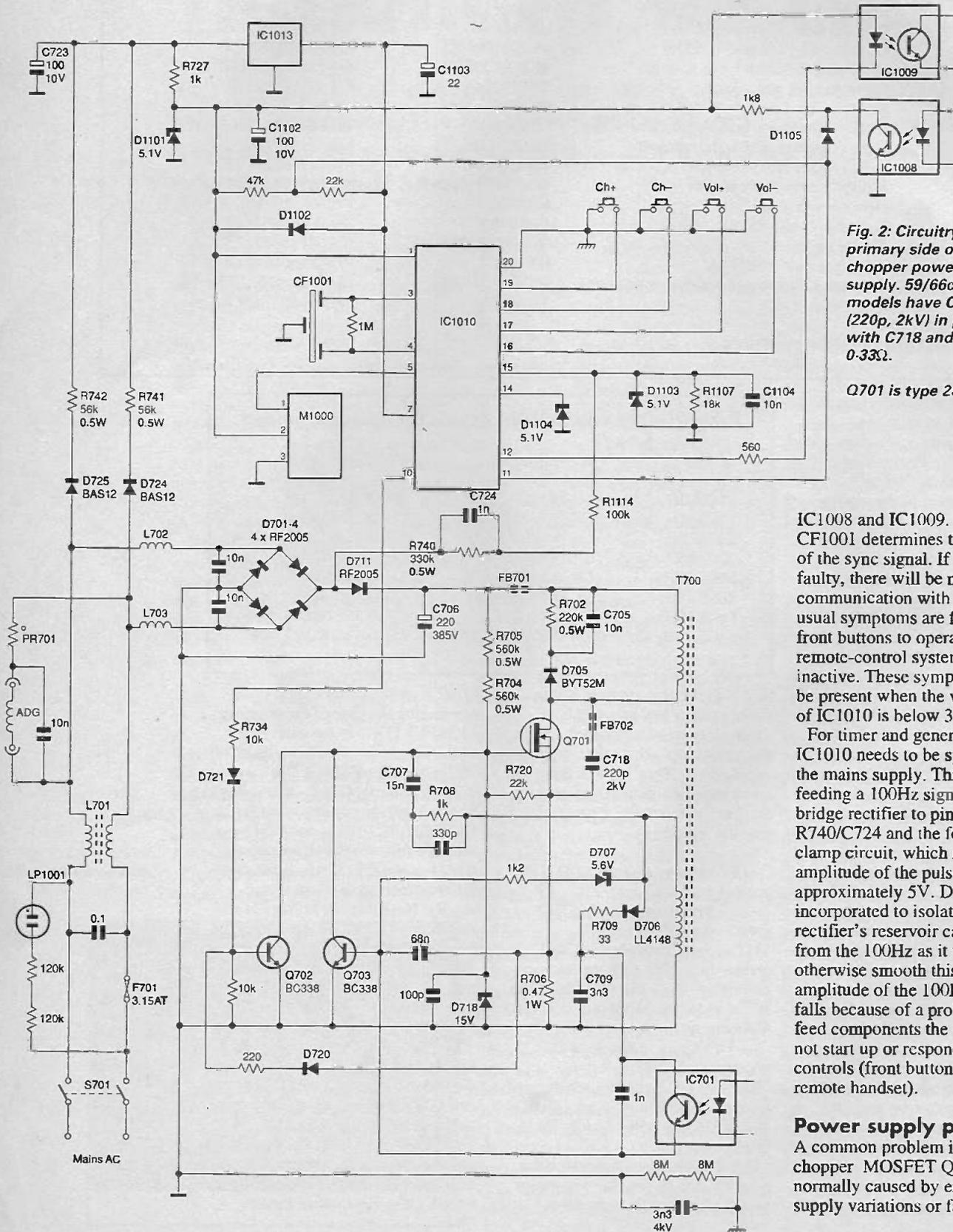
Fig. 2: Circuitry on the primary side of the chopper power supply. 59/66cm models have C733 (220p, 2kV) in parallel with C718 and R706 is 0.33Ω.
