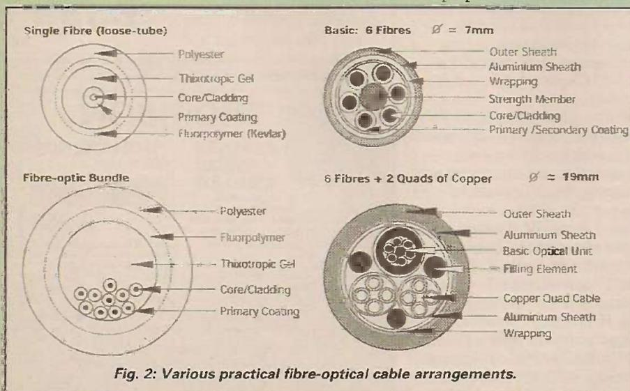
Fig. 2: Various practical fibre-optic cable arrangements.
