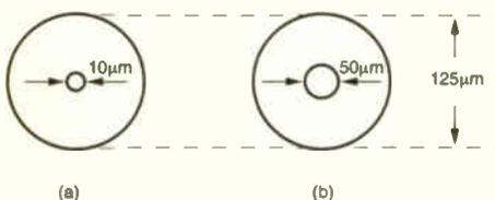
**Fig. 1: The two basic types of fibre, (a) single-mode and (b) multi-mode.**
