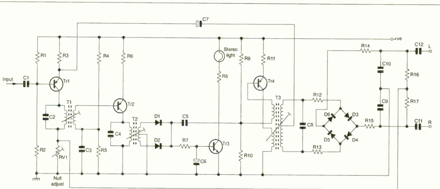
Fig. 2: Typical early stereo decoder circuit, simplified.
