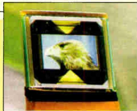
*Philips Research has demonstrated this 51cm, 64 x 64 pixel polymer-dispersed LCD screen which could be a significant step towards cheap, flexible displays. It uses a polymer active matrix based on a polythienylenevinylene precursor, which is separated from the polymer-dispersed LCD by spin-coated polyvinylphenol. The LCD is voltage switched and can produce 256 contrast levels. No polariser or alignment layer is required.*
