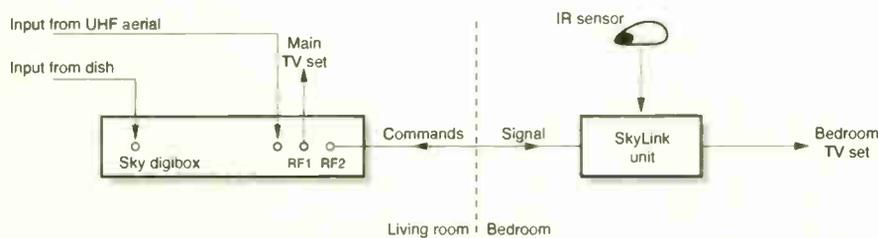
Fig. 1: The basic SkyLink arrangement.
