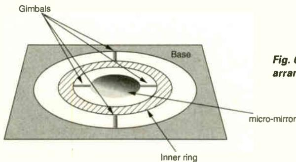
**Fig. 6: Basic MOEMS arrangement.**
