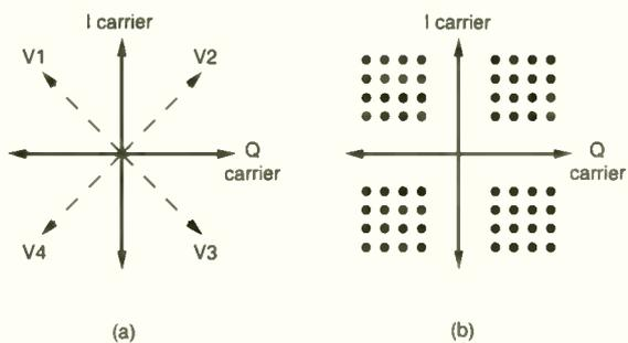
**Fig. 4: QPSK and 64QAM modulation.** (a) With QPSK two carriers, I and Q, can be modulated to produce four vectors (V1-4). The technique can handle four 2-bit codes. (b) 64QAM: each of the 64 dots represents the end point of a vector produced by phase and amplitude modulation of one or both carriers, I and Q.
