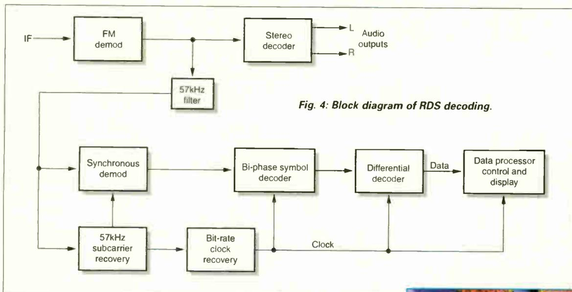
Fig. 4: Block diagram of RDS decoding.
