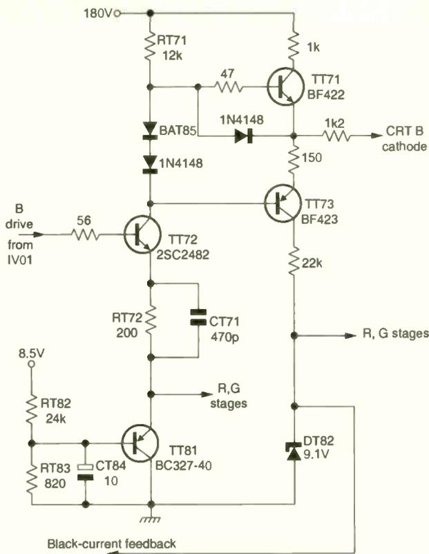
Fig. 7: RGB output stage circuitry, ten-transistor version.
