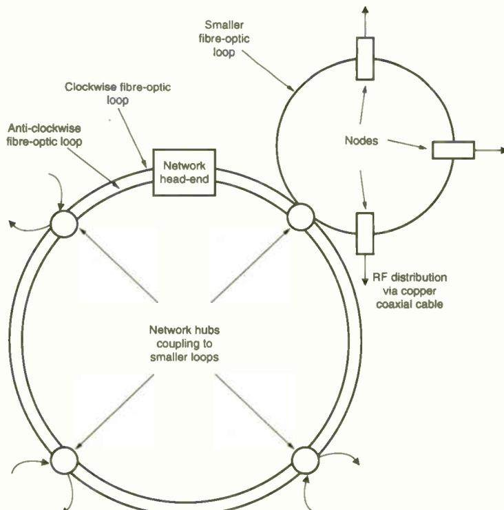
Fig. 3: Distribution network consisting of a primary fibre loop fed from the main head-end, hubs and local distribution nodes.
