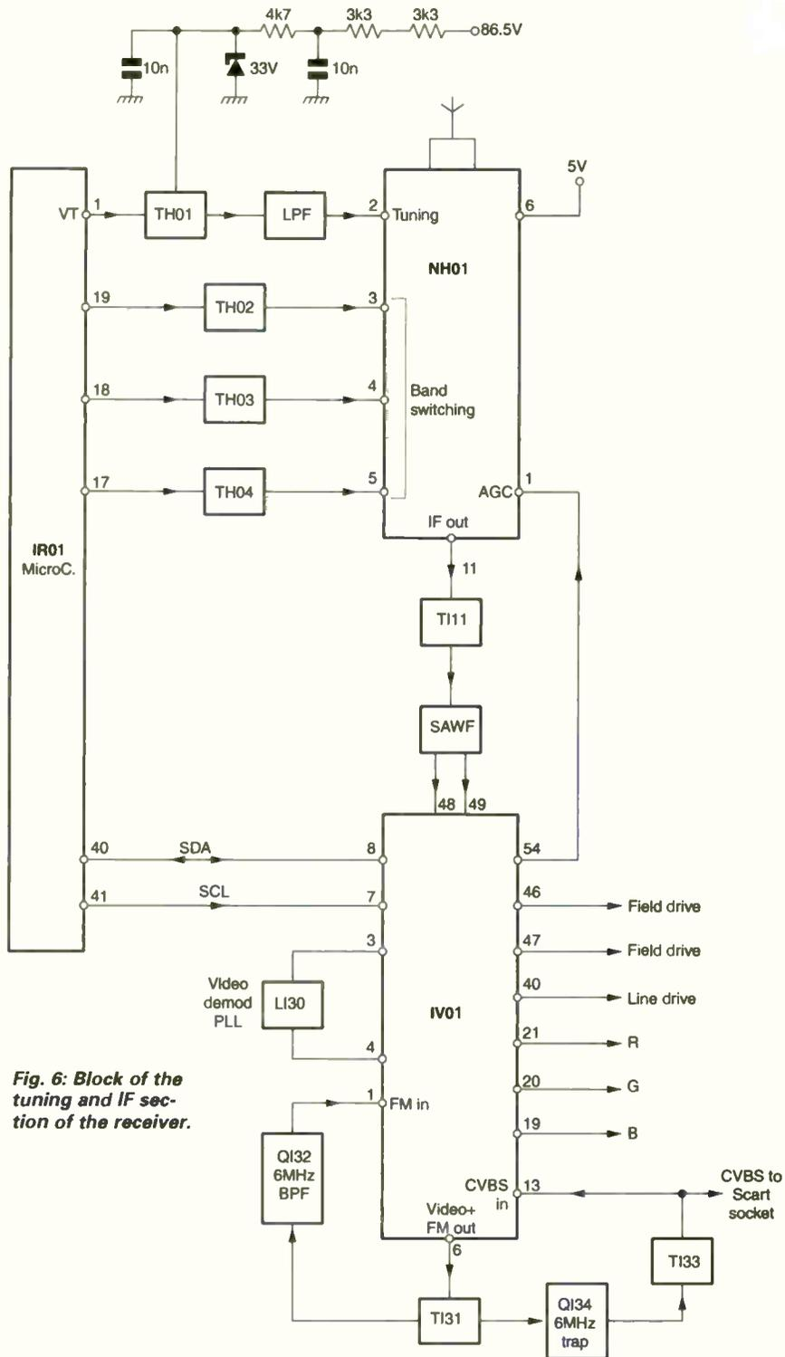
Fig. 6: Block of the tuning and IF section of the receiver.
