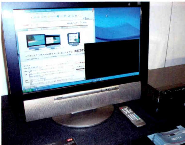
**Sharp's IT-TV, which is an LCD multimedia monitor with a built-in tuner and the ability to display graphics from a PC.**
