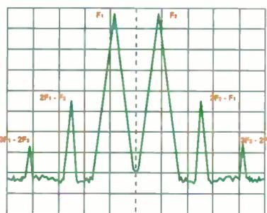
Figure 2: Two tone intermodulation analysis
