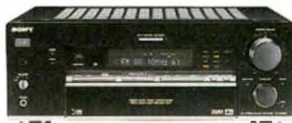
On this unit, A clicking noise could be heard just before the unit would switch off (intermittently). A look inside the unit using the (bottom) service plate, on the Main Amp PWB revealed the fault to be dry joints on both audio output relays (RY601) and (RY701) and all that was needed to restore the intermittent fault was to re-solder the relays.
