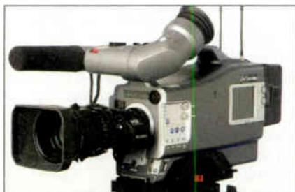
*Infinity camcorder features 14-bit digital imaging*
