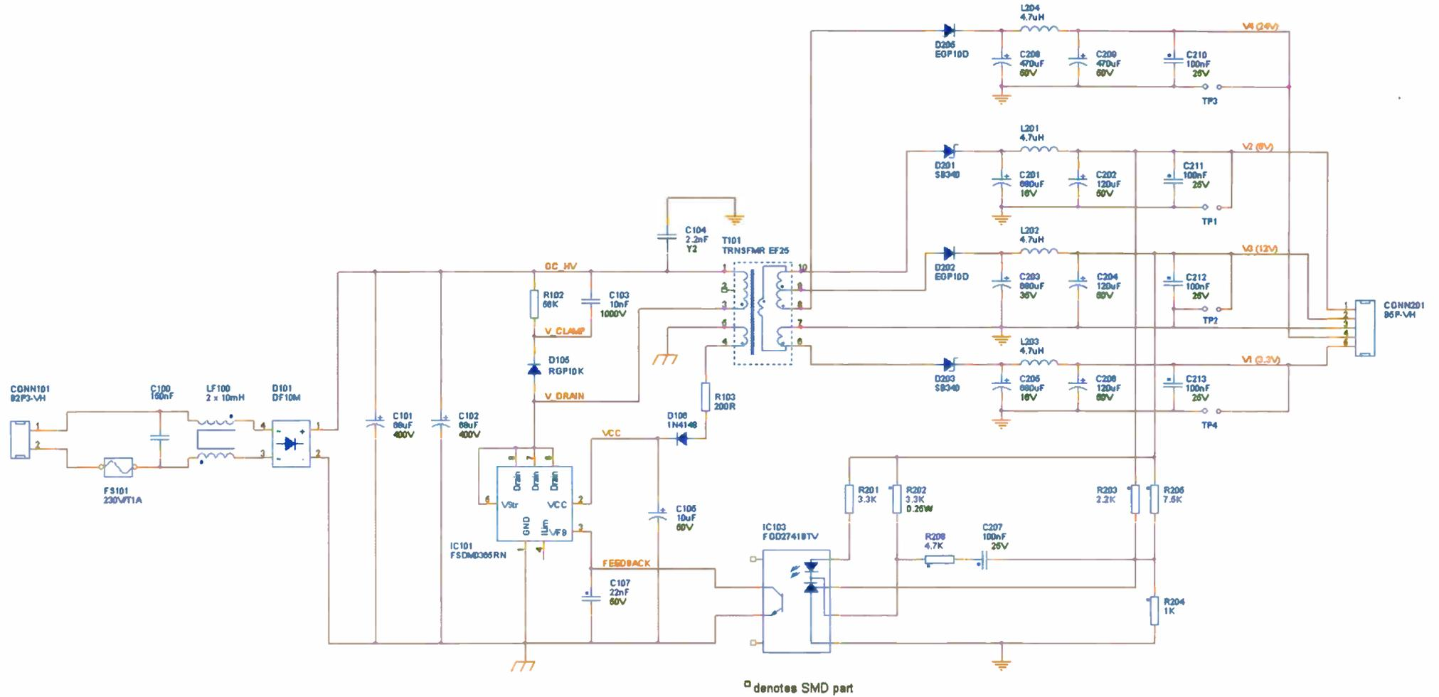
Sense FET with a current mode PWM control block.
