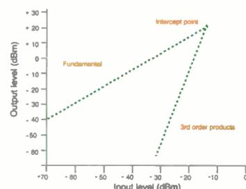
Figure 3: Intermodulation intercept point
