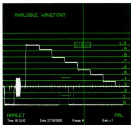
Figure 1: Luminance waveform display
