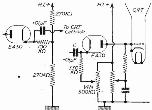
Fig. 13 (left).—Modification of Fig. 12. Fig. 14 (right).—Diode gate fitted to the Lynx.
