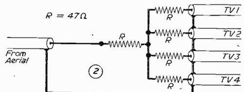
Fig. 2.—In this scheme four receivers may be fed from a single aerial.
