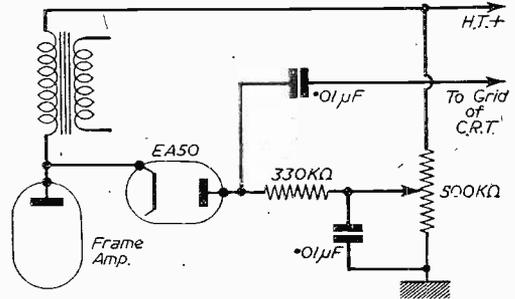
Fig. 16.—Directly-coupled gate.
