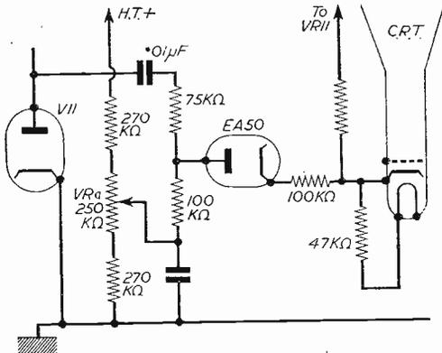
Fig. 12.—Details of the "Simplex" with diode gate.
