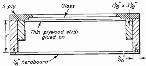
Fig. 2.—Section through case.
