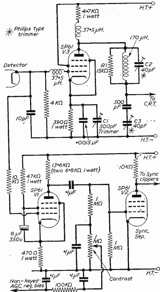
Fig. 1(b).—Theoretical circuits of the Fig. 1(a) scheme.
