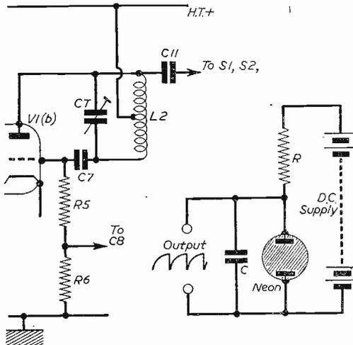
Fig. 2 (left).—Alternative 81 kc/s oscillator circuit if centre-tapped coil is available. C1=250 pF trimmer. R4, C5 and C6 are not required. Fig. 3 (right).—Basic circuit of a neon relaxation oscillator. The D.C. supply charges C through R until the potential of C is sufficient to cause the neon to strike. On striking, the neon discharges C and the cycle is repeated.
