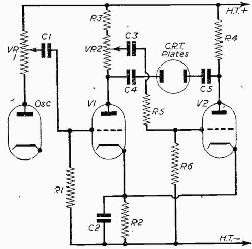
Fig. 14.—A dual amplifier (frame)
