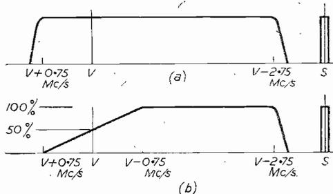
Fig. 7.—Showing (a) a vestigial-sideband transmission; and (b) the correct receiver alignment curve.
