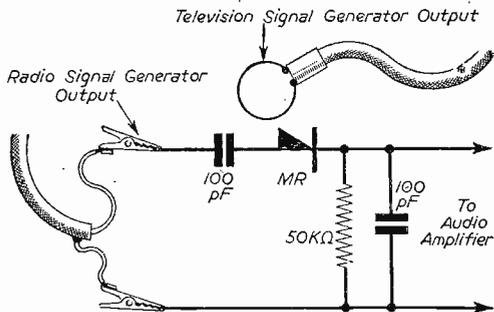
Fig. 6.—Circuit used for beating the outputs of two generators together.
