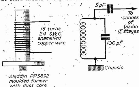
Fig. 3.—Suitable retractor for use with ex-Government I.F. strips.
