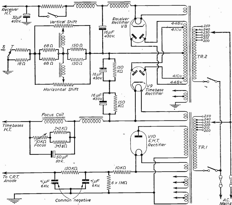
Fig. 5.—H.T. and heater supply. TR1 is disconnected on radio.
