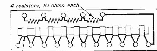
10 coils, 1 ohm each (27" of 40 s.w.g. copper wire wound on bakelite tube)
