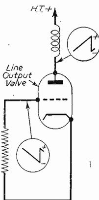
Fig. 16.—Waveform at grid and anode.
