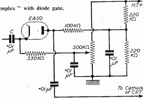
Fig. 15.—Diode with separate potential divider.
