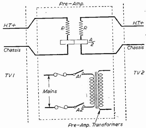
Fig. 5.—Using a mains-operated relay for switching on and off.
