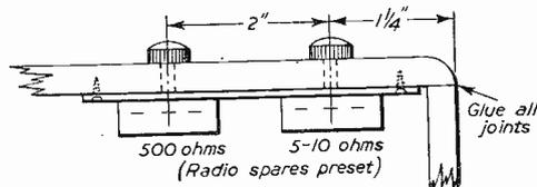
Fig. 4.—Corner of case showing potentiometers.
