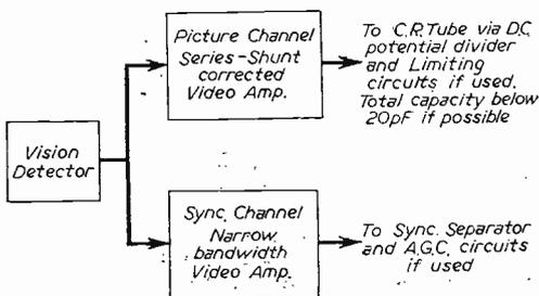
Fig. 1(a).—Block diagram of picture and sync channels.
