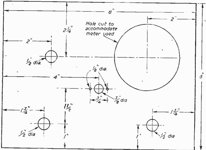
Fig. 4.—Front panel drilling.
