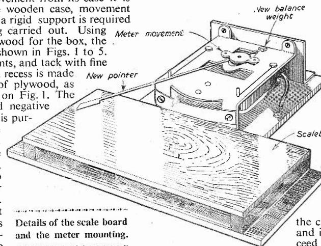
Details of the scale board and the meter mounting.
