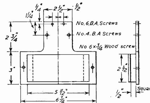
Fig. 3.—Details of the 5-ply support and scale board.
