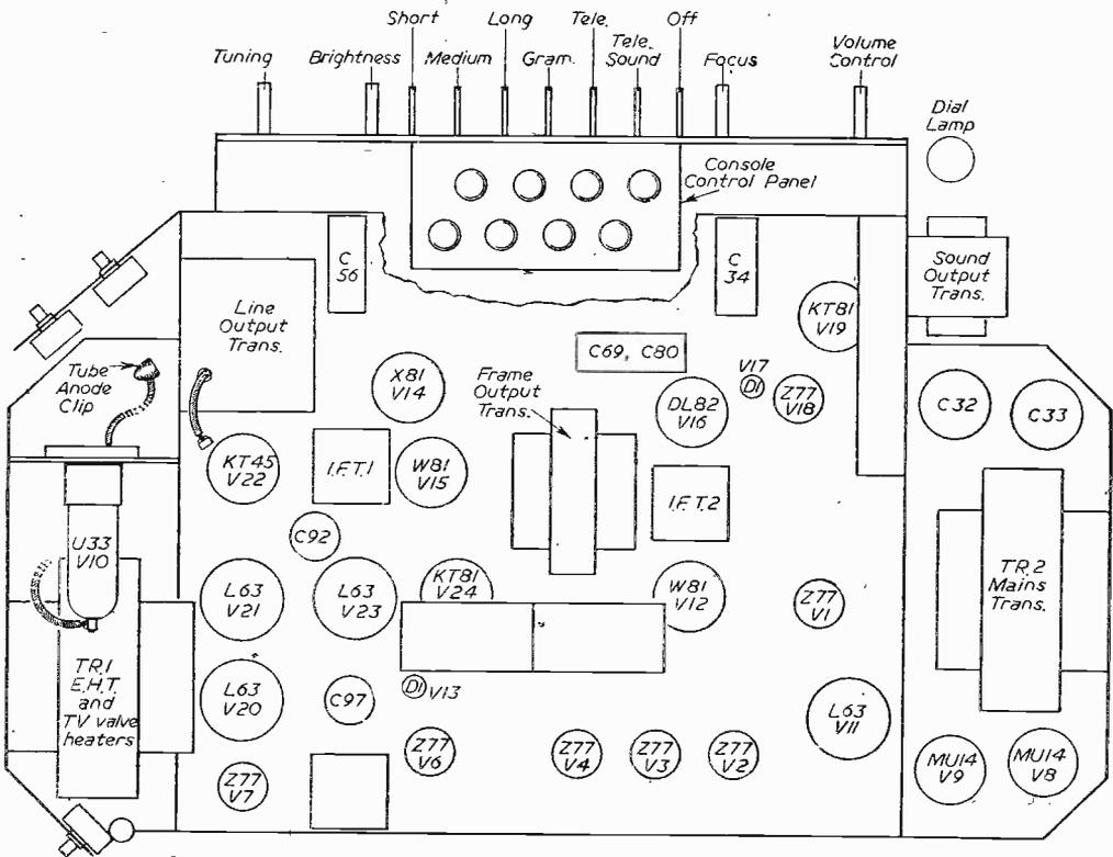
Fig. 4.—Top chassis view of table model. The side transformer "wings" are combined to form a power pack on the console version. The panel marked "Console control panel" is only mounted on the Console and is actually located under the P.B. selector unit. The positions of C92, C97 and C33 should be noted.
