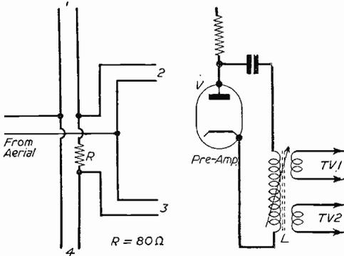
Fig. 3 (left).—Using a balanced twin feeder. Fig. 4 (right).—Splitting the output of a pre-amplifier.
