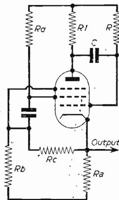
Fig. 17.—Producing a positive scan.
