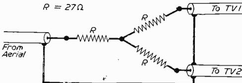
Fig. 1.—A simple method of providing two channels from one aerial.
