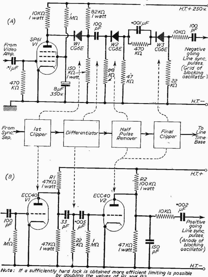
Note: If a sufficiently hard lock is obtained more efficient limiting is possible by doubling the values of R1 and R2
