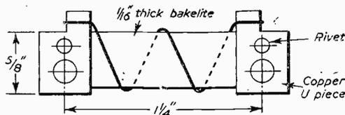
Fig. 10.—Details of the shunts.
