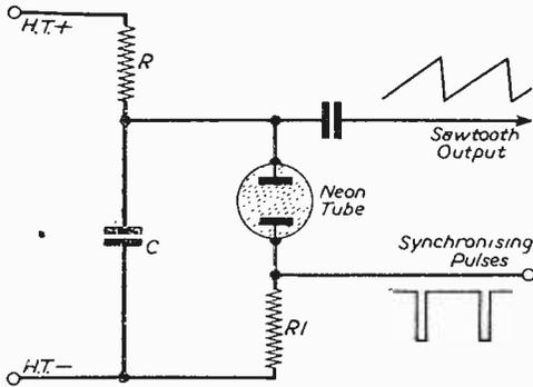
Fig. 10.—Simple neon-tube timebase.
