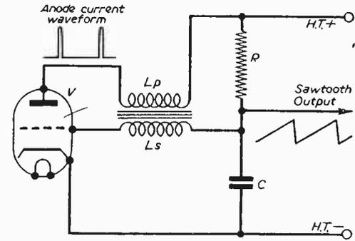
Fig. 12.—Blocking oscillator—simplified circuit diagram.
