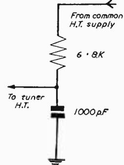
Fig. 4.—Circuit of an H.T. filter.
