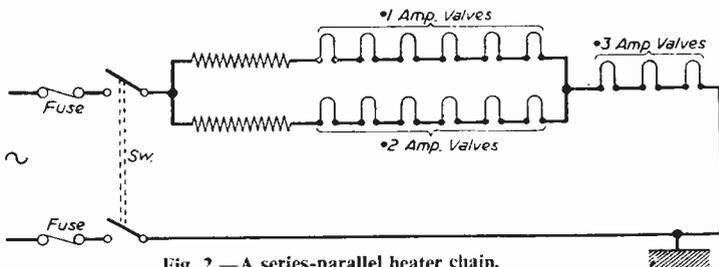
Fig. 2.—A series-parallel heater chain.
