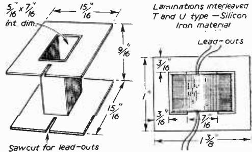
Fig. 15.—Transformer constructional details.
