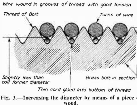
Fig. 3.—Increasing the diameter by means of a piece of wood.
