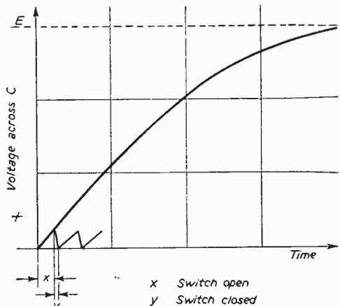
Fig. 9.—Graph showing variation of voltage across C with time.
