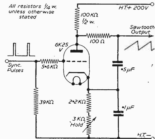
Fig. 11.—Thyratron timebase (for frame scanning).
