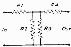
Fig. 3.—A simple "Pi" attenuator for reducing the gain where overloading takes place.
