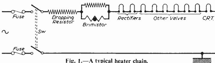
Fig. 1.—A typical heater chain.
