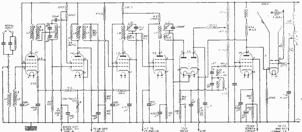
Fig. 1.—The vision strip showing H.T. supplies and biasing arrangements. Note: The aerial input capacitor and shunt resistor should connect to chassis, i.e. bottom of L1, not top as shown.
