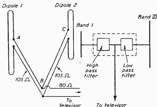
Fig. 5.—This diagram shows the method of connecting two folded dipoles.
