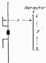
Fig. 2.—Adding a reflector.
