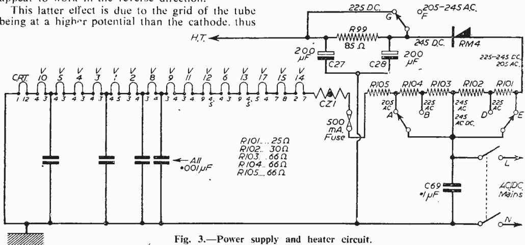
Fig. 3.—Power supply and heater circuit.
