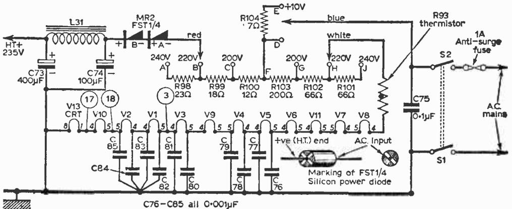
Fig. 1—The power circuit and heater chain, and the end markings of a silicon power diode.
