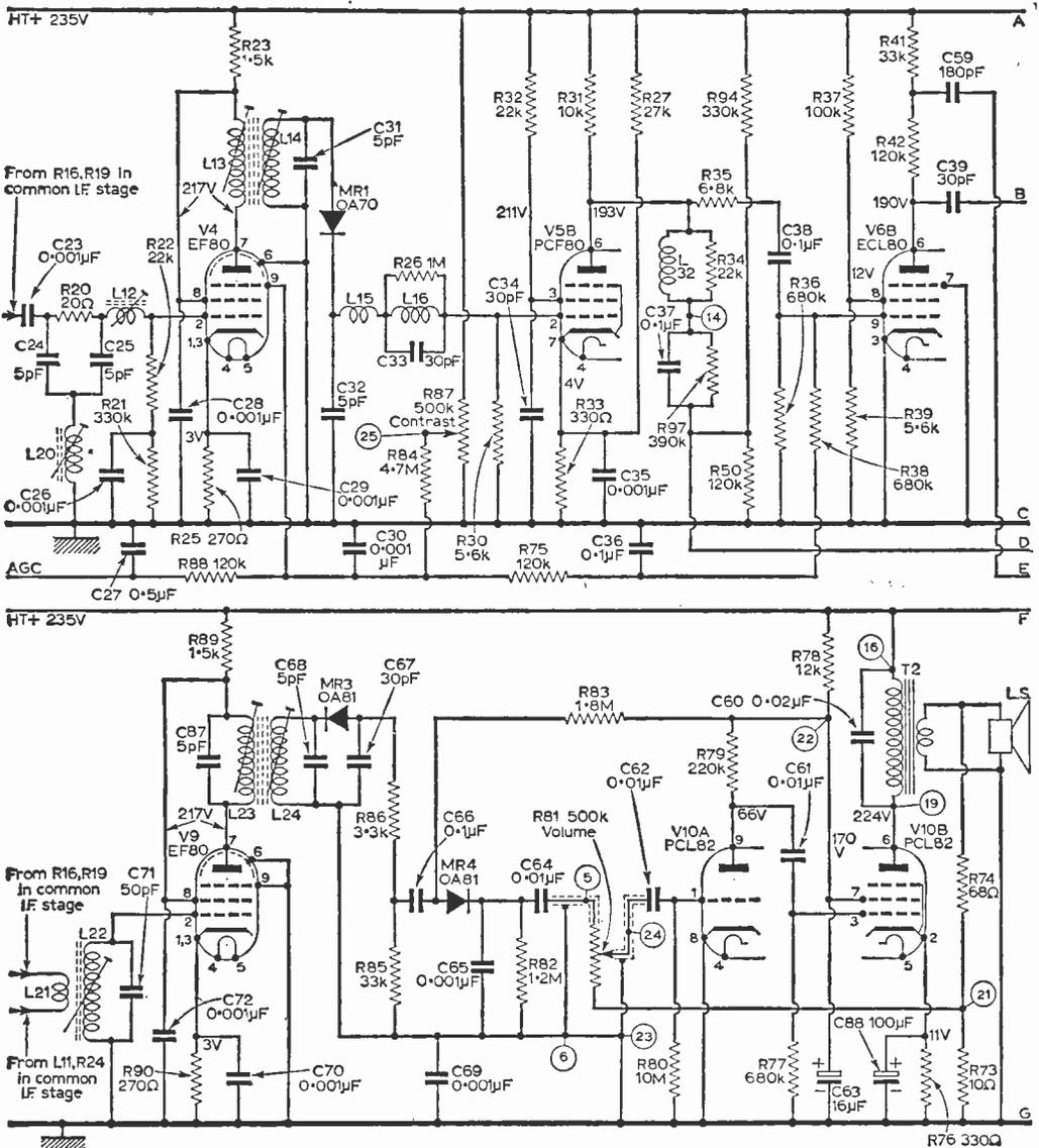
Fig. 2—The vision I.F. and sound stages.
