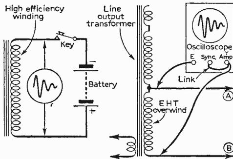
Fig. 18 (left)—Due to the L and C elements in a high efficiency winding, the circuit will tend to produce a damped oscillation when subjected to current pulses. The oscillation will have a frequency equal to the natural frequency of the winding, and the waveform produced is of the type shown.
