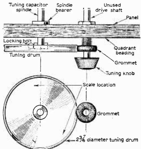
Fig. 5—Details of the tuning mechanism.
