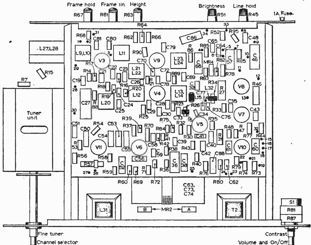
Fig. 3—The underchassis layout of components.
