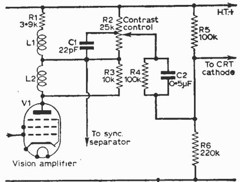
Fig. 9—How the contrast is controlled by varying the actual vision signal level applied to the tube cathode from across the vision amplifier anode load.
