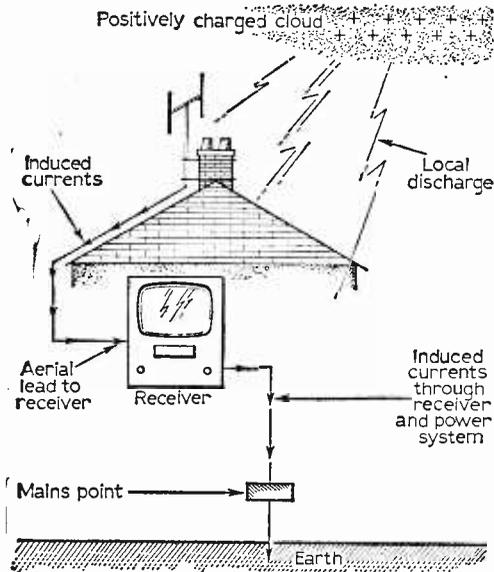
Fig. 4—If the aerial system is inadequately earthed, induced current from a nearby discharge may flow through the set and mains supply, and cause unnecessary damage.
