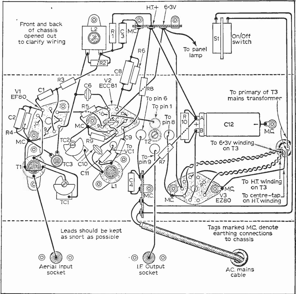
Fig. 6—The underchassis wiring diagram.
