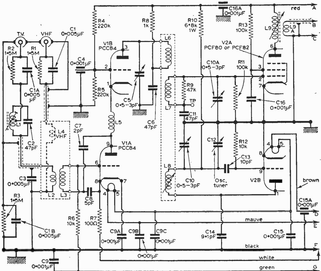
Fig. 1 (a)—The tuner circuit.
