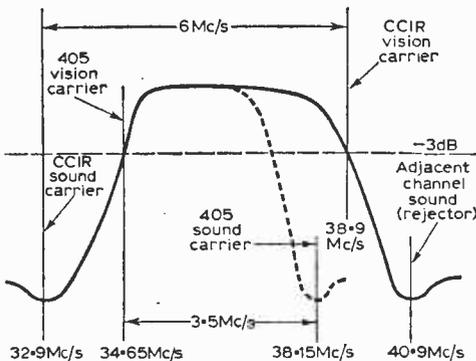
Fig. 8—How the bandwidth of the vision I.F. channel is decreased (dotted line) on 405 lines, and the relative positions of the various carriers. Note the reversal of sound and vision carriers on CCIR.
