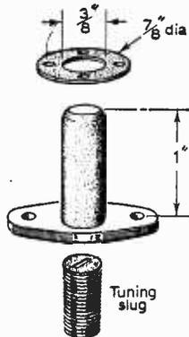
Fig. 4 (right)—The type of coil former used in this unit.
