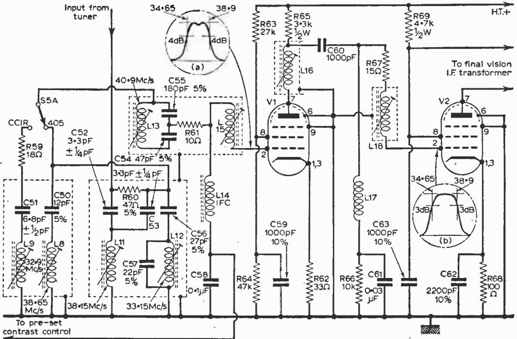
Fig. 7—The vision I.F. stages of a dual-standard receiver (Pye—V700D). The responses in (a) and (b) represent the overall response of the channel, which is reduced in bandwidth by the operation of S5A on 405 lines, as shown in Fig. 8
