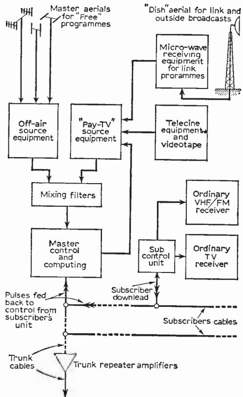
Fig. 1—The basic principles of a “piped” television system handling both “free” and “pay” programmes.
