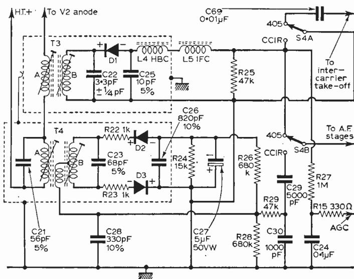
Fig. 6—The sound detector stages; diode D1 and associated components form the A.M. sound detector, while diodes D2 and D3 form the ratio detector for the CCIR F.M.-sound signals.
