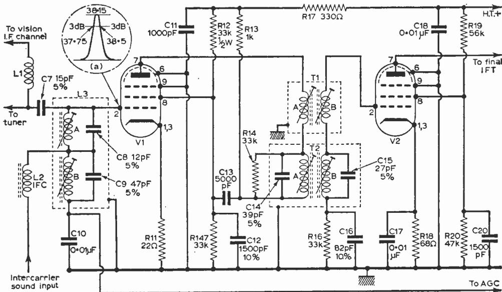
Fig. 5—The sound I.F. channel of a dual-standard receiver. The circuit features series-connected I.F. transformers, one which tunes to the 405-line I.F. (38.15 Mc/s) and the other which tunes to the CCIR inter-carrier I.F. (6 Mc/s).
