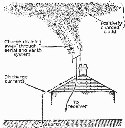
Fig. 3—A television aerial would appear to act as a "lightning conductor", in that it progressively drains away electrical charges in proximity to the house thereby making a local discharge less probable.
