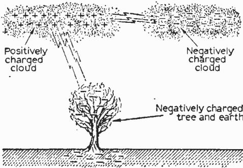
Fig. 1 (above)—A solitary tree, fully exposed on a hill, is an ideal target for lightning. After the main discharge, an adjacent cloud may go negative and give rise to an inter-cloud discharge.
