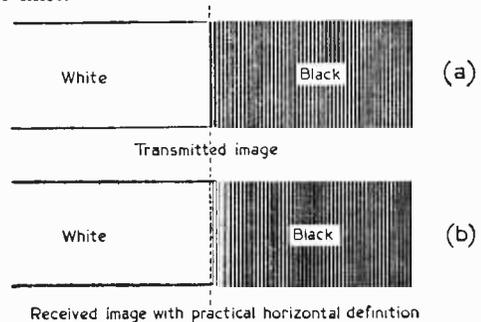
Fig. 1—A sharp shade transition at the camera (a) would be reproduced on a practical system as at (b).
