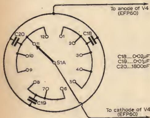
Fig. 2a (above)—Wiring details of S1A.
