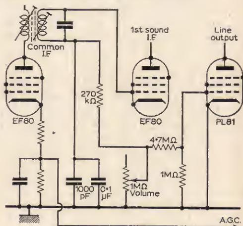
Fig. 17—Alba 988; volume control varies bias applied to sound i.f. amplifier grid. The negative bias voltage is derived from the control grid of the line output valve. Fixed a.g.c. is applied to the cathode of the common i.f. amplifier.
