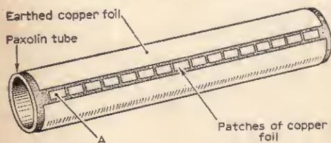
Fig. 5—The completed former of the V4 anode delay line.
