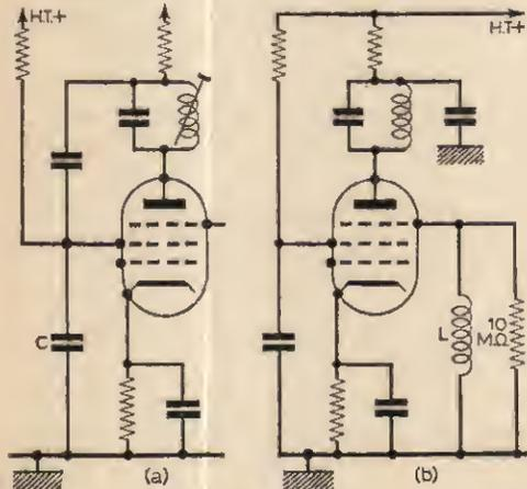
Principal fault with the older models was deterioration of the high value load resistor, or the resistor from h.t. which provided bias. An example is the HMV 1918, where the EB91 has a 3.9MΩ anode load, which can increase to 10MΩ and cause distortion and intermittent sound breakthrough. Loads on TV sound detectors tend to be lower than on radio receivers, with smaller reservoir capacitors, because of the higher frequency i.f.
