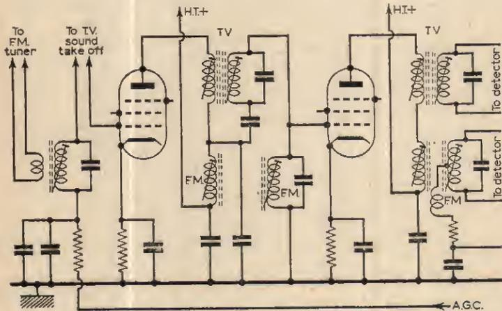
Fig. 12—Sound i.f. stages of a Bush TV77, with supply, etc., components omitted. Separate coils are tuned to the intermediate frequencies, TV 38.15Mc/s, f.m. 10.7Mc/s.
