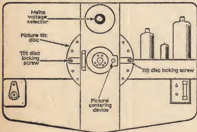
Fig. 1—A rear view of the Murphy V410 receiver showing the layout of the major components.
