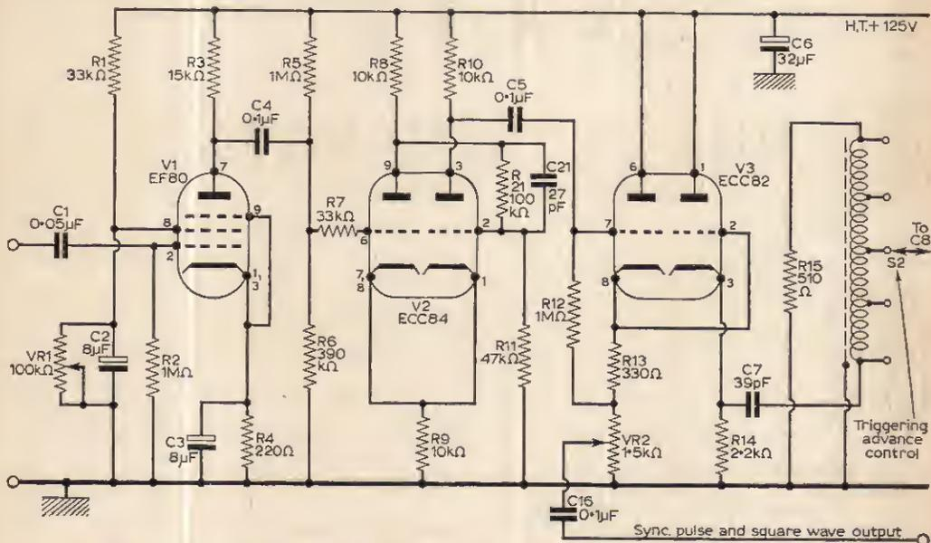
Fig. 1a (above) and b (below)—The circuit. The delay lines referred to in the text connect to the circuit via S1 and S2 and in Fig. 1b these connections are only indicated by arrows.
