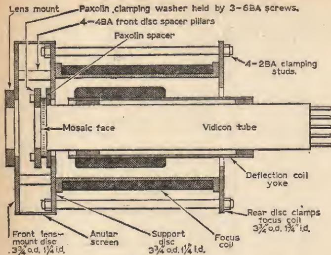
Fig. 4 (above)—A cross-section of the coil assembly.
