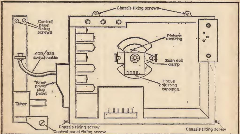
Fig. 4—A V873 series receiver viewed from the rear, showing the component layout.
