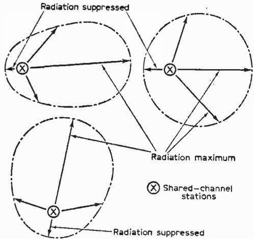
Fig. 3: Directional aerials are used by shared-channel stations to minimise co-channel interference. Added precautions are given by opposed planes of signal polarisation (see text).
