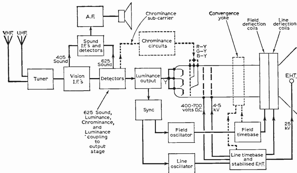
Fig. 27: Simplified block diagram of a colour receiver, omitting dual-standard switching, a.g.c. circuitry, all controls and the grey-scale tracking circuits.
