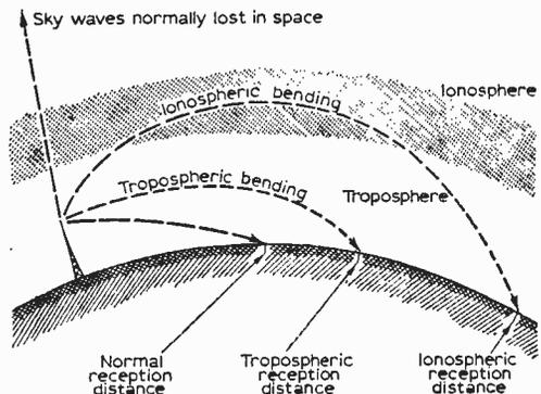
Fig. 4: Showing how TV signals are propagated over greater-than-normal distances due to tropospheric and ionospheric bending.
