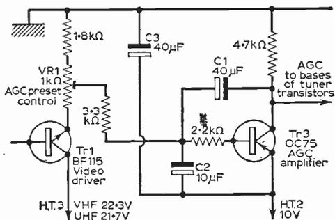
Fig. 9: In the Philips T-Vette the a.g.c. amplifier Tr3 is driven from the first video stage Tr1. Tr1 mean emitter current being dependent on signal strength on both systems, the a.g.c. voltage decreases with rising signal strength to reduce the gain of both r.f. amplifier transistors. Electrolytics C1 and C2 filter out the a.c. component of the video signal and stabilise Tr3.
