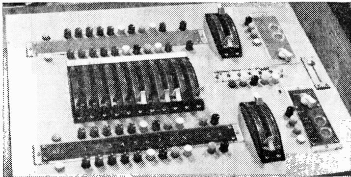
*The ATV network vision mixer: the main cut button selects the remote sources or the three banks, designated red, effects (X), or green. Red and green are the simple mixers described in the text and the effects vision mixer is the fader type. Each bank's output also appears as a source on each other bank, allowing great flexibility of operation.*
