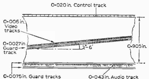
Fig. 4: Track disposition on the video tape with the Ampex helical scan technique.
