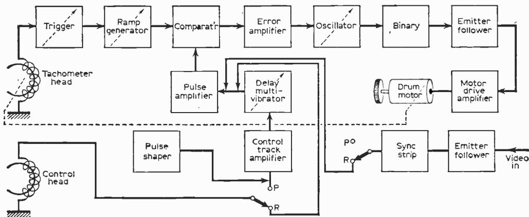
Fig. 6: Block diagram of the servo circuits used in the Ampex VR6000 video tape recorder.
