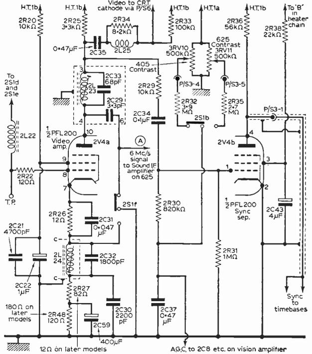
Fig. 7: Video amplifier and sync separator stages.
