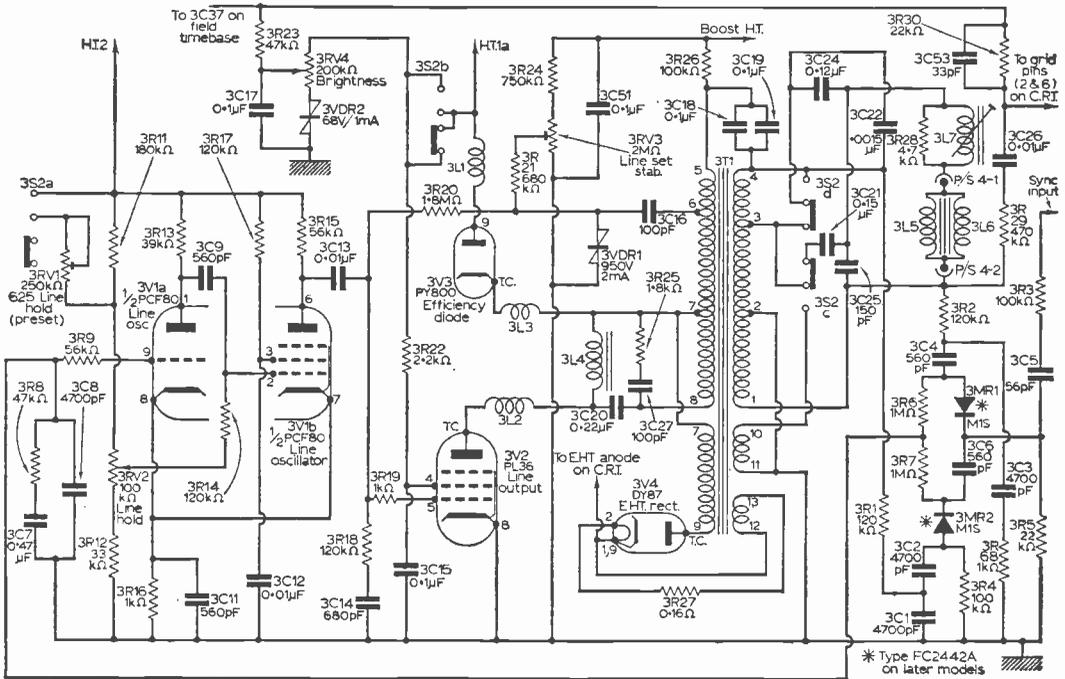
Fig. 6: Circuit diagram of the line timebase.
