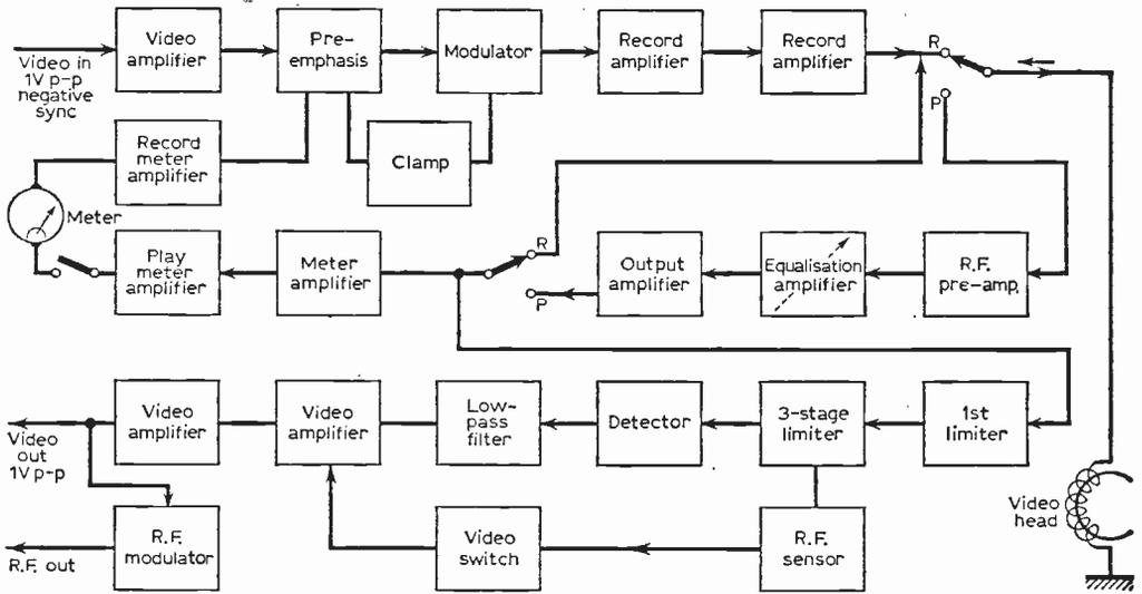
Fig. 5: Block diagram of the video signal circuits, Ampex Model VR6000.
