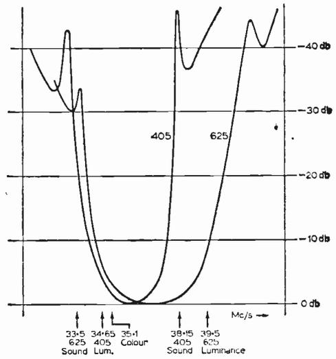
Fig. 28 (a) Suitable chrominance response for a separate chrominance detector. (b) 405-line response and a 625 compromise response using a single chrominance/luminance detector.
