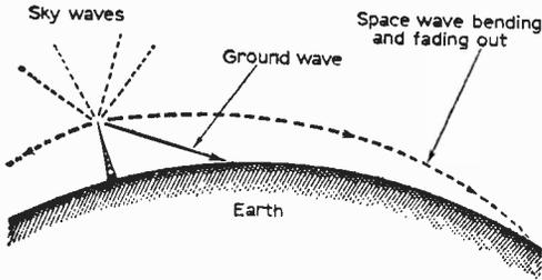
Fig. 2: The three types of wave radiated from a television transmitting aerial showing how the space wave bends slightly while reducing in intensity.
