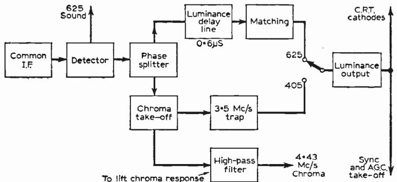
Fig. 29: A possible means of extracting luminance and chrominance information using a single detector, with suitable coupling arrangements to the luminance output stage.
