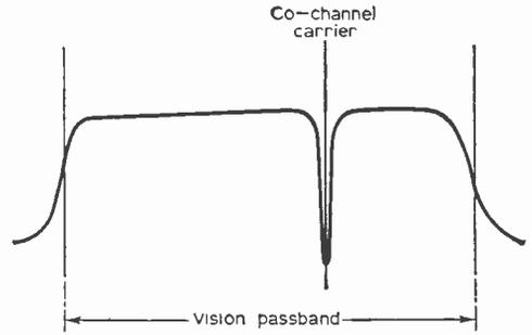
Fig. 6: How the Bovill filter "notches out" the interfering co-channel carrier.
