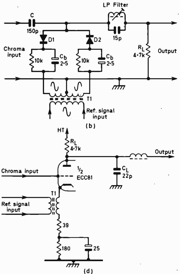
porated in the reference oscillator feed to the B-Y detector in order to achieve the correct  $90^\circ$  phase displacement between the instants of conduction of the two colour-difference synchronous detectors.
