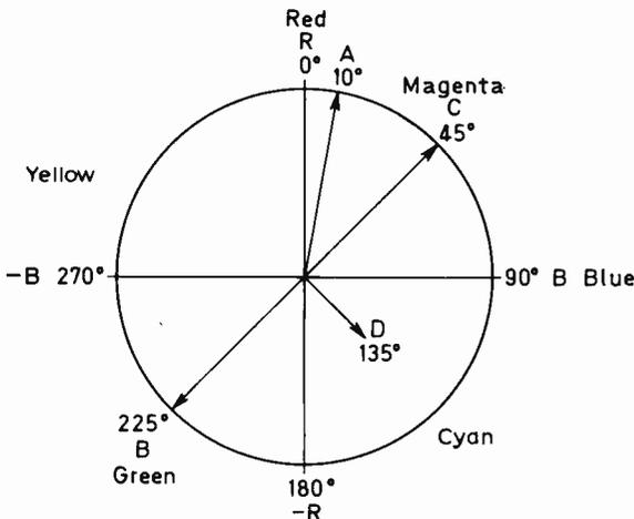
Fig. 3: The "colour clock": the phase of the chroma subcarrier varies to indicate different colours.
