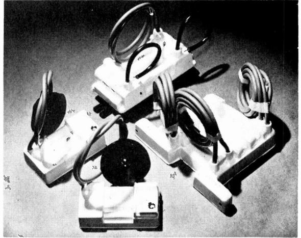
A selection of the replacement e.h.t. rectifier trays available from Clayridge Electronics Ltd.
