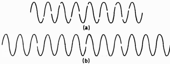
Fig. 7: (a) Diagrammatic representation of "quanta" or "wave packets". Note that the phase usually changes after each break. (b) Effect of quantum breaks at longer wavelengths (not to scale).
