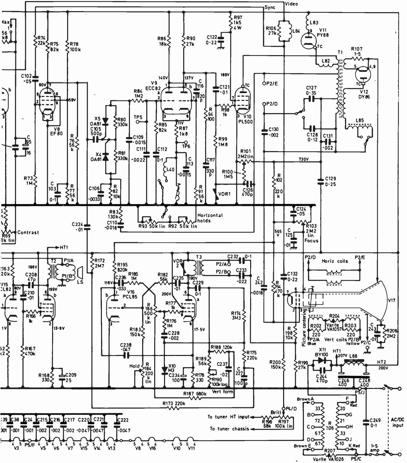
transformer (the v.d.r. will allow a little voltage to appear at pin 6 but not a lot).
