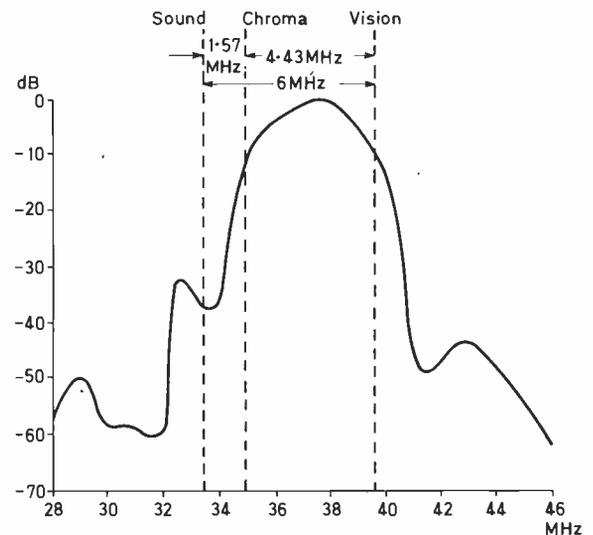
Fig. 2: Typical colour receiver response curve.
