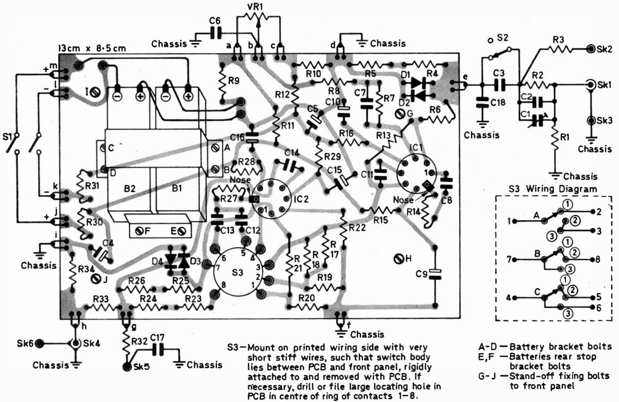
Fig. 4: Layout of the printed board, viewed from the component side.
