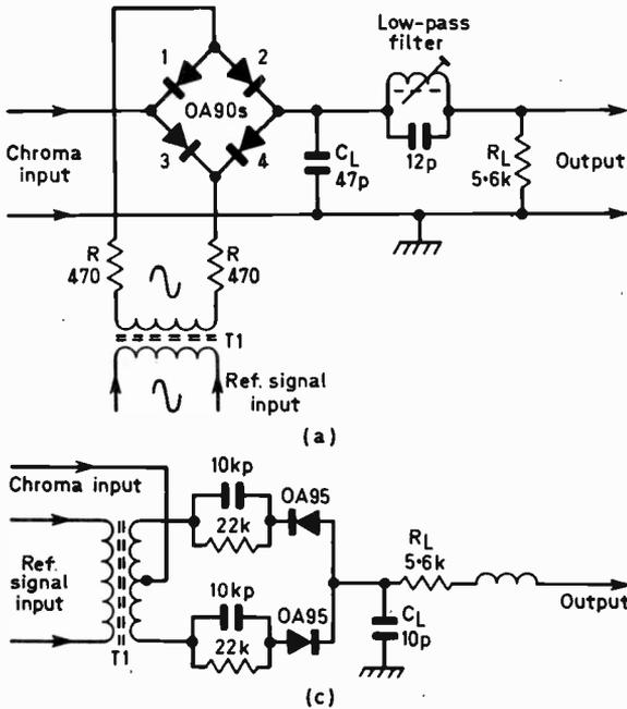
Fig. 4: Four types of synchronous detector: (a) series diode bridge; (b) shunt diode pair; (c) series diode pair; (d) triode valve.
