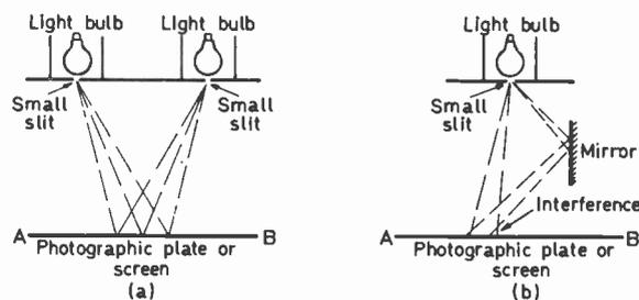
Fig. 6: Interference is seen only when one light beam is split into two sections one of which travels farther than the other. (a) There are no interference effects seen with this set up. (b) With one bulb and one slit, interference effects are seen.
