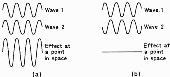
Fig. 1: Addition of waves.
