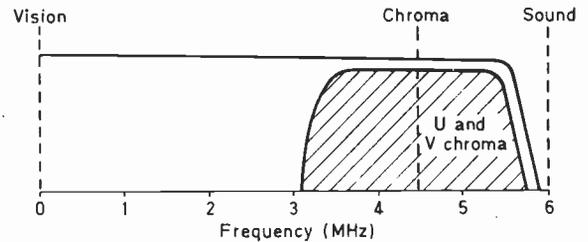
Fig. 1: Video frequency spectrum of the PAL colour television signal.
