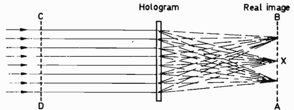
Fig. 5: If the hologram is held in a parallel beam of suitable waves the interference of these waves caused by the hologram forms a real image which can be projected on to a screen at position AB. If instead an observer's eye is at position X he will see the image at position CD.
