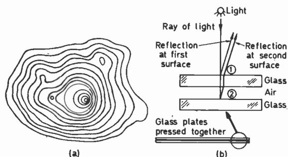
Fig. 3: Newton's rings. (a) Typical pattern seen between glass plates. (b) The two reflected waves have travelled different distances and their phase will depend on the spacing between the plates, which are never truly flat. Perfectly flat plates would show no pattern. Each space between rings represents a change of air gap of 50 millionths of a centimetre.
