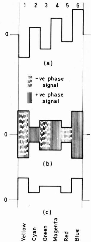
Fig. 2 (right): (a) The B-Y colour-difference signal for the standard colour-bar test pattern. (b) The signal shown at (a) modulated on to its subcarrier. (c) Output derived from (b) by a simple diode detector.
