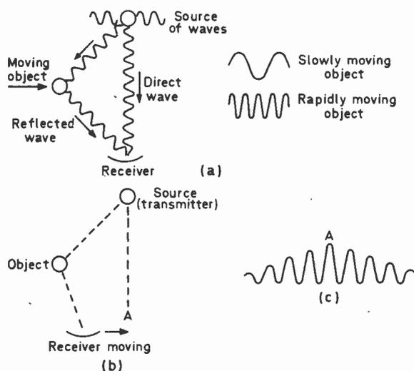
Fig. 2: (a) A moving object gives an interference signal which varies with time—it is in fact a sinewave. (b) Fixed object but moving receiver. (c) Pattern of waves picked up by the receiver. The peak amplitude is usually at the point where the receiver and transmitter are closest.
