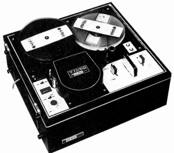
*The Rank Nivico KV810 videotape recorder.*
