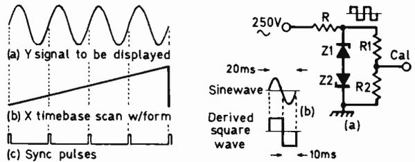
Fig. 5 (left): Relationship between the displayed signal, the timebase waveform and the sync pulses.
