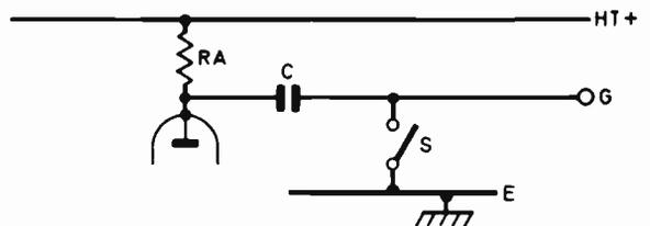
Fig. 4: Simple explanation of a clamp.
