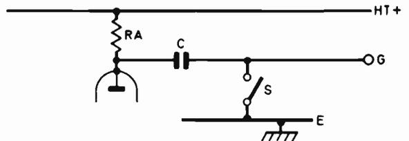
Fig. 4: Simple explanation of a clamp.
