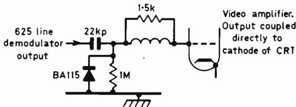
Fig. 3: The d.c. restorer used in the Philips 19TG170A series of models.
