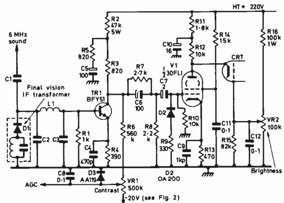
Fig. 1: The suggested video amplifier and a.g.c. circuit. A 6MHz retractor should be included in series with the grid or cathode of V1.
