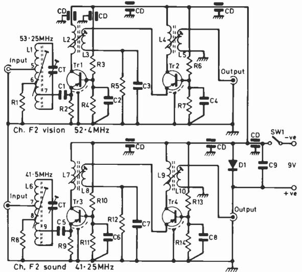
Fig. 1: Circuit diagram of the preamplifier used. The vision and sound channels are separate.
