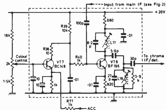
Fig. 3: Circuit of the controlled chroma i.f. amplifier stage in the Bush-Murphy single-standard chassis. Manual colour and automatic chroma control are applied via transistor VT7.
