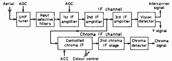
Fig. 1: Block diagram of the i.f. and detector sections of the all-transistor Rank-Bush-Murphy single-standard chassis.
