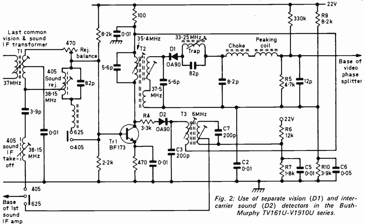
Fig. 2: Use of separate vision (D1) and inter-carrier sound (D2) detectors in the Bush-Murphy TV161U-V1910U series.
