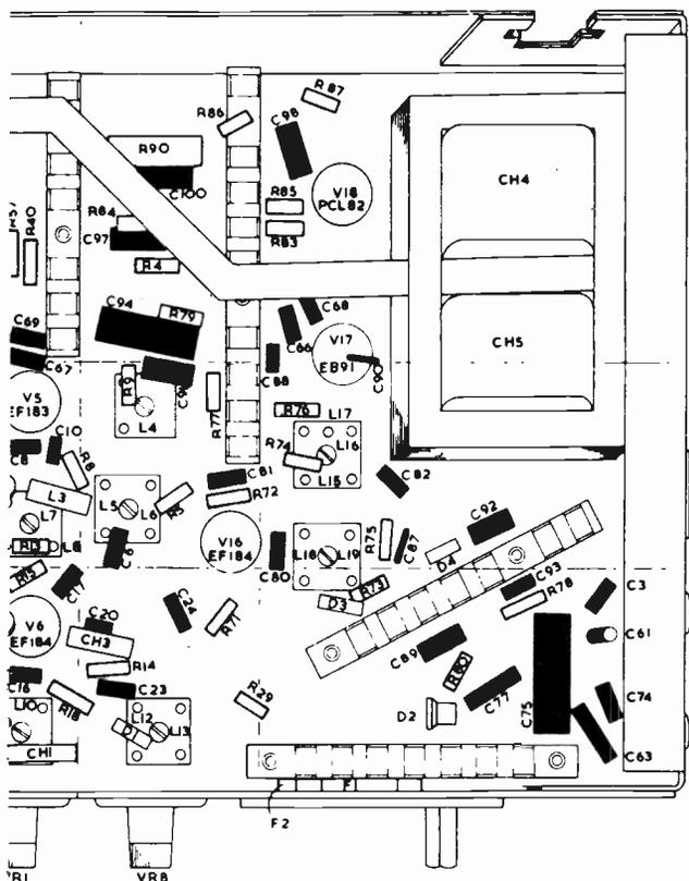
network. The main bias is developed across the 3.9kΩ resistor (R84) which is decoupled by C97 25μF. Now if this capacitor should become open-circuit the total feedback becomes excessive and the sound, although wonderfully pure, becomes hardly audible!
