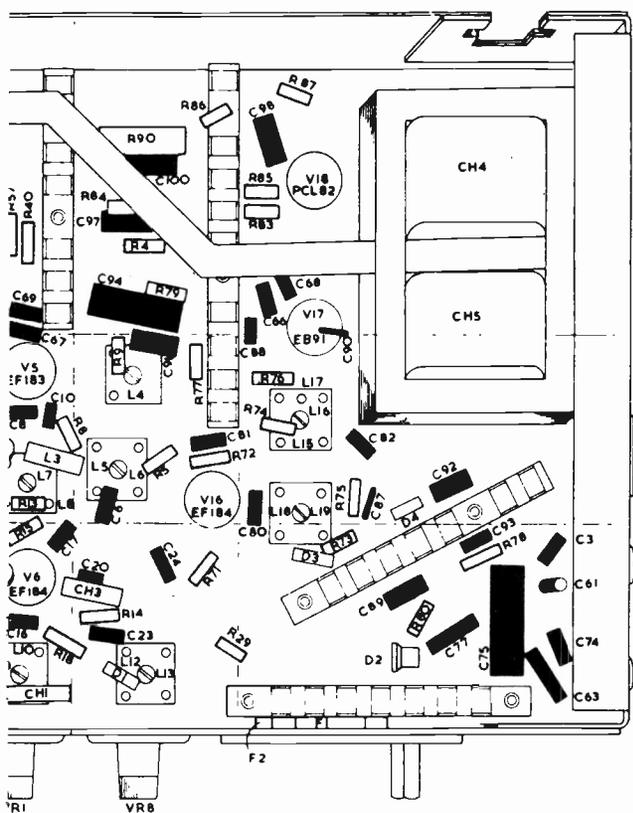
network. The main bias is developed across the  $3.9k\Omega$  resistor (R84) which is decoupled by C97  $25\mu F$ . Now if this capacitor should become open-circuit the total feedback becomes excessive and the sound, although wonderfully pure, becomes hardly audible!
