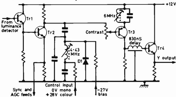
Fig. 7: Simplified circuit of the luminance preamplifier stages of the Bang and Olufsen 3000 chassis.
