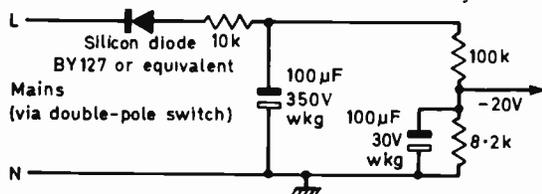
Fig. 2: Obtaining the -20V supply for the contrast control circuit.
