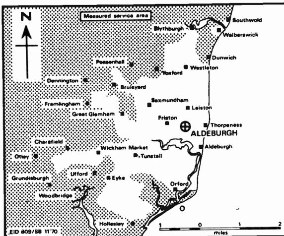
Channels: BBC-2 55; ITV 59; BBC-1 62. Horizontal polarisation, receiving aerial group C. Maximum vision e.r.p. 250kW.
