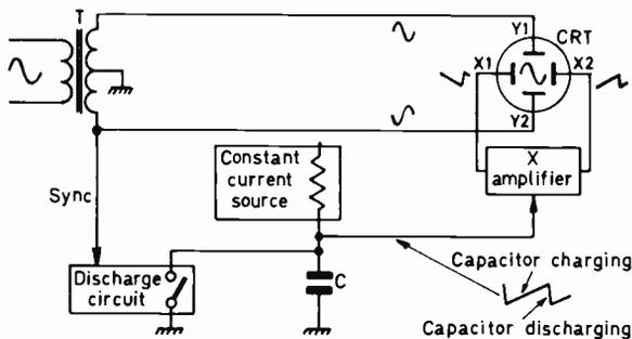
Fig. 3: The basic oscilloscope principle.
