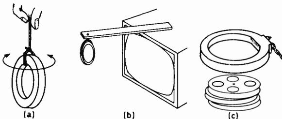
Fig. 3: Some improvised tools. (a) A focus magnet twirled on drive cord will degauss small impurities; move away from the shadowmask tube before stopping magnet rotation. (b) A 40p concave shaving mirror on a lath makes static convergence child's play. (c) Bulk tape erasure using a degaussing coil.
