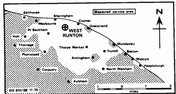
For both relay stations the channels are ITV 23; BBC-2 26; BBC-1 33. Vertical polarisation, receiving aerial group A. Aldeburgh maximum vision e.r.p. 10kW, West Runton 600W.
