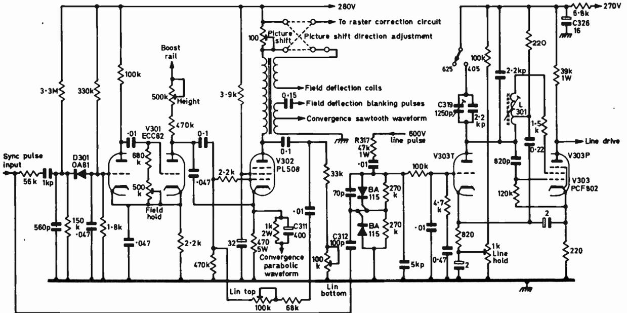
Fig. 1: Circuit of the Decca dual-standard timebase panel on which the line and field generators and field output stage are mounted. R317 47k $\Omega$  is a "favourite" in many chassis. It is 3R1 in dual-standard Rank-Bush-Murphy sets.
