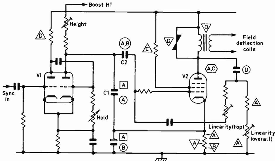
Fig. 2: Circuit of a representative field generator and output stage showing likely component defects and their effects on linearity.
