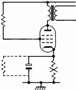
*Fig. 1: If a cathode bias resistor goes open-circuit the full h.t. then appearing across the bypass capacitor will break it down forming a leakage path. This will act as a "bias resistor" but of the wrong value, resulting in bottom cramping.*
