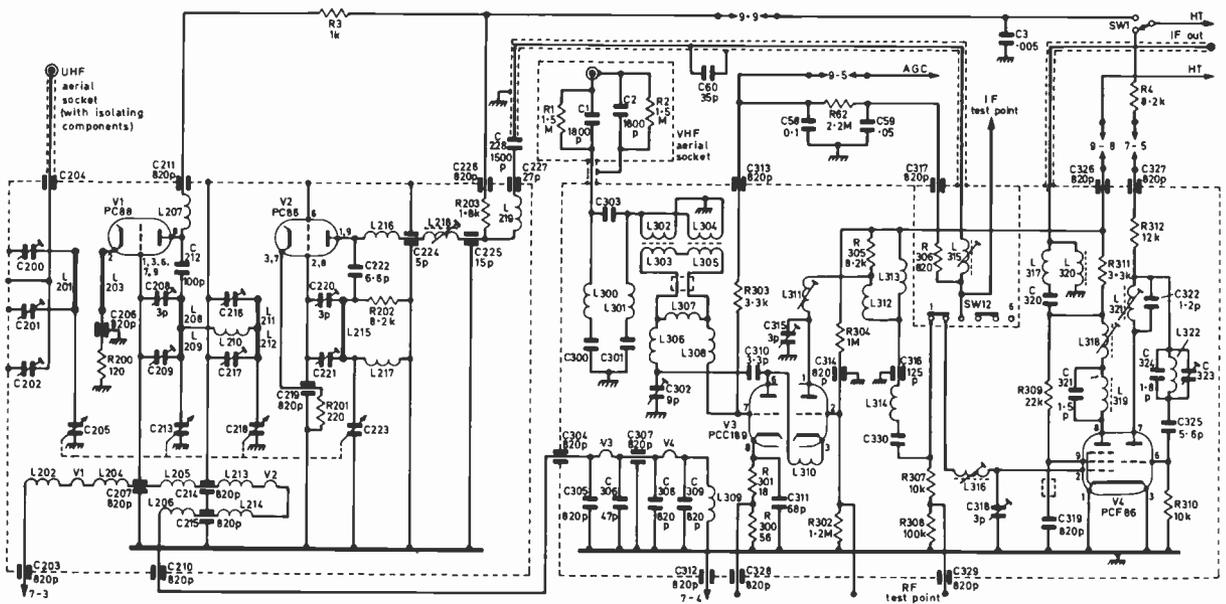
Fig. 4: Circuit diagram of the u.h.f. and v.h.f. tuner units.
