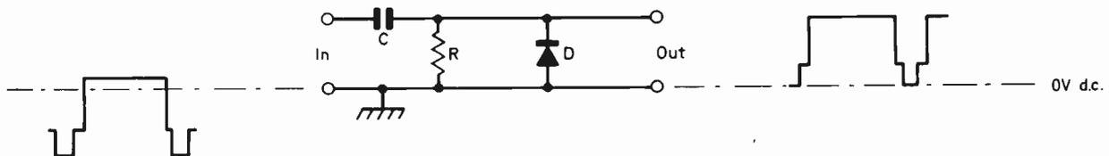
Fig. 2: The basic d.c. restorer and its effect.
