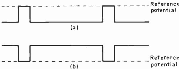
Fig. 6: D.C. restored clamp pulses, (a) at point A, (b) at point B.
