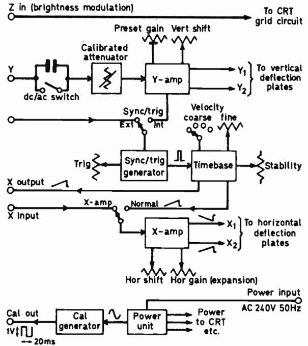
Fig. 4: Block diagram of the elements of a typical oscilloscope.
