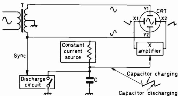
Fig. 3: The basic oscilloscope principle.
