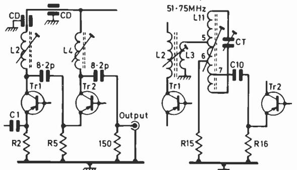
Fig. 2 (left): Alternative circuit using capacitive coupling between stages (the primary coils remain unaltered).
