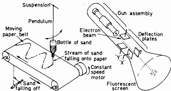
Fig. 1 (left): A mechanical analogy of the operation of an oscilloscope.
