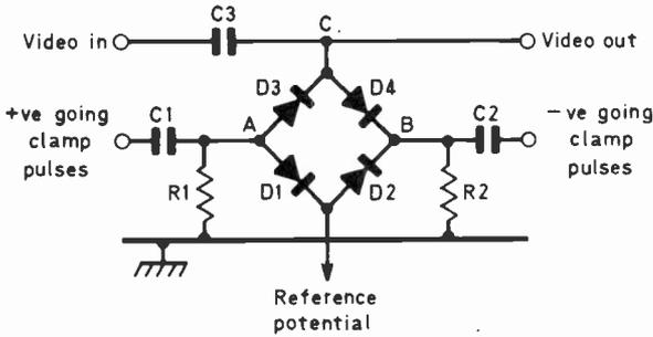
Fig. 5: The four-diode clamp circuit.
