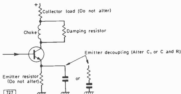
Fig. 8: The response of a video output stage can be modified by altering the damping of the peaking coil or the emitter decoupling.
