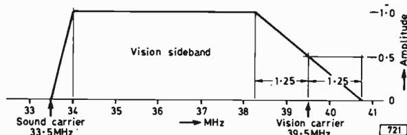
Fig. 2: The i.f. response of an "ideal" receiver matched to the vestigial sideband transmission. (Note that an amplitude of 0.5 = -6dB.)
