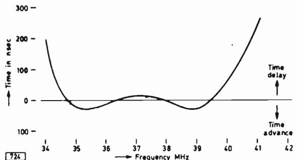
Fig. 5: A group delay curve for a complete i.f. strip.
