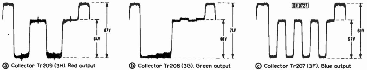
Fig. 2: RGB module waveforms.
