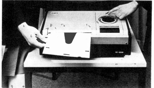
*The Telefunken TP1005 "TED" videodisc player. The 21cm. disc in its sleeve is inserted in the slot at the front of the player. The only controls required for operation are the start, stop and repeat buttons.*
