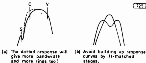
Fig. 6: All response curves should be as smooth as possible.
