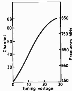
Fig. 5 (right): Tuning voltage plotted against channel setting with a vision i.f. of 39.5 MHz—Mullard ELC1043 u.h.f. varicap tuner.
