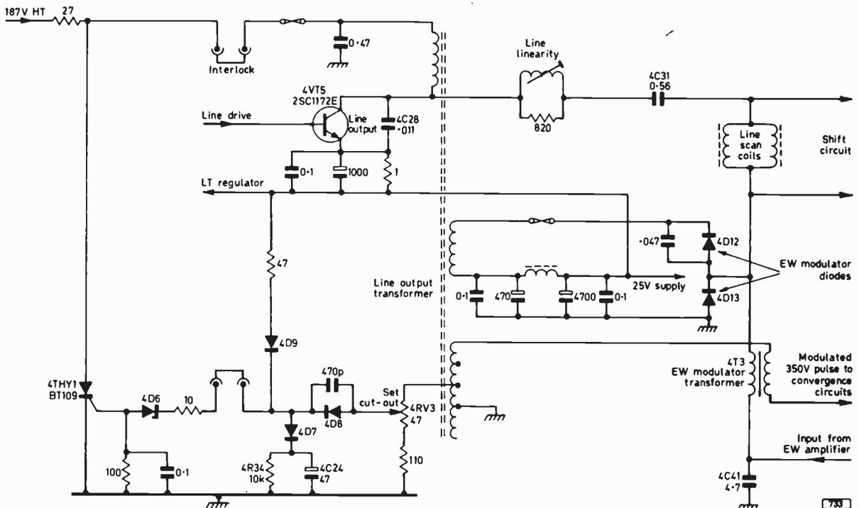
Fig. 4: Simplified circuit of the line output stage, showing the EW pincushion correction arrangements and the overvoltage protection system. The EW modulator diodes also provide the 25V supply.
