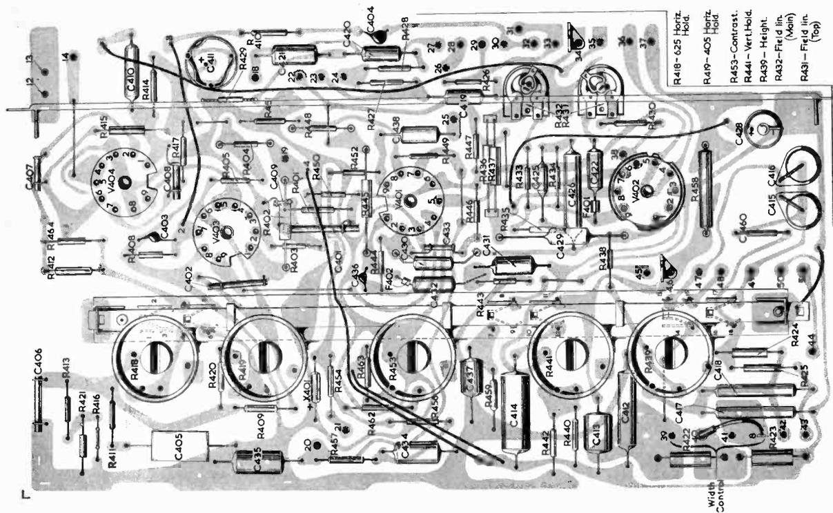
Fig. 2: Layout of the timebase printed panel, viewed from the component side.
