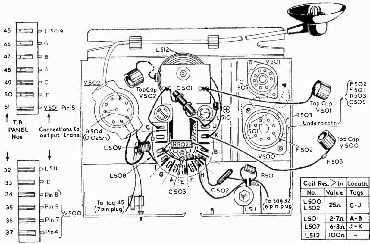
Fig. 3: Physical layout of the line output stage. When replacing the line output transformer clear the tags then unsolder the heater wires from V502 holder, accessible after prising out the top moulding. Coil d.c. resistances given where greater than 1Ω.
