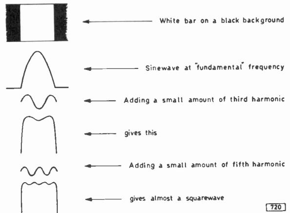
Fig. 1: A reasonable approximation to a squarewave (corresponding to a white bar on a black background) can be obtained by adding small amounts of third and fifth harmonic components to the fundamental sinewave.
