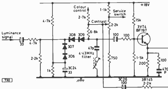
Fig. 1: Contrast control circuit. 3C26 and 3R145 form an anti-bounce network to prevent picture disturbance with rapid operation of the contrast control.
