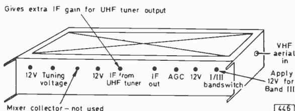
Fig. 2: Pin connections of the Philips v.h.f. varicap tuner available from Manor Supplies.
