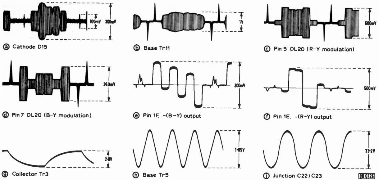
Fig. 1: Key decoder module waveforms.
