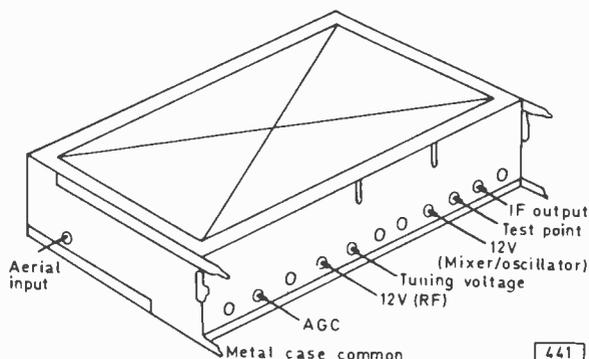
Fig. 1: ELC1043 u.h.f. tuner pin connections.
