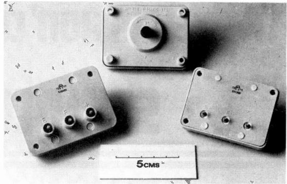
Fig. 2: High-voltage thick-film focus modules for use in colour TV sets. The circuit provides automatic focus voltage correction for wide variations in mains voltage. Courtesy Welwyn Electric Ltd.
