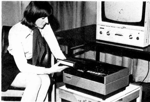
*The new IVC VCR100 series of video recorders combines the user convenience of cartridge loading—insert a cartridge, close the lid and press a button—with the quality obtained by using a 1in. tape format as in conventional IVC studio-type recorders. Marketed in England and Wales by Bell & Howell A-V Ltd.*
