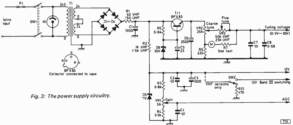
Fig. 3: The power supply circuitry.
