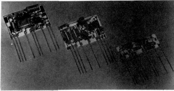
Fig. 1: Thick-film hybrid circuits for use in colour TV receivers. Courtesy Erie Electronics Ltd.
