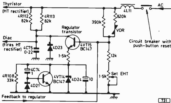
Fig. 2: Slow-start system in the power supply circuit.
