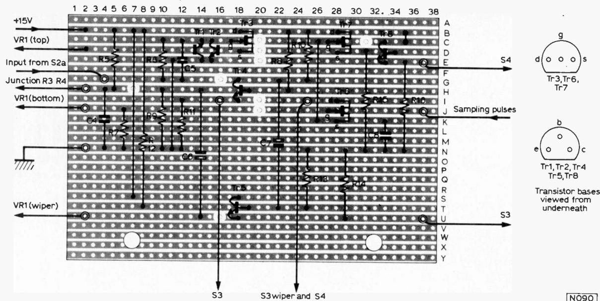
Fig. 10: Layout of the Preamplifier and Sample and Hold board, viewed from the component side. The copper strips should be broken at locations C20; C31; D20; E20; G16; H7; I20; J20; U16.
