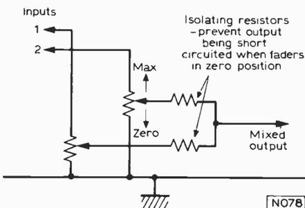
Fig. 2: Circuit of a simple audio mixer.
