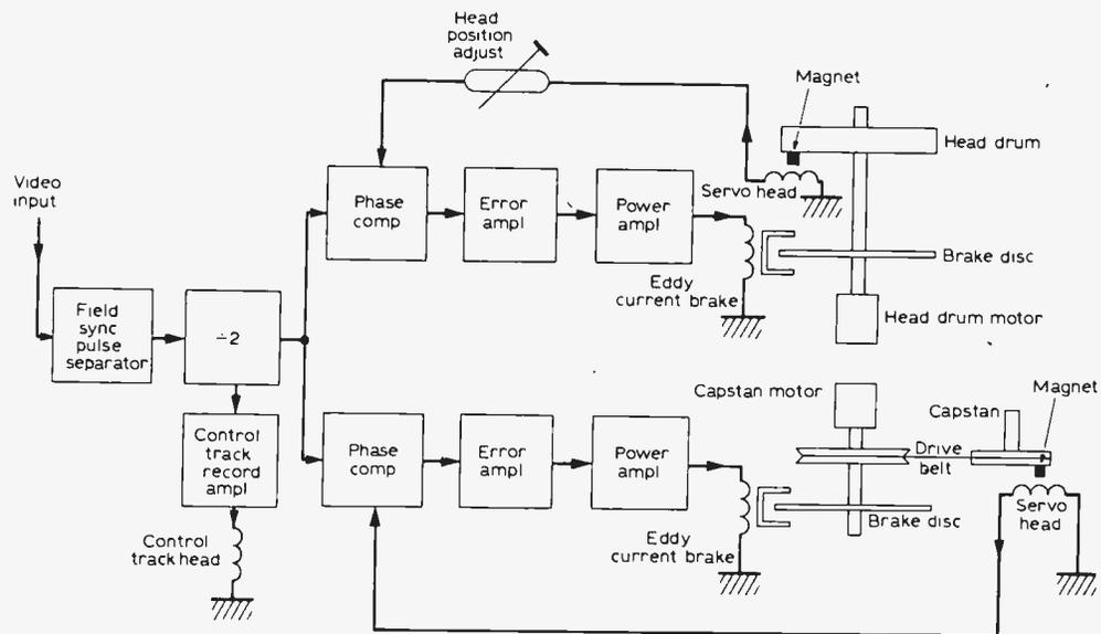
Fig. 16: A typical VTR servo system in the Record mode.
