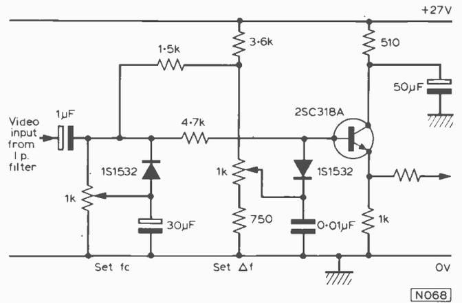
Fig. 11: Deviation control circuitry.
