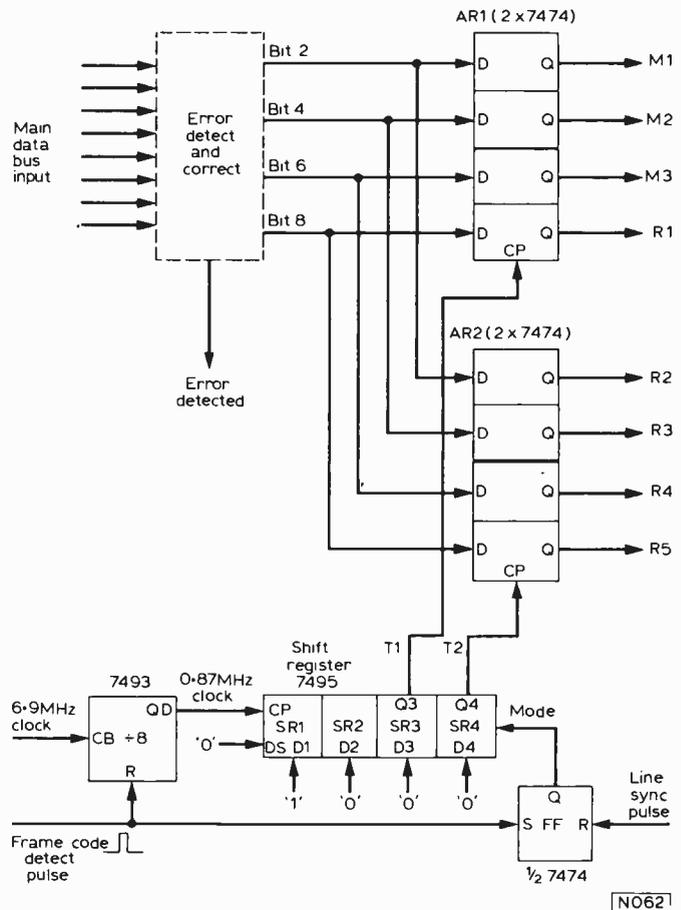
Fig. 13: One form of row address detection circuit.
