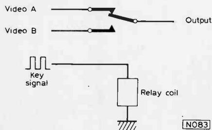
Fig. 7: An elementary split screen effect generator.
