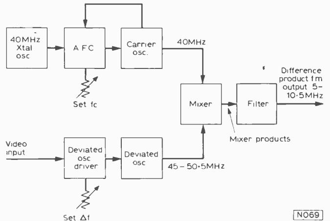
Fig. 12: Two-oscillator method of f.m. generation.
