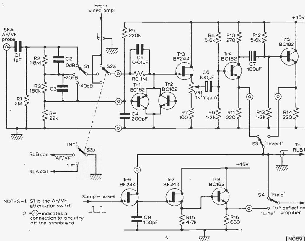
Fig. 9: Circuit diagram of the Input Attenuator and Preamplifier and the Sample and Hold circuit. Capacitors C2 and C3 are selected for optimum pulse response. In the prototype, C2 consisted of two insulated wires, twisted together for 30mm (1.25in), whilst C3 was a 36pF silvered mica capacitor.
