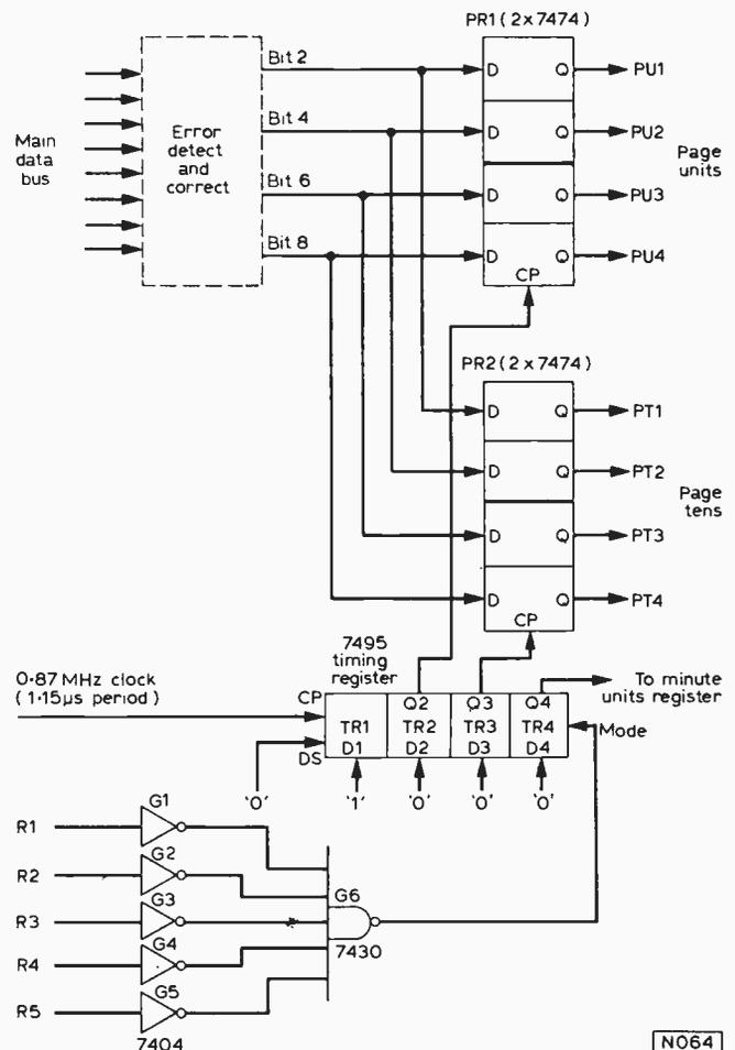
Fig. 15: A page address detection circuit.
