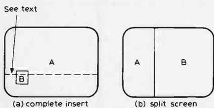
Fig. 6: Two types of insert and their appearance on the screen.
