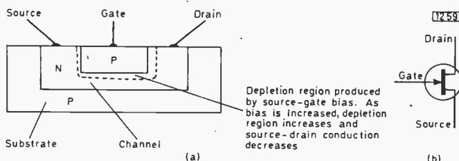
Fig. 1: (a) Basic construction of the junction gate field effect transistor, n-channel version. Conduction from source to drain via the channel varies as the bias applied between the source and gate connections alters. (b) Circuit symbol for an n-channel junction gate field effect transistor.
