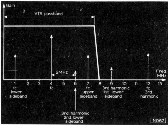
Fig. 10: The VTR spectrum and the production of "Moiré".
