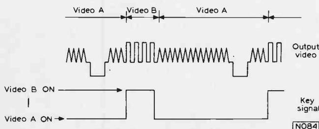
Fig. 8: Keying in an insert at line frequency.
