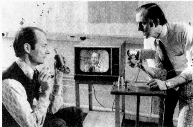
*The world's first entirely solid-state TV camera with broadcast quality resolution. Bell Laboratories engineer Carlo Sequin (left) shows the CCD sensor he designed to replace the bulky tube with its deflection assembly held in his left hand. His picture, taken by the experimental solid-state camera designed by Edward Zimany (right), appears on the 525-line monitor.*
