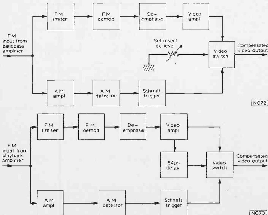
Fig. 15: Dropout compensation circuits.
