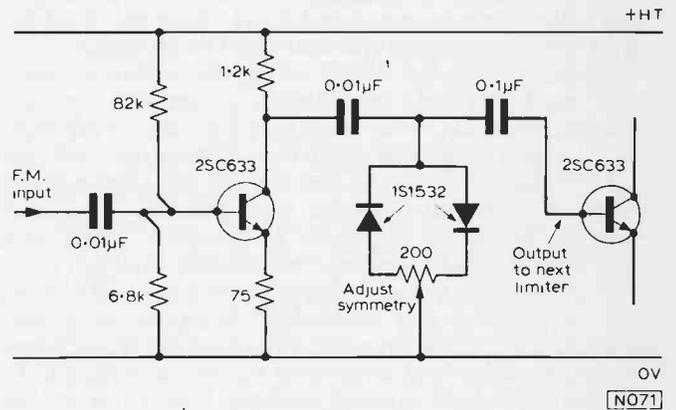
Fig. 14: A diode f.m. limiter stage.
