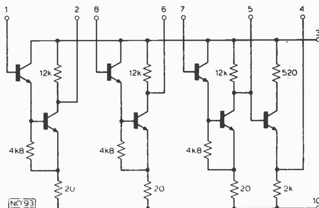
Fig. 3: Internal circuit of the TAA960 i.c.
