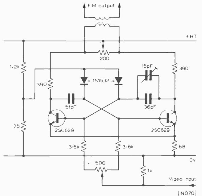
Fig. 13: A typical multivibrator f.m. generator.
