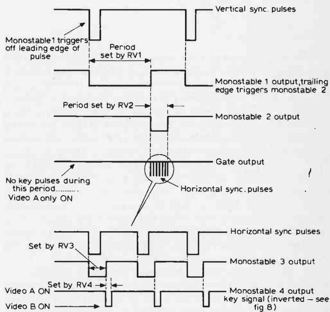
Fig. 9: Generating the box insert of Fig. 6(a).
