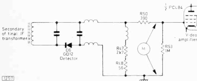
Fig. 1: Checking the forward and reverse resistance of the vision detector diode by means of a meter connected to the control grid of the video output valve. The circuit is as used in the ITT/STC VC3 dual-standard chassis, with the switching omitted for clarity. This test on the detector diode cannot be made with the set switched to 625 lines since the detector diode is capacitively coupled to the video output pentode on this system.
