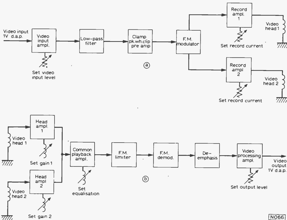
Fig. 9: The video system of a videotape recorder.
