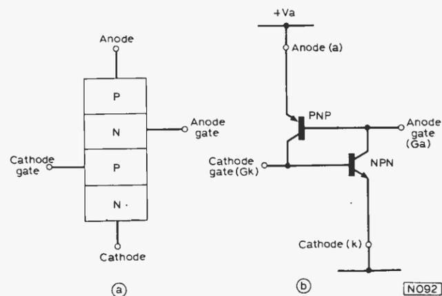
Fig. 2: The silicon controlled switch.
