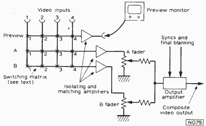
Fig. 3: Simplified circuit of a video mixer.
