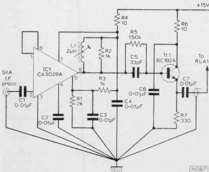
Fig. 7: Circuit diagram of the I.F. Preamplifier.
