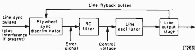
Fig. 1: Block diagram showing the basic elements of a flywheel line sync circuit.
