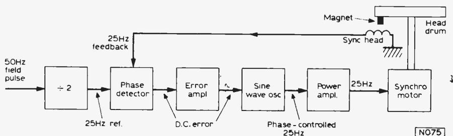
Fig. 17: A Record servo system using a phase-controlled oscillator.
