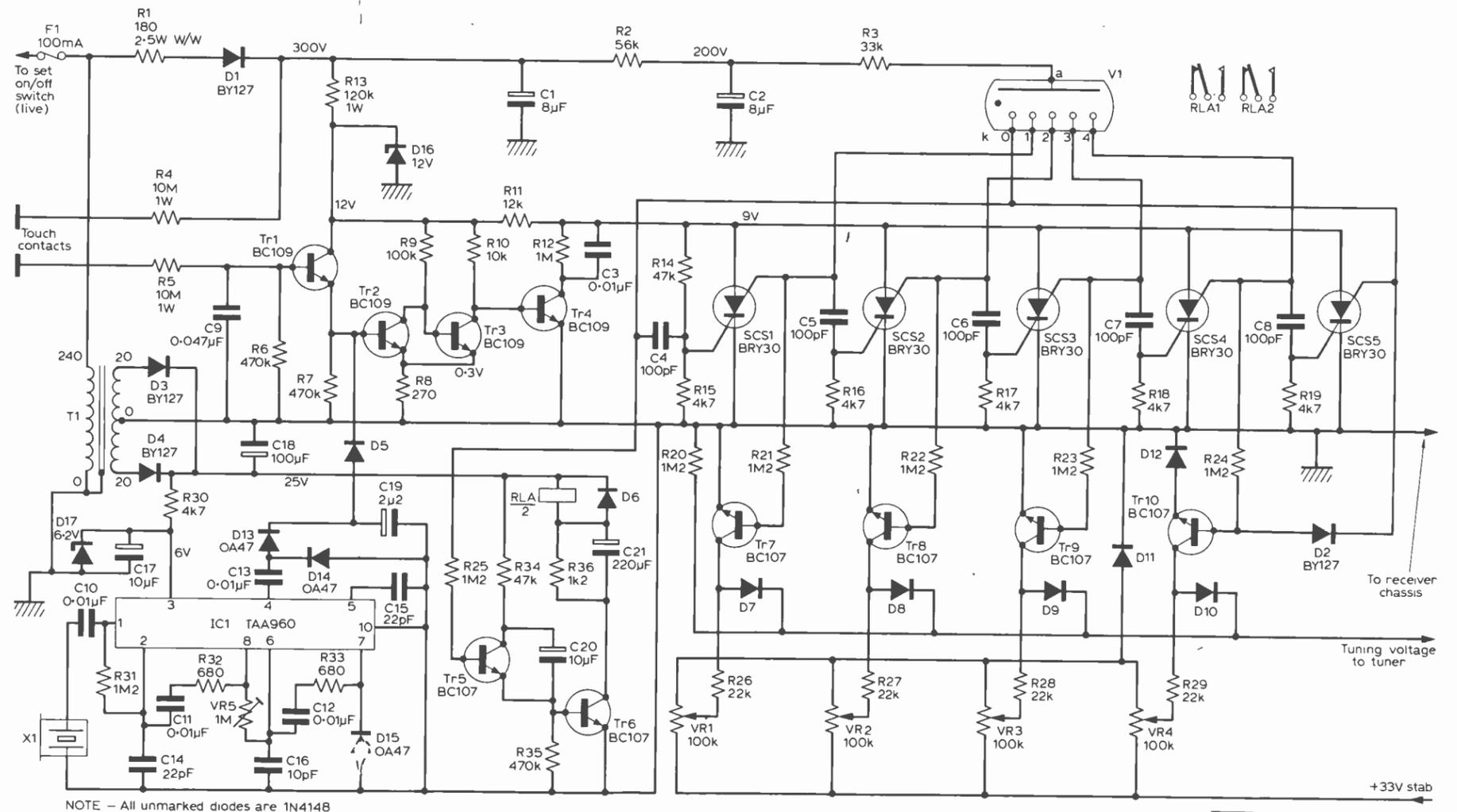
contacts are closed; on station No. 0 they drop out after a few seconds' delay. This delay is introduced to avoid the circuit switching off the TV when No. 0 is passed whilst changing stations.
