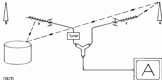
Fig. 4: The final installation. The tuner attenuates the signal picked up by aerial X when receiving station A.
