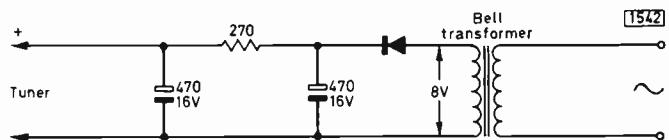
Fig. 3: Suitable power supply for the tuner — the component values shown are a guide only.
