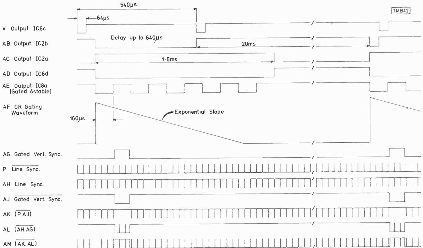
Fig. 5: Timing diagram with waveforms related to field rate. As with Fig. 4, these waveforms are ideal and some differences will be apparent when viewed on a scope.
