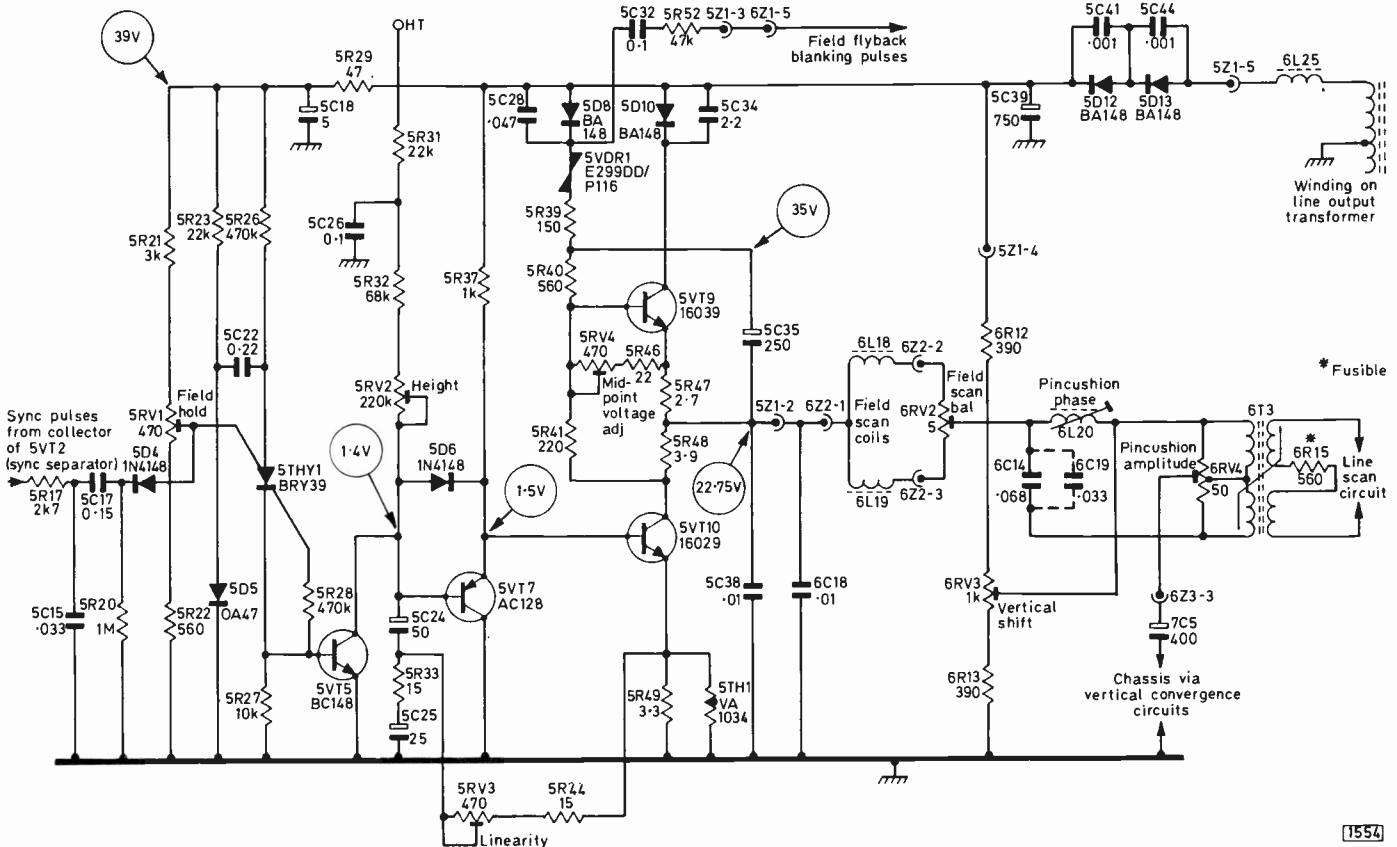
Fig. 1: Field timebase circuit used in the Rank A823A/AV/B chassis.
