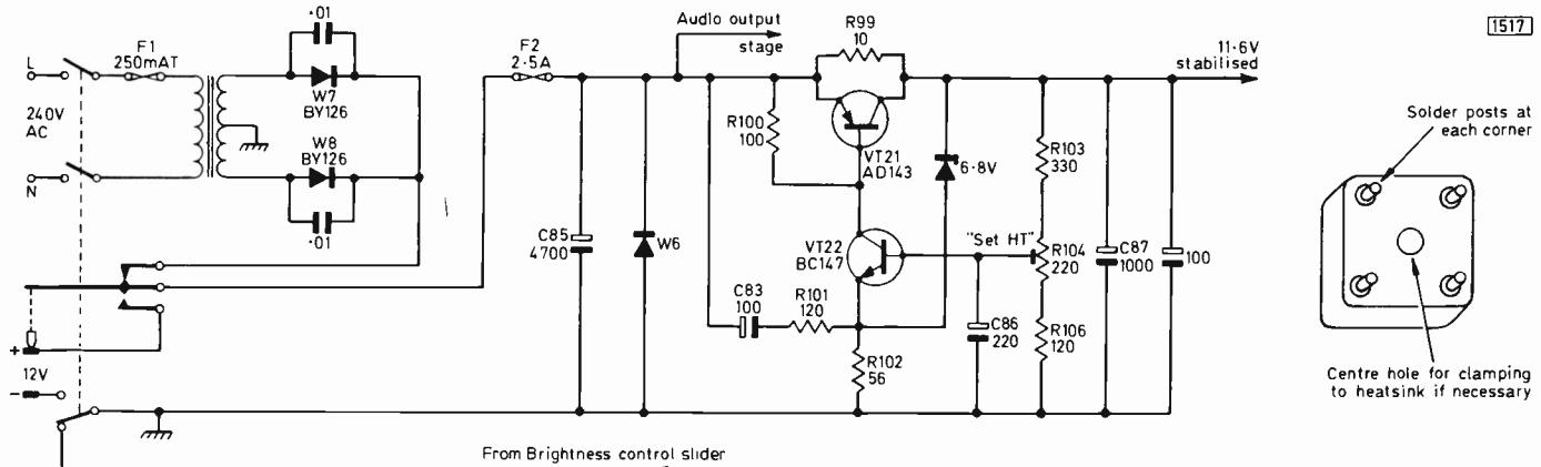
Fig. 5 (left): The power supply circuit used in the Thorn 1590/1/3 chassis. A suitable Mullard replacement for the series regulator transistor VT21 is the AD149.
