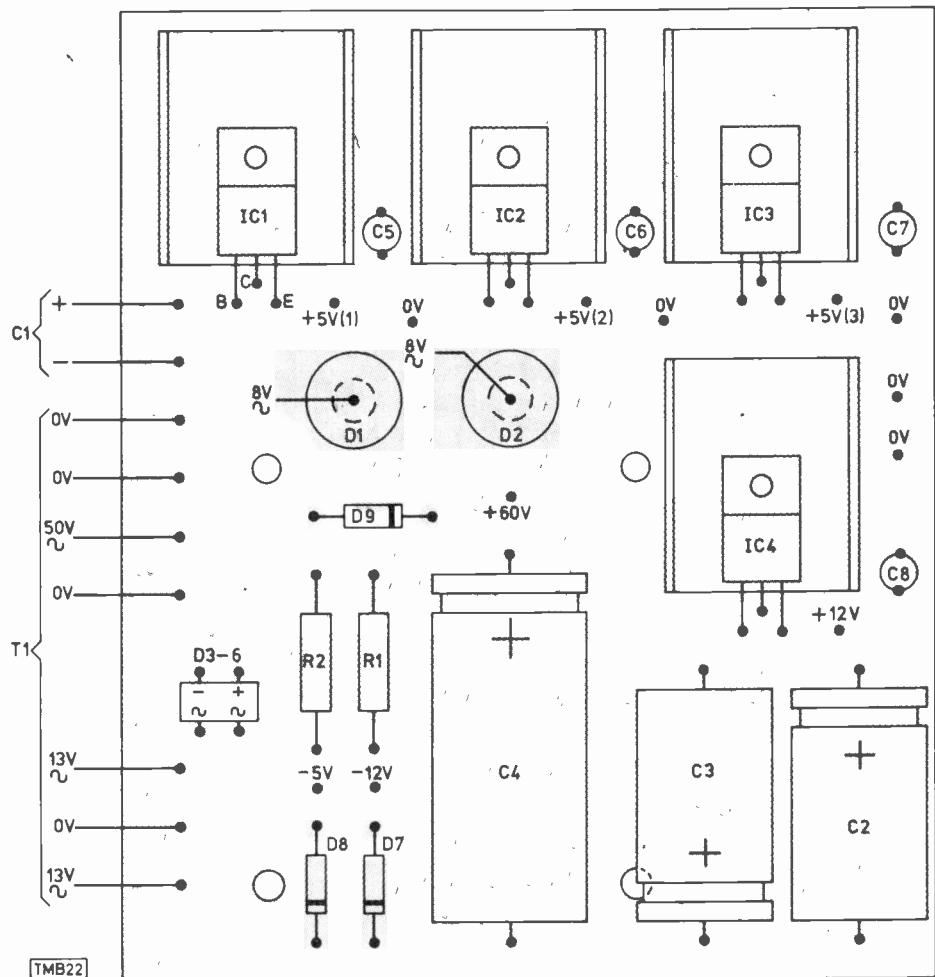
Fig. 4: Component layout diagram for the power supply.
