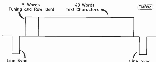
Fig. 1: Layout of transmitted data.
