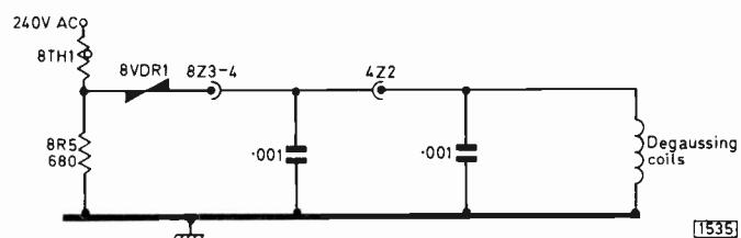
Fig. 3: The degaussing circuit used in the Rank 90° solid-state colour chassis. When the set is cold and 8TH1 in its low-resistance state, removal of 8Z3 will place 8R5 across the mains, leading to smoke when the power is applied.
