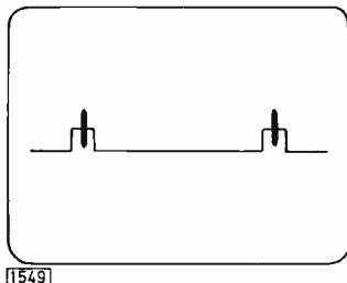
Fig. 6 (left): Typical oscilloscope showing a correctly adjusted burst gate.
