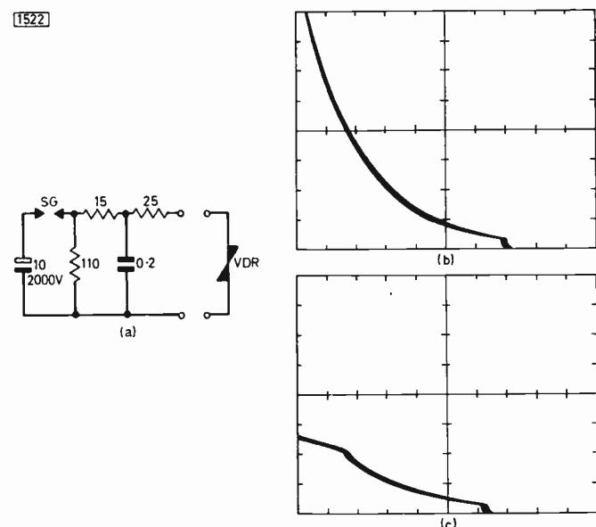
Fig. 1: (a) Lightning simulation test circuit. (b) Voltage waveform without the VDR in circuit. (c) Voltage waveform with VDR included. Vertical scale 200V/division, horizontal scale 500μs/division. Courtesy Mullard Ltd.
