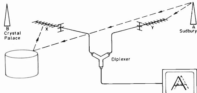
Fig. 1: The use of a diplexer simplified the installation but lead to unwanted signal pickup by aerial X during reception from station A (Sudbury), with the result that the picture was spoilt by ghosting.
