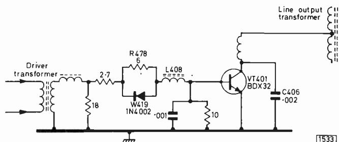
*Fig. 1: Line output transistor circuit used in the Thorn 8500 chassis. A dry-joint on L408 upset the drive conditions, leading to demise of the line output transistor and, subsequently, lack of width and loss of line sync when a replacement transistor was fitted.*
