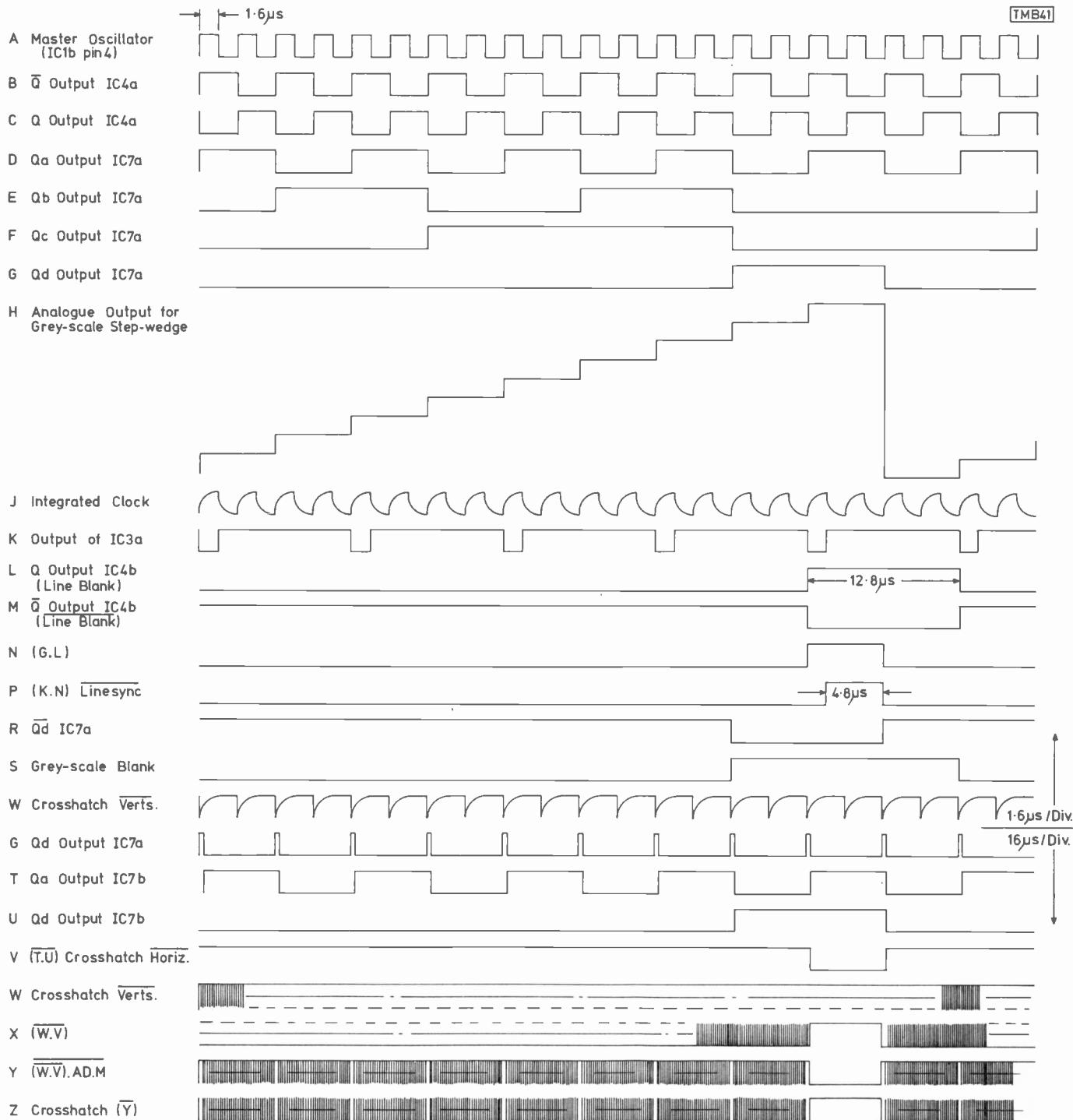
Fig. 4: Timing diagram. The waveforms above are related to line rate. Note that all waveforms except H are binary. S and Z have field components which are not shown. Shading on waveforms W, X, Y and Z represent fast pulses.
