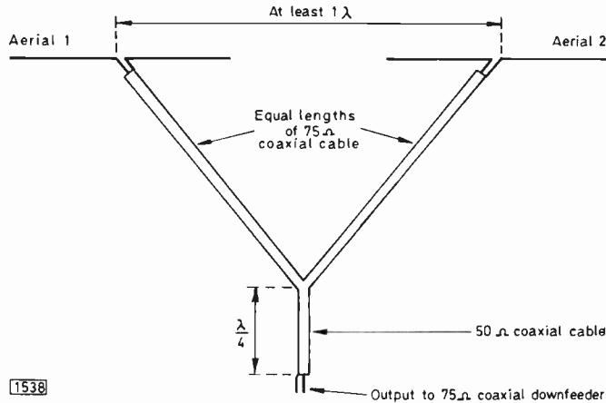
Fig. 1: Method of interconnecting two stacked aerials. To calculate a quarter wave, use the formula  $(246/f) \times$  cable velocity factor. Answer in feet; frequency  $f$  in MHz.
