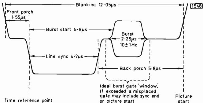
Fig. 5: Line flyback blanking period parameters.
