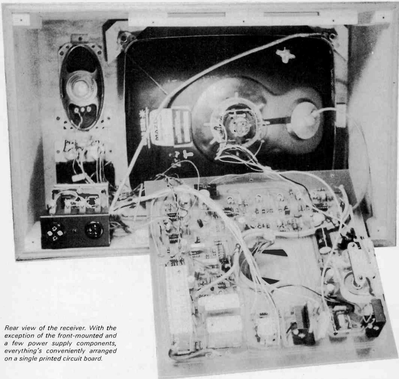
Rear view of the receiver. With the exception of the front-mounted and a few power supply components, everything's conveniently arranged on a single printed circuit board.
