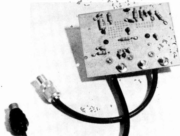
Component and print sides of the Jostykit HF385 v.h.f./u.h.f. amplifier board after completion of assembly.
