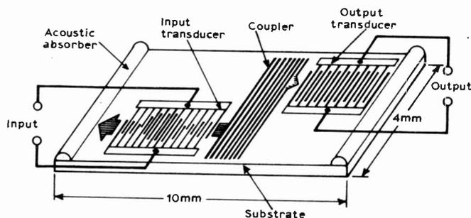
Fig. 2: (a) SAW filter structure.
