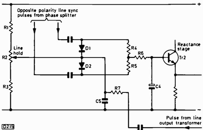
Fig. 4: Simple flywheel line sync discriminator circuit.
