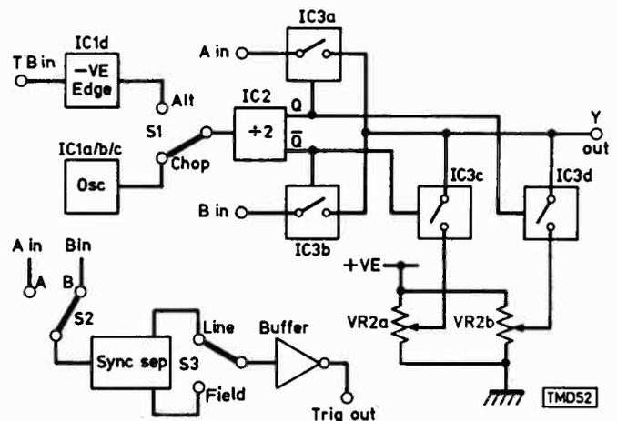
Fig. 1: Block diagram of the unit, showing the principles of operation.
