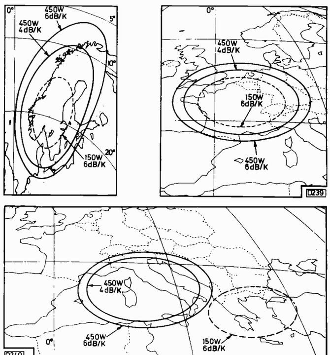
Examples of the OTS-2 satellite's European "footprints". Top left, coverage of Scandinavia by both beams (450 and 150W). Top right, coverage of Western Europe with both beams directed at the same area. Bottom, Southern European coverage, with the 450W beam directed at Italy and the 150W beam at Greece.
