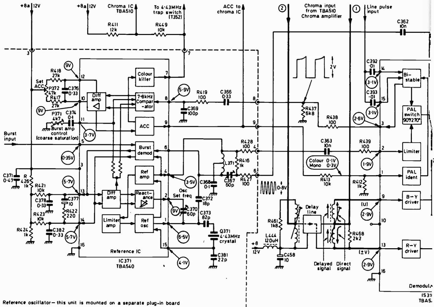
Fig. 15: The reference oscillator, demodulator and lumina
