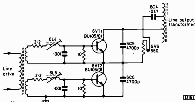
Fig. 2: Line output transistor circuit, Rank A823 chassis.
