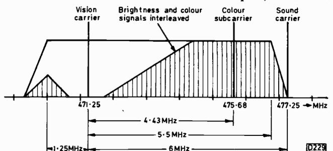
Fig. 1: Relative positions of the signals in a television channel. The carrier frequencies shown are for channel 21.
