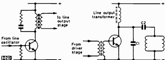
Fig. 5 (left): Basic features of a line driver stage.
