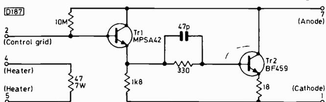
Fig. 1: A solid-state PL802: resistors 0.33W unless otherwise indicated; 47pF capacitor ceramic plate.
