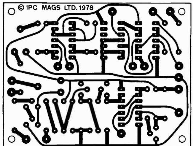
Fig. 2: Suggested printed board pattern for the unit.
