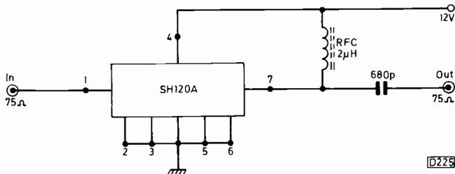
Fig. 2: Test circuit for the SH120A thick-film wideband signal preamplifier i.c. This version operates at 12V with a current consumption of 20mA. The input pin is d.c. isolated internally by means of a 680pF, 50V capacitor.
