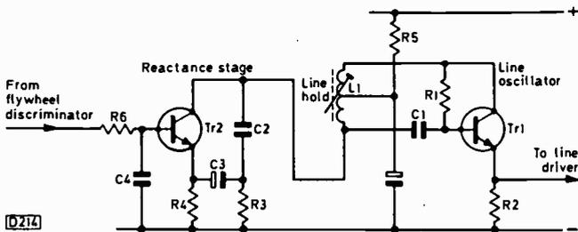
Fig. 3: Simplified line oscillator/reactance stage circuit.
