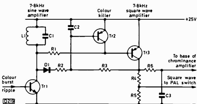
Fig. 9: The colour-killer arrangement used in the Thorn 8000 series chassis. The colour burst ripple input is taken from the burst detector: the ripple arises due to the phase changes ( $\pm 45^\circ$ ) of the burst signal on alternate lines.
