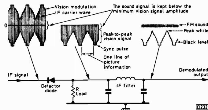
Fig. 4: Demodulation using a diode and LC filter.
