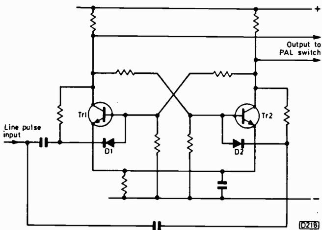
Fig. 8: A bistable multivibrator triggered at line frequency to provide 7.8kHz outputs to drive a PAL switch. Simplified by omission of the ident circuit which synchronises the PAL switching in the receiver with that at the transmitter.
