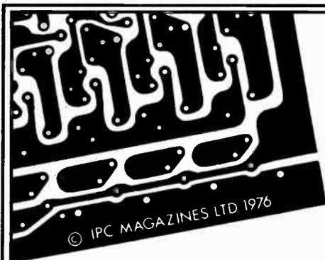
All boards are epoxy glassfibre and are supplied ready drilled and roller-tinned.
