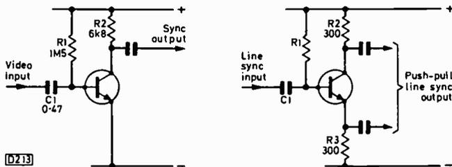
Fig. 1 (left): Typical sync separator stage.
