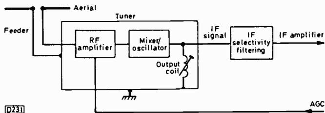
Fig. 3: Signal path up to the first i.f. amplifier transistor.
