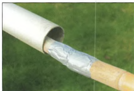
Fig. 2: Bamboo canes taped end-to-end and fed up inside the antenna mast.
