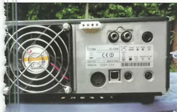
Fig. 3: The back panel, with external interfaces and cooling fan.
