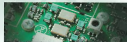
3 kHz and 15 kHz Roofing Filter
