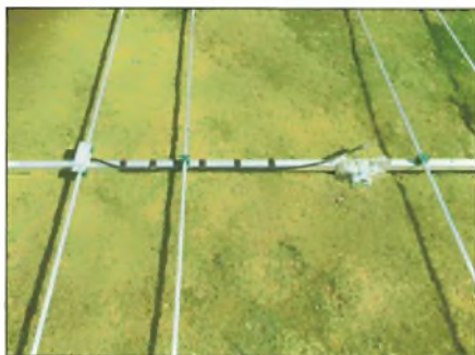
Fig. 4: The antenna comes complete with a short length of Ecoflex 10 cable connected to the driven element weatherproof housing and fitted with an N-type female connector at its far end. The cable is secured to the boom as shown. I placed the boom to mast clamp 1820mm forward of the rear reflector so as to achieve a mechanical balance.
