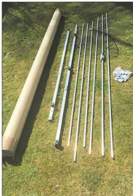
Fig. 2: The PowAbeam 6m Yagi prior to assembly. All hardware is stainless and comes in a sealed packet. The Stauff insulator blocks are all factory mounted on the boom, which comes in two sections. The heavy duty cardboard container can be seen on the left of the picture.
