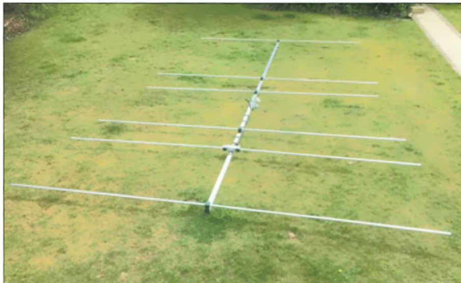
Fig. 3: The completed antenna laid out on the lawn prior to mounting on the tower.
