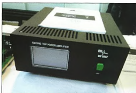
As we reported last month, several new amplifiers were on show. Here is the solid-state OM 2002 for the 144MHz band.
