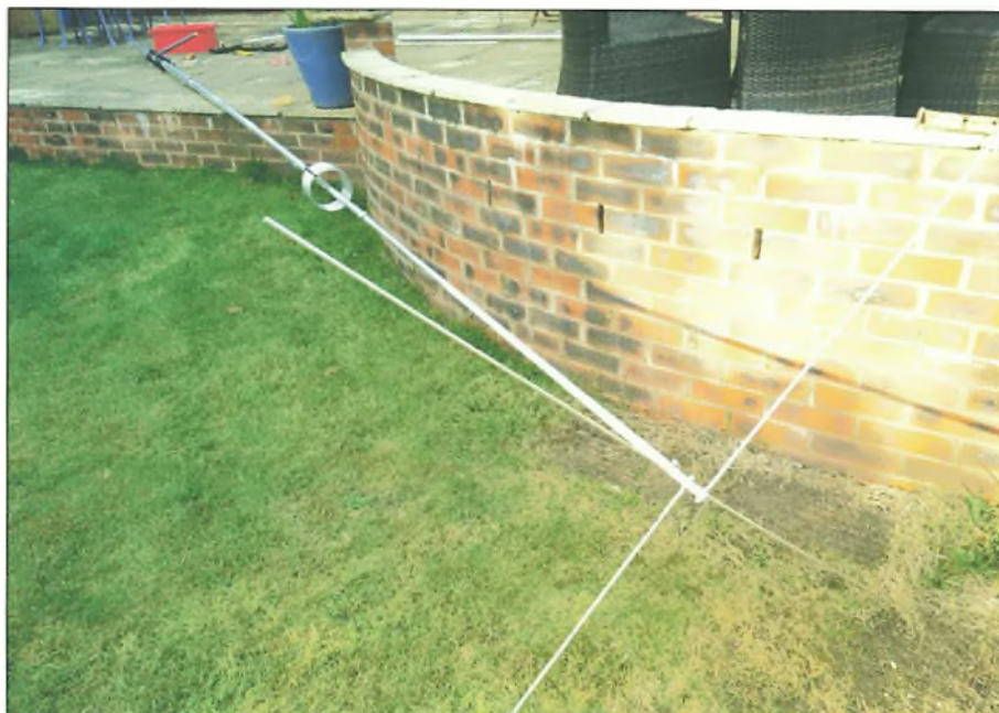
Half the dipole – the loading coil and capacity hat can be seen clearly.
