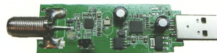
Fig 2: An internal board view of an RTL-SDR.
