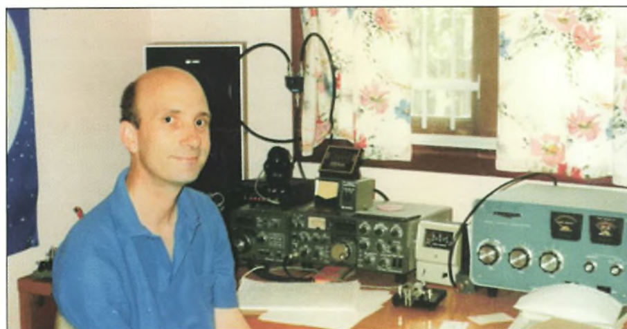
The Heathkit SB-220 (far right) is a classic 80 – 10m linear amplifier, using 3-500Z triodes, pictured at VK6VZ in 1990.
