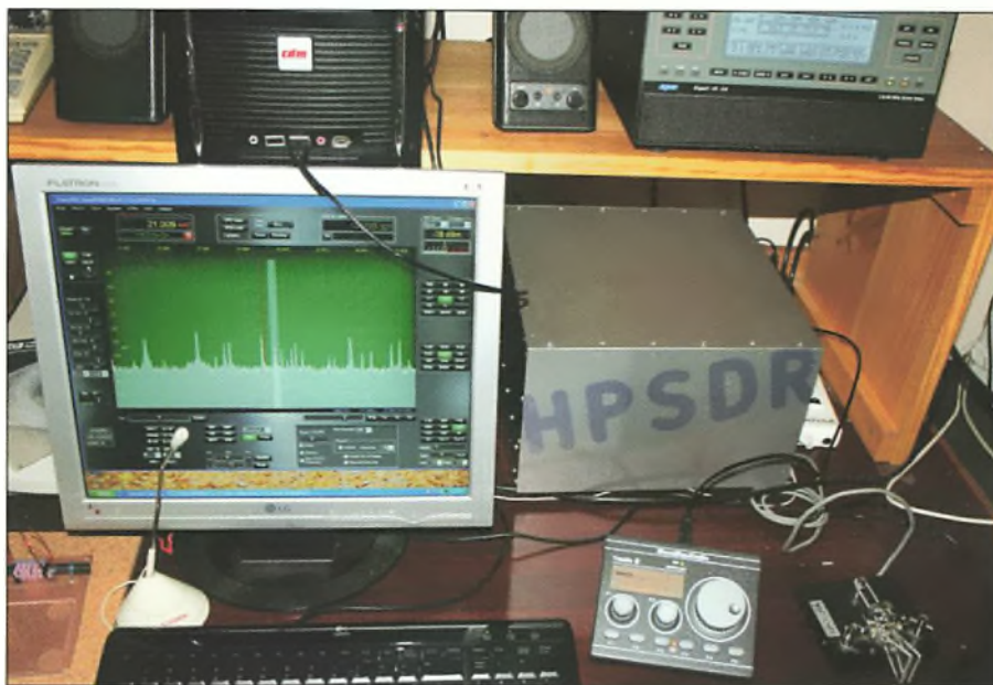
A modern SDR HF 400W HF station, using the Expert 1K-FA linear amplifier (at upper right).
