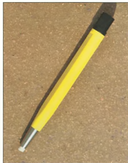
Fig. 5: An abrasive fibreglass pencil can be useful for cleaning a small area of a PCB.
