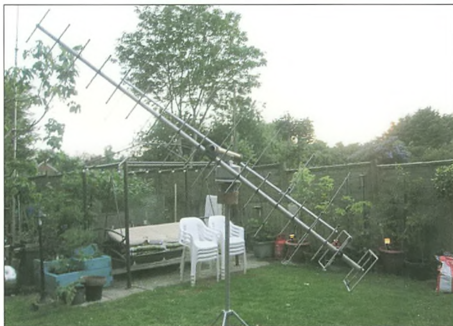
Fig. 1: MOJEC's homebrew AZ/EL rotator, powered by a Raspberry Pi computer.
