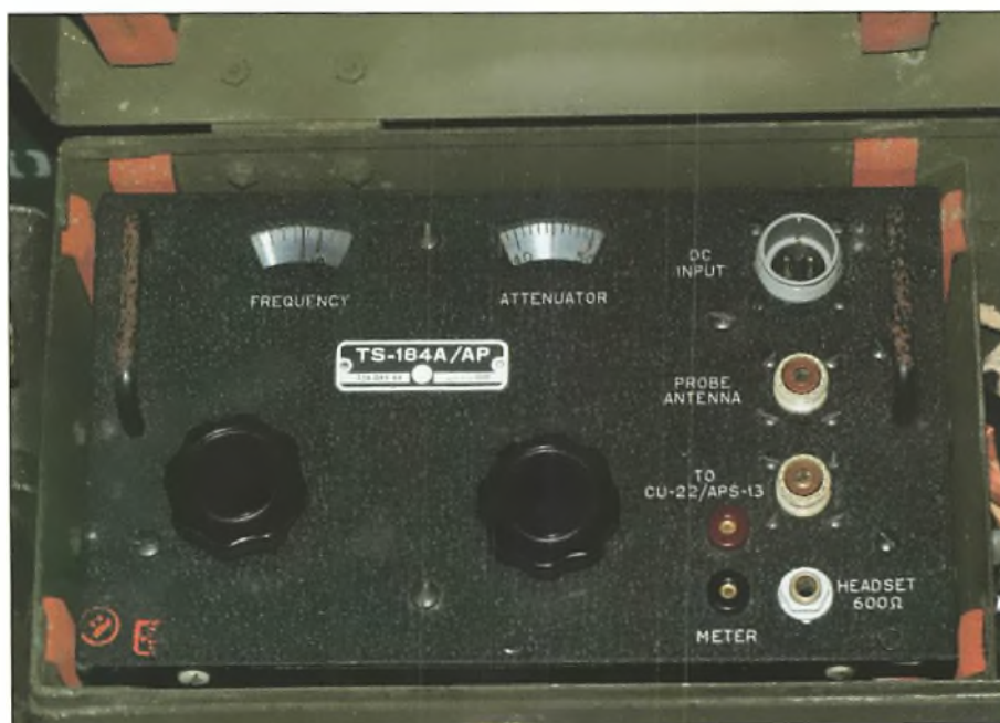
Fig. 9: Simplified controls on the set.
