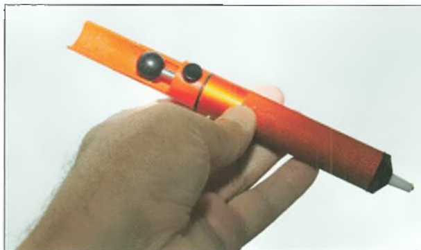
Fig. 9: A solder sucker helps to remove solder from a joint before removing a component.
