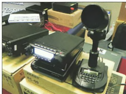
The new FT-891, FC-50 ATU and M-1 microphone from Yaesu, on show on the ML&S stand. The M-1 has two independent elements, graphic equaliser, memories for recording and playback and much else.
