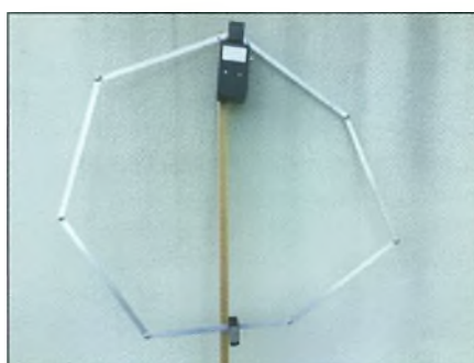
Fig. 5: The 10/12m loop with remote tuning box.
