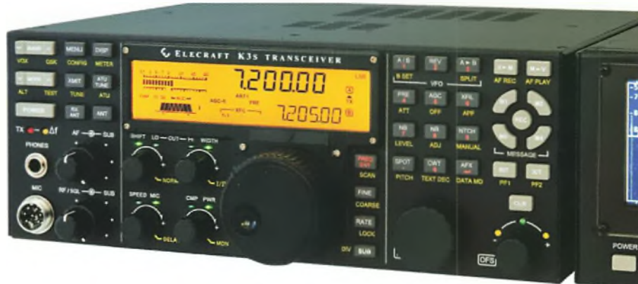
Fig. 2: A top specification Elecraft K3 transceiver can be assembled from pre-soldered PCBs.
