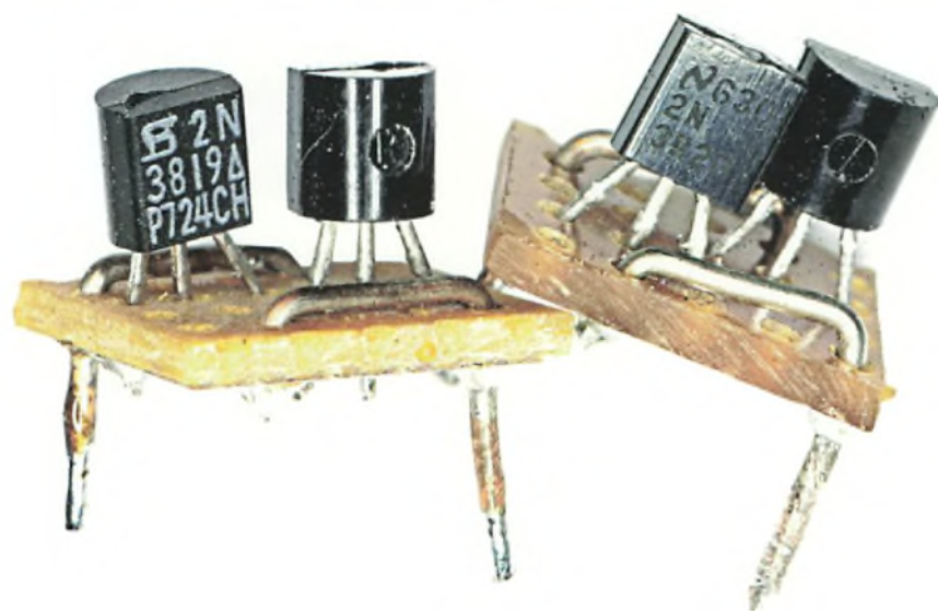
Two versions put together on small pieces of stripboard.
