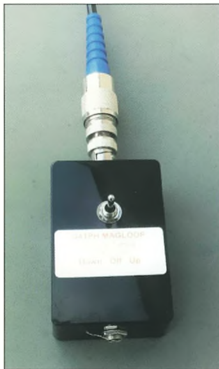
Fig. 7: The switch box as used at the shack end.
