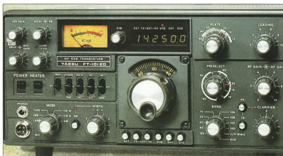
Fig. 3: The FT-101ZD is a great rig but needs a rear panel link before the PA will operate.
