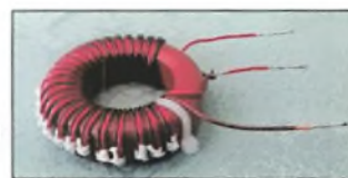
Fig. 4: A photograph of the finished toroidal balun.
