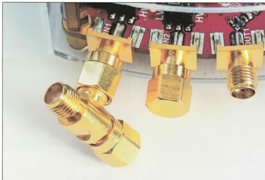
Fig. 2: SMA tee connector and 50Ω termination.
