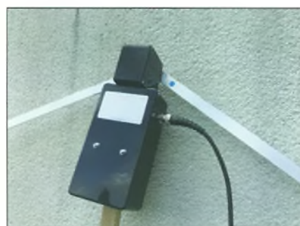
Fig. 6: A close-up of the remote tuning box.
