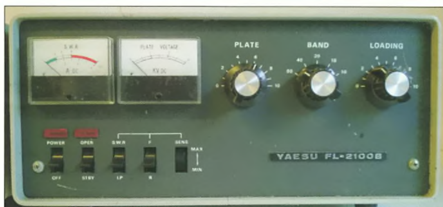
The Yaesu FL-2100B HF linear amplifier, using a pair of 572B valves.
