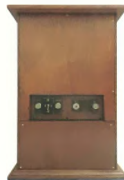
A rear view of the Chakophone 1B showing the speaker terminals.
