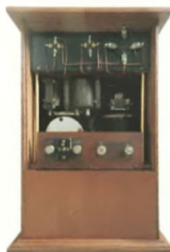
The rear of the Chakophone 1B with the back panel removed for access and maintenance.
