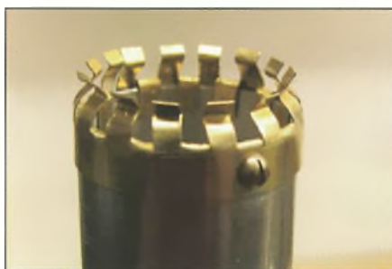
Fig. 9: The fitted fingerstock, secured with M4 nuts.
