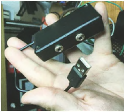
Fig. 8: The completed project. No batteries needed as all power is drawn from the USB connection itself.
