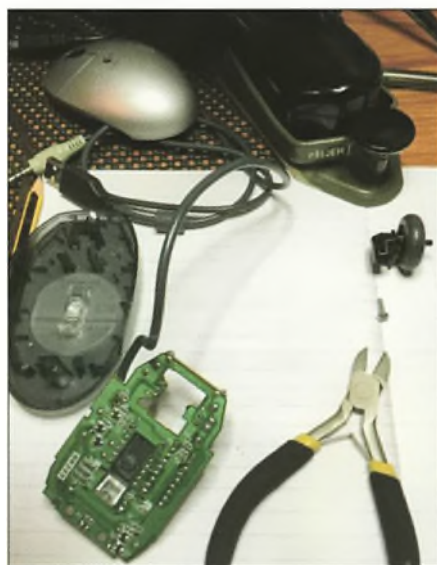
Fig. 1: An old mouse disassembled in order to access the left mouse button contacts. Remember, this switch is normally open.
