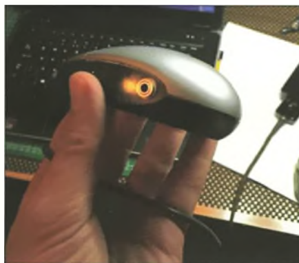
Fig. 3: The reassembled mouse with the subtle new addition of the jack. The mouse operates entirely as normal even when inserting the plug to your key. The key simply extends the use of the mouse button.
