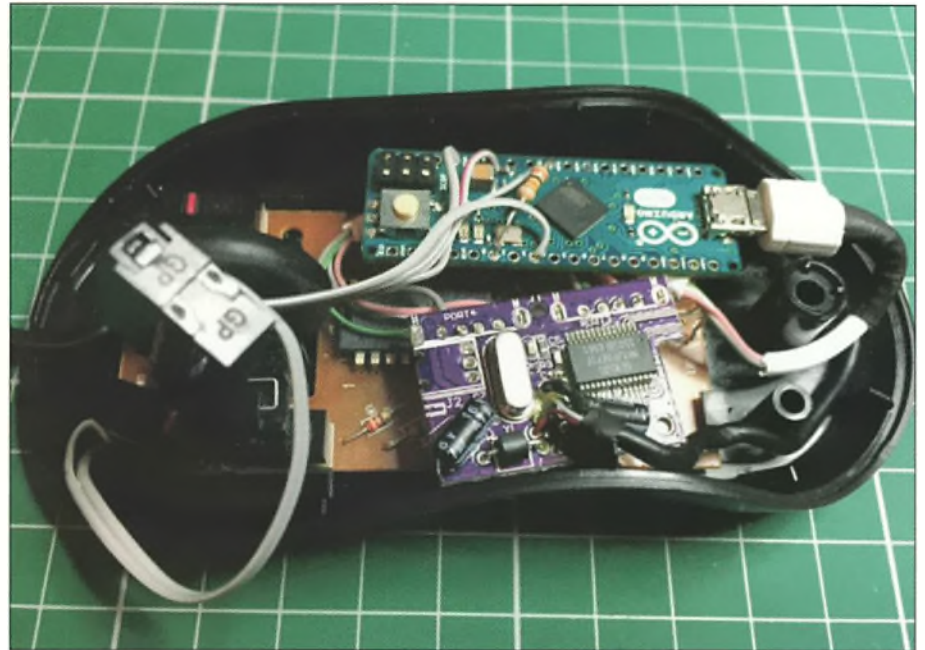
Fig. 10: Combining an optical mouse (brown board), Arduino Micro (green board) and 2-port USB hub (purple board) entirely inside the mouse itself.
