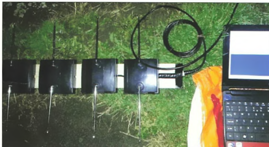
Fig. 3: The homebrew antenna made by Kevin M0GTD to receive the 70cm signals from the ISS digipeater.
