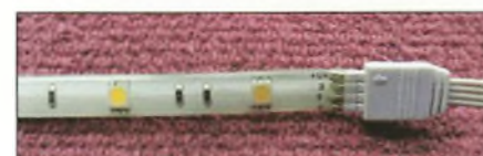
Fig. 4: Strips of LEDs incorporating surface-mount resistors can be daisy-chained using suitable connectors. They are ideal for use under shelves to illuminate operating positions or work benches.
