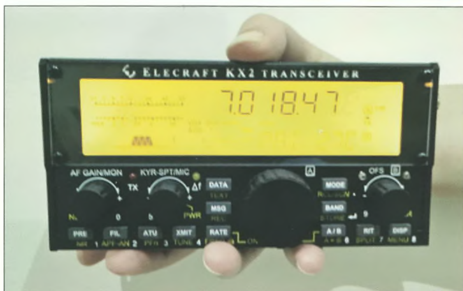
The KX2 really is a handheld HF transceiver. Here the subsidiary display is showing PA temperature.
