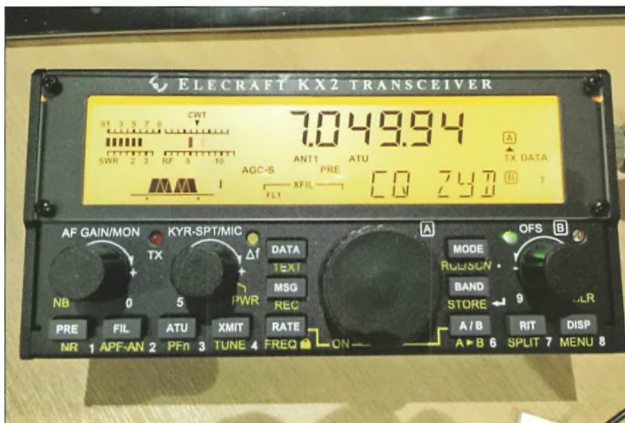
The KX2 decodes a CQ on RTTY. Note (to left of display) that the filter receives just the two RTTY tones, with a notch between them – something only digital filters can do.
