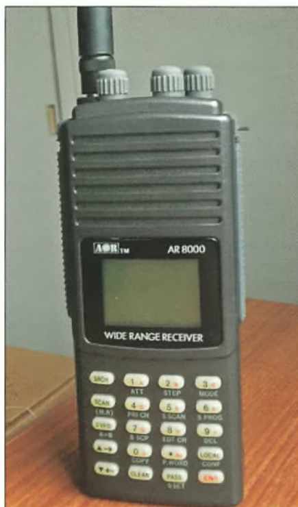
Fig. 1: Dick thought his AOR scanner was insensitive but the truth was that it was his friend’s receiver that was also receiving image signals.
