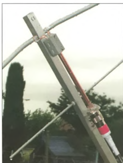
Fig. 1: The 2-element Yagi used at MX0CNS for the 70cm moonbounce contacts with HB9Q and DL7APV.
