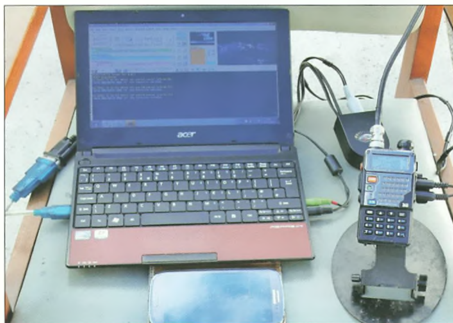
Fig. 3: The portable APRS setup used by Kevin M0GTD/ZB2GI for contacts through the ISS digipeater.
