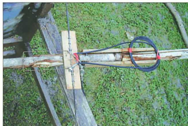
Fig. 4: The U-shaped hairpin matching system, along with coaxial phasing line.
