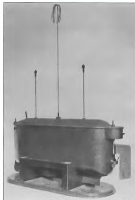
Fig. 6: Nikola Tesla's 1898 radio-controlled boat.
