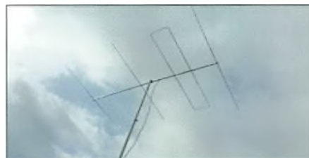
A 4-element 50MHz LFA-3 Yagi.
