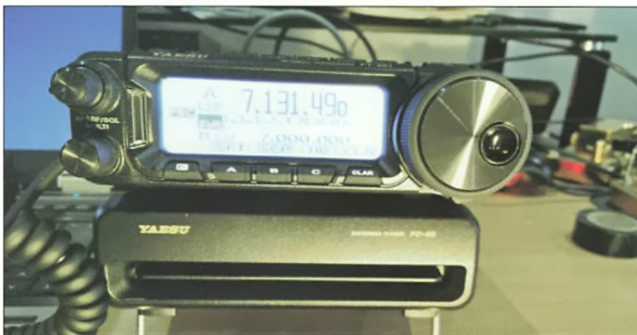
Fig. 2: The FC-50 ATU, below the FT-891 (But not attached with the Yaesu brackets).
