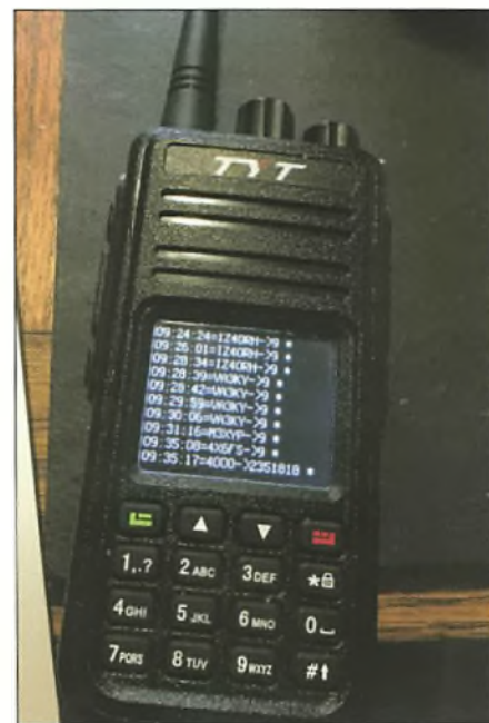
Fig. 1: The MD-380, after the software update, shows a useful 'Last Heard' display.
