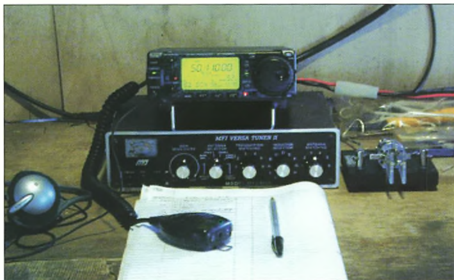
Fig. 1: The simple 3D2AG/P station consisting of IC-706, antenna tuner and a few ancillary items.
