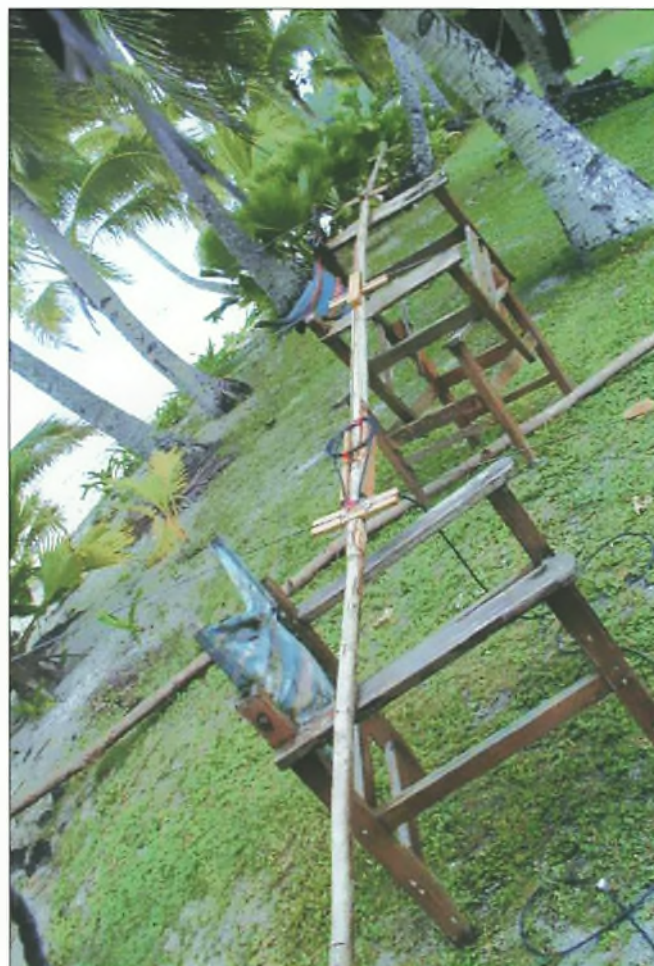
Fig. 3: Starting to build the Yagi on the old lounge chairs.
