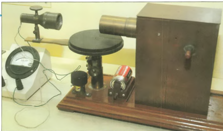
Fig. 7: Jagadish Bose's 60GHz spark-gap transmitter (right) on display at the Bose Institute in Kolkata. The metal tube on the left of the transmitter is a waveguide and Bose's microwave receiver is at the left the picture (the galvanometer and battery are modern replacements). (Photo: Biswarup Ganguly / Wikipedia).
