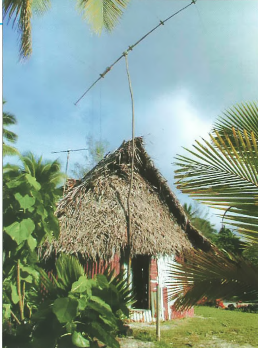
Fig. 5: Not exactly the neatest looking antenna system but the homebrew Yagi and mast (seen here by the 'shack') brought some remarkable contacts. The 10m beam can also be seen behind the shack.
