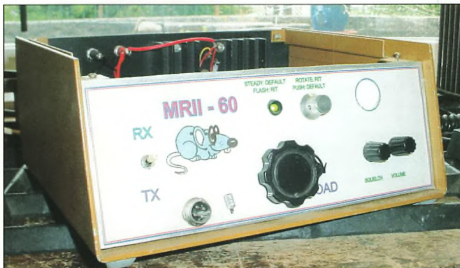
Fig. 5: A single frequency AM transceiver for 60 meters.
