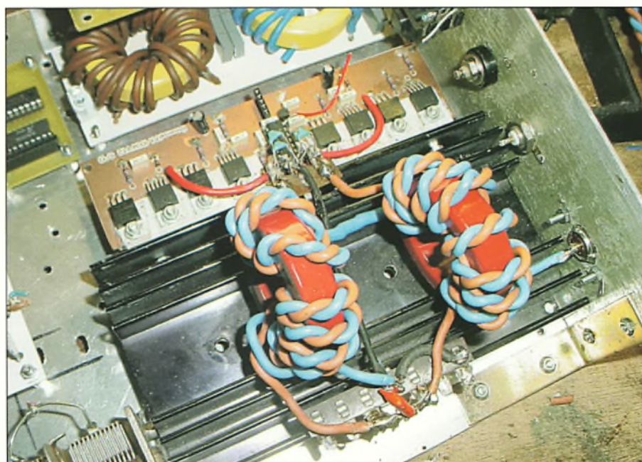
Fig. 4: Higher power version complete with anti-phase circuit and output tuning transformer.
