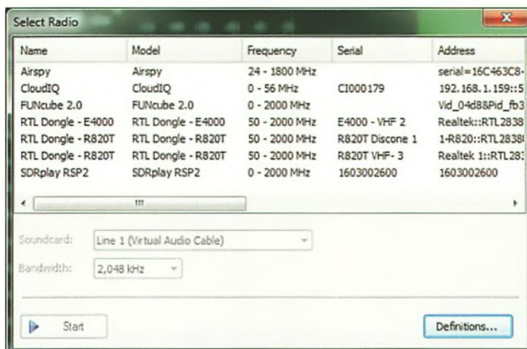
Fig. 6: SDR-Console radio selection panel showing DVB-T dongles with modified serial numbers.
