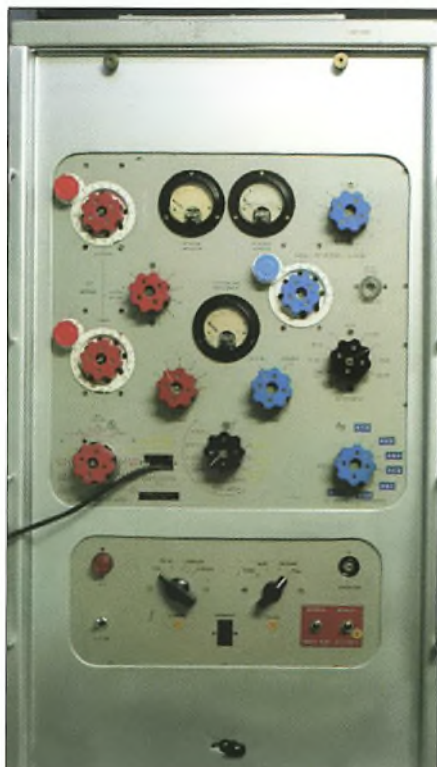
Fig. 6: Oceanspan transmitter. Transmitter in top section. Power supply and modulator in lower section. The dress panel is not original, it was made at Internal Fire. We are still looking for the correct Marconi Hammer finish grey paint.
