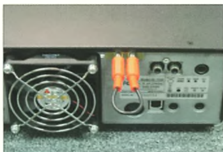
The IC-7300 rear panel with the RX7300 installed and loop fitted to maintain TX/RX through the original SO239 socket.
